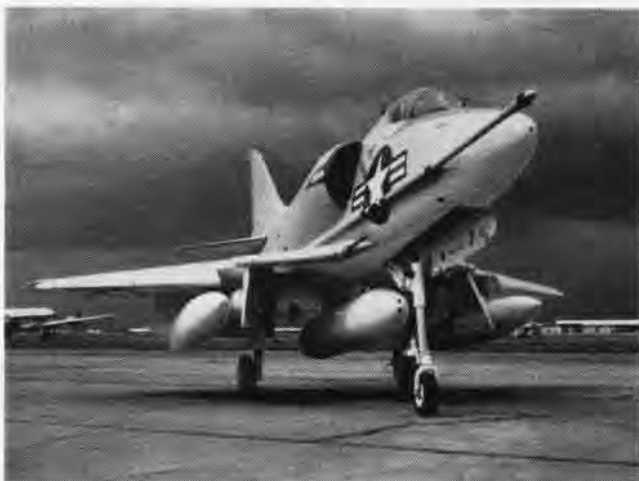
NEW POD-MOUNTED WEAPON , a 20-mm aircraft gun capable of firing 4000 rounds per minute, is displayed on an A4D-2 Skyhawk at the Naval Air Weapons Meet, NAS El Centro. Called the Mark II, the weapon is undergoing evaluation at the Naval Aviation Ordnance Test Station, Chincoteague, Va., and is expected to become opera-
