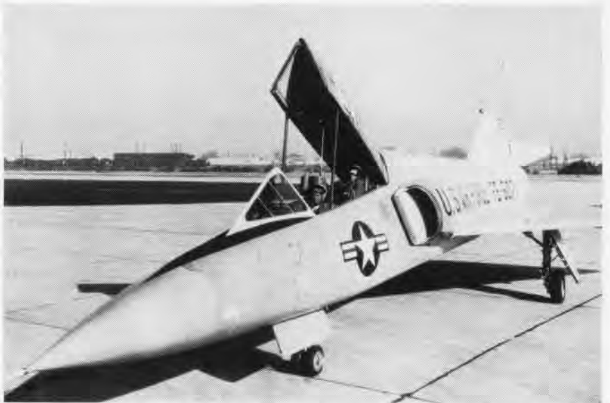
THE ELONGATED NOSE is a distinctive feature of the F-106B Delta Dart. Except for the tandem second seat and the longer cockpit canopy, A and B versions of the F-106 look alike externally. Forward sections of the Delta Dart, a plane described as the fastest, highest flying all-weather jet interceptor in the U.S. Air Force, are fabricated at the Fort Worth plant of Convair Division, General Dynamics, and shipped to San Diego for assembly with rest of aircraft.
