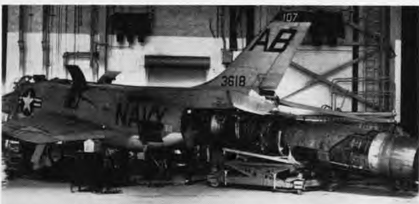
AFTER REWORK IS COMPLETED, THE POWERPLANT OF AN F3H DEMON IS RE-INSTALLED
