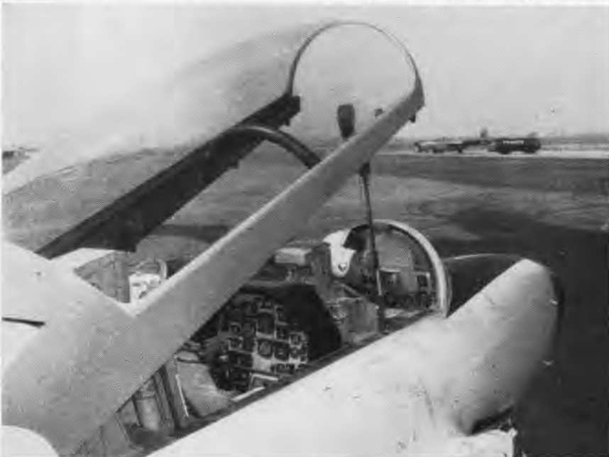
SUCCESSFULLY FLIGHT-TESTED cockpit panel of the future, installed in cockpit of this Navy T2V-1 trainer, has been under development since 1953 as a joint Army-Navy instrumentation program. It has been made available to U. S. Airlines. Panel not only tells pilot what he is doing, but what to do next. Note simplicity of television-type front panel as compared to standard instrument panel in rear cockpit. New concept (story, p. 33) was developed under Douglas contract.
