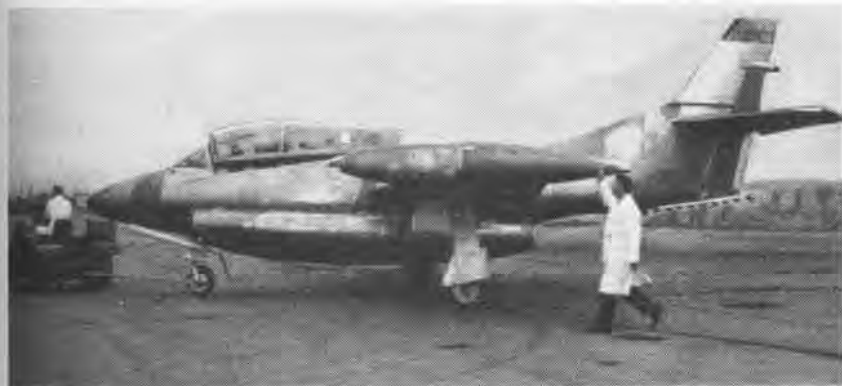
FIRST PRODUCTION model of the North American T2J all-purpose jet trainer rolls out of the plant at Columbus, Ohio. The T2J has a top speed of 429 knots at 25,000 feet and a stall speed of 67 knots. It is a mid-wing cantilever monoplane and is suitable for training in deck operations. The T2J is powered by a Westinghouse J-34 engine which is rated at 2400 pounds thrust.
