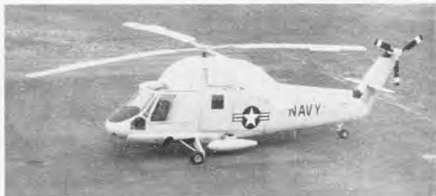
KAMAN HU2K-1 utility helicopter which won BuAer design competition has retractable landing gear, four bladed main rotor equipped with "scruo-flap" control system and will be powered by General Electric gas turbines. The Navy has awarded Kaman a $13-million contract for a prototype quantity of the new helicopters. It will succeed the HOK-1 and HUK-1 craft.
