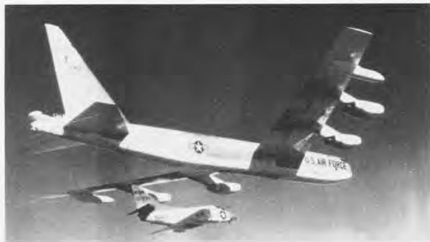
THE LARGEST and the smallest in the United States defense arsenal! The Navy 13,000 lb A4D, Skyhawk makes a striking contrast alongside the Air Force 450,000 lb. B-52 Stratofortress . The A4D is a tactical attack plane and can double in mass with a far-flung nuclear attack when its legs are lengthened by an aircraft carrier, just as are the B-52's with refueling assistance.
