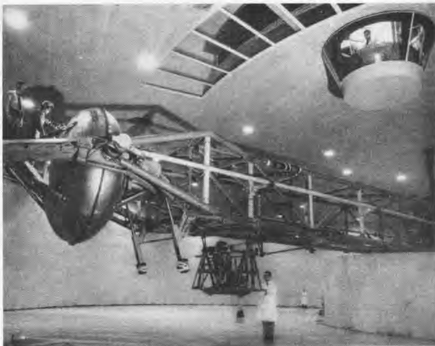
GIANT AMAL human centrifuge, believed to be world's largest, is first to afford pilot control. Dubbed "The Big Wheel," rotor arm and gondola can reach 480 mph in 7 seconds from dead stop.
