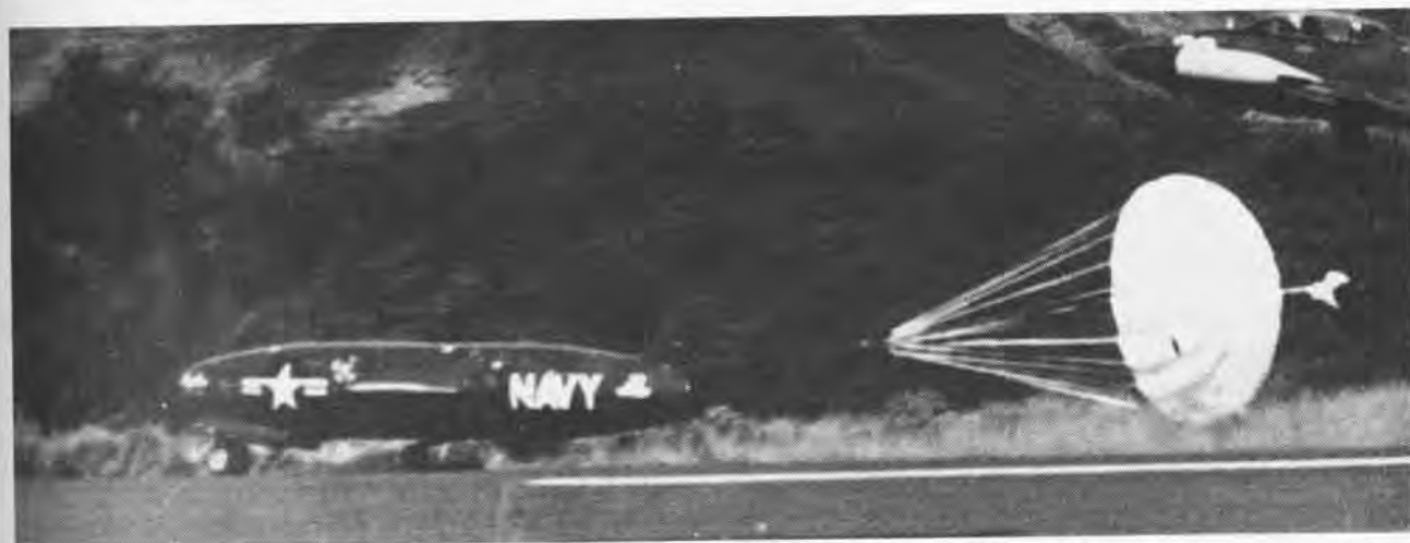
MISSILE TOUCHES DOWN, HITTING THE RUNWAY AT A SPEED IN EXCESS OF 225 MPH. PARACHUTE BRAKE SLOWS MISSILE'S LANDING
