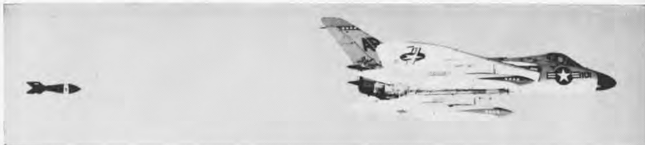
DELMAR HIGH-SPEED target which appears to be zeroing-in on a VF-101 Skyray, was demonstrated recently aboard the USS Forrestal . The bomb-shaped target and special tow rig can be reeled out to lengths up to 20,000 feet and are used for all-weather intercept tactics training.
