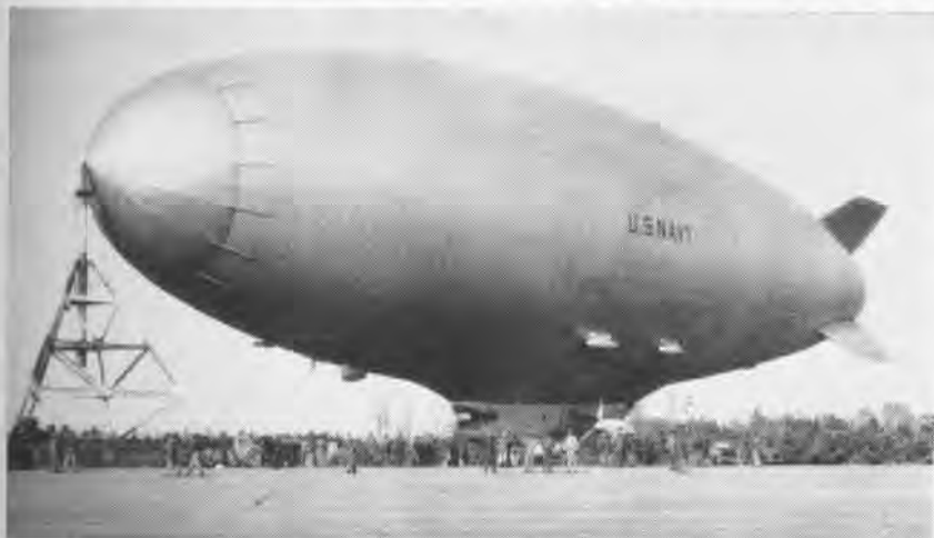
343-FOOT "NAN" SHIP 719 NOSES INTO MOBILE MOORING MAST AT CHERRY POINT
