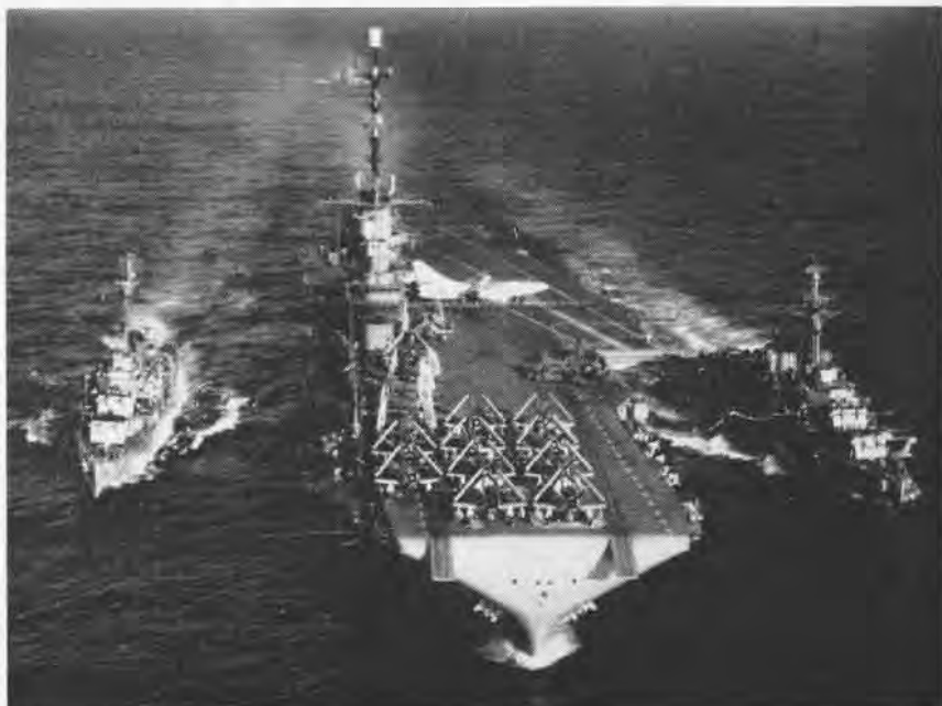
ATTACK AIRCRAFT CARRIER USS Bon Homme Richard (CVA-31) recently inaugurated a port and starboard double-refueling system for destroyers which escort the flattop while operating with the Seventh Fleet in the Far East. This procedure cuts the time the "Bonnie Dick" spends in refueling "tin cans." During the refueling, the carrier replenishes the destroyers with supplies and movies and also delivers mail and messages. The double-refueling system is now SOP.
