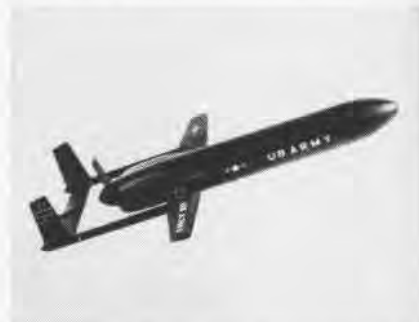
ARMY 'SPYING' machine being produced by Republic is an unmanned drone that has three interchangeable nose units for switching from photography to radar to infra-red. It can be launched "zero length" and is recoverable.
