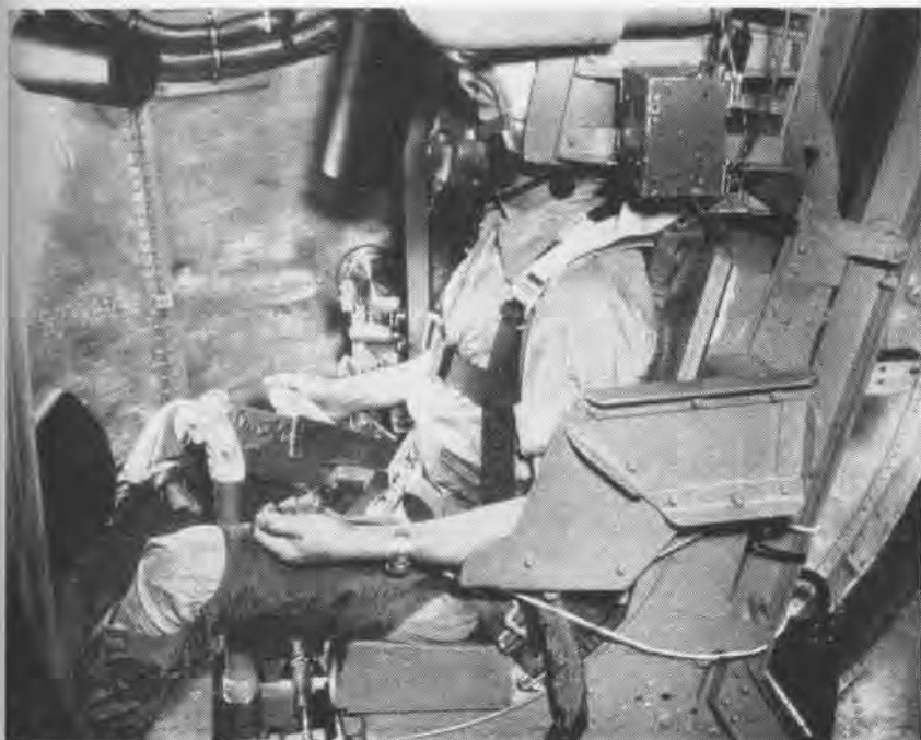
CENTRIFUGE tests provided means of positive study of effect of restraint equipment on head, body, arms and legs of pilot. High "G" forces led to right hand console stick adaptation.
