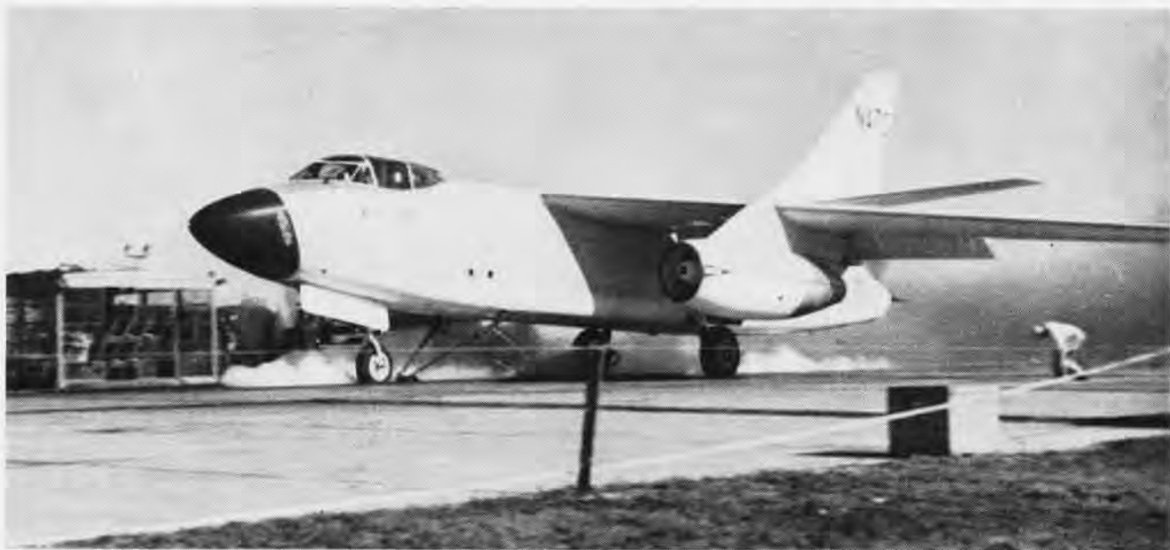
IN LESS THAN three seconds, this A3D-1 Douglas Skywarrior travels 168 mph from a standstill as the steam cat hurls it forward. Once
