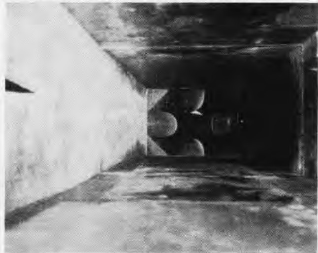
THE SAAB WIND TUNNEL IS POWERED BY FOUR JET ENGINES
