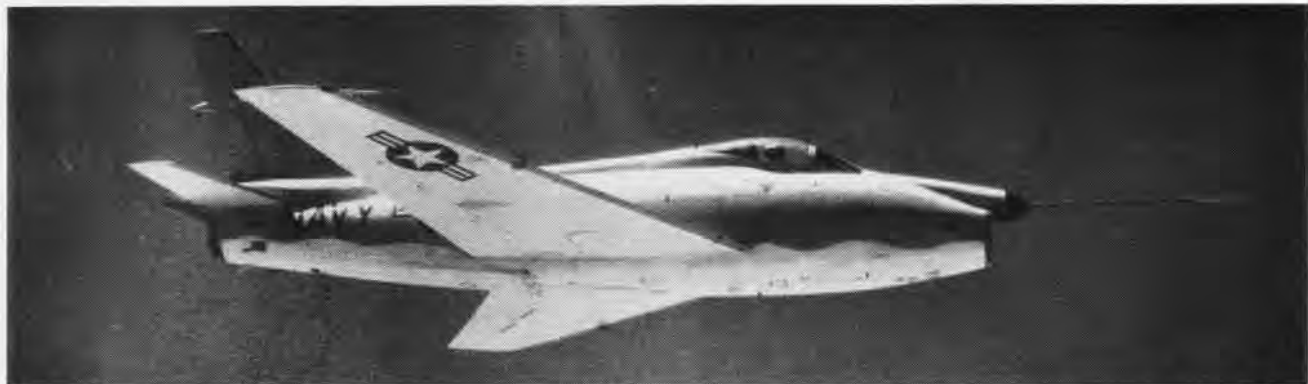
ONE OF NEWEST EXPERIMENTAL MODELS TO UNDERGO TESTING AT NATC IS THE FJ-4F FURY WITH AR-1 ROCKET POWER AUGMENTATION
