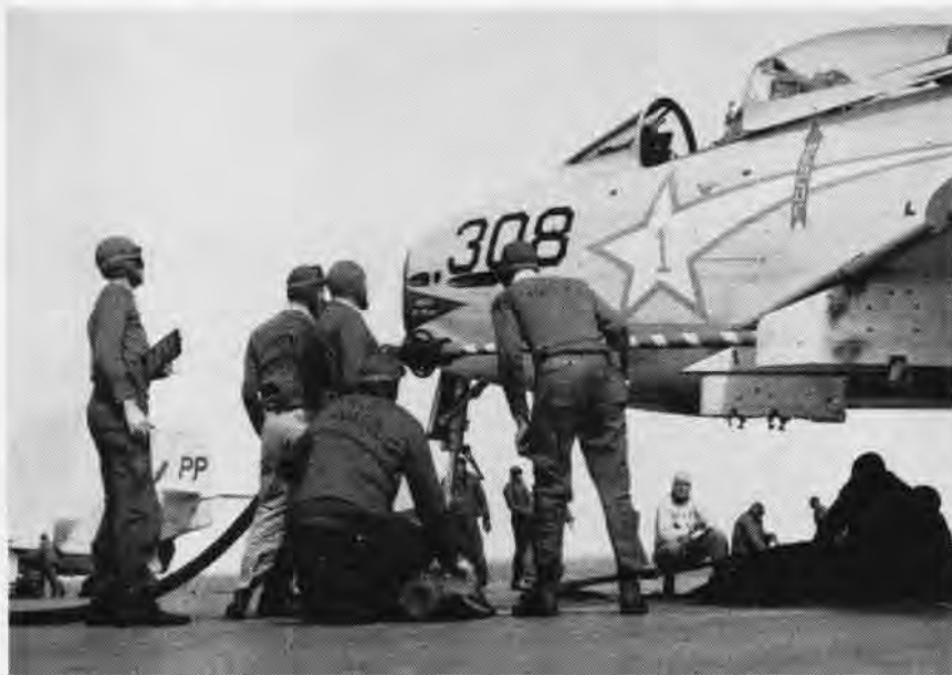
OPERATION QUICK DRINK is conducted by members of VA-151 while deployed aboard USS Bennington . By adapting the principle used in fueling the Regulus missile, FJ-4B Furies were refueled on the catapult. An adapter ground fuel check fitting was attached to the in-flight refueling probe. Time consumed by this method of refueling is approximately three minutes. Previously the Fury was struck below after the second or third arrestment for its refueling.
