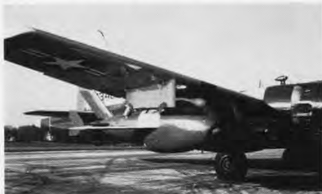
THE FIREBEE TARGET, CAPABLE OF MACH 0.9, MOUNTED ON P2V
