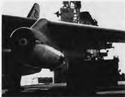
A NAVY A3D tests the Midway's modern jet-blast deflectors during a rest period in the busy ship's training schedule at Alameda, California. Deflector consisting of three plates may be used singly or jointly.
