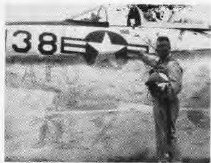
GUNNERY BANNER held by Cdr. F. S. Standing, OinC ATU-201 Corpus Christi, shows 156 hits out of 200 rounds. The 78% score, a record for ATU-201, was fired in an F9F-5 using a fixed Aero-3A gyro without radar.
