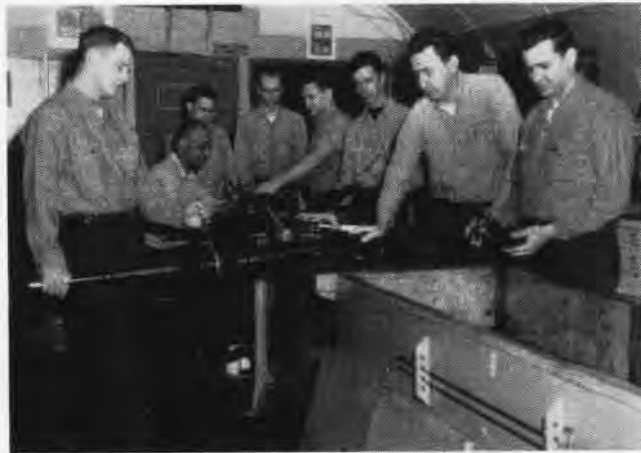
20 MM CANNON is broken down during periodic inspection by VA-662 Aviation Ordnancemen. R. Greathouse, AO1, far right, is in charge.
