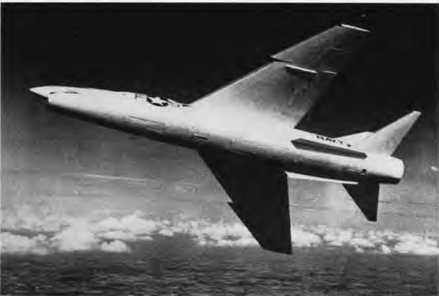
THE F8U-2, MANUFACTURED by Chance Vought Aircraft, has made its first flight. A faster and higher flying version of the F8U-1 Crusader , world's fastest Navy jet fighter, the F8U-2 can achieve speeds in excess of 1000 miles per hour and yet land on some 200 feet of carrier deck. Powered by a Pratt & Whitney J-57-P16 engine, the F8U-2 resembles the F8U-1 except for the addition of two fixed lower aspect ratio ventral fins mounted under the tail section and two afterburner air scoops on the tail cone between the horizontal tail and vertical stabilizer. The first flight of the production model of the F8U-2 is scheduled to take place in September.
