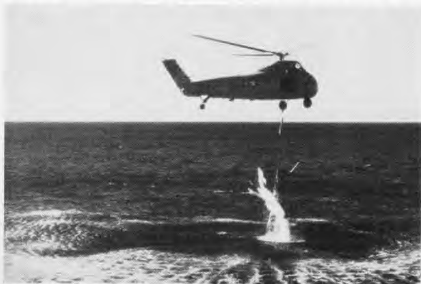
HELICOPTER FROM HU-1 RETRIEVES FIREBEE AND HEADS HOMEWARD WITH ITS 'CATCH'
