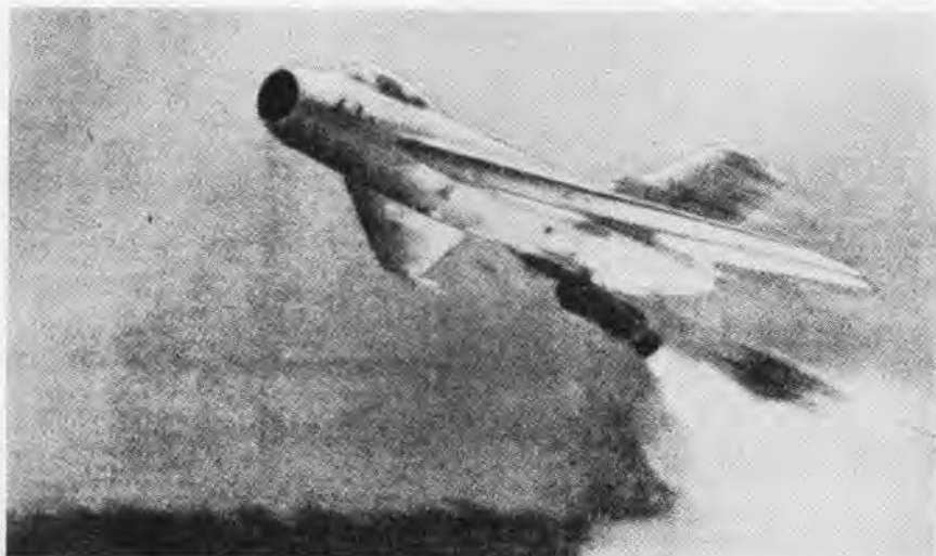
IN A SOVIET MAGAZINE, the "Sovietskaya Aviatsia," published in December 1957, the editors published a picture of a MiG-19 immediately after launching with a rocket booster. The booster, which is jettisoned after burn-out, is mounted below the rear fuselage. The launching system appears to be similar to those developed in this country for the Republic F-84 Thunderjet aircraft.
