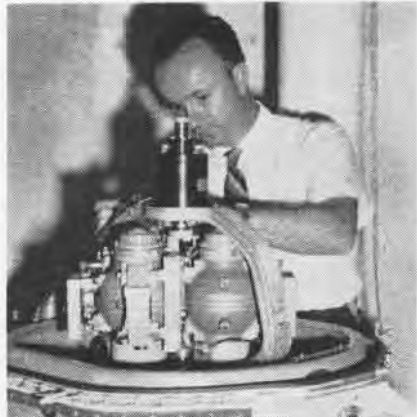
ENGINEER from North American Aviation goes over inertial navigation system's stable element.
