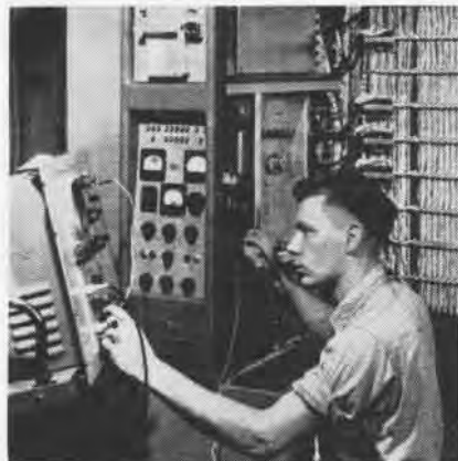
FARRAND star tracker's camera assembly is adjusted by a ship's Electronics Technician.
