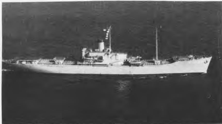
COMPASS ISLAND cuts the brine. Mission of experimental ship is to assist in the development and evaluation of a navigational system which is completely independent of shore-based aids.
