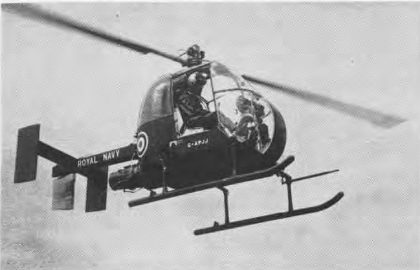
FAIREY ULTRA LIGHT CAN TAKE OFF AND LAND ON SHIPS DURING VERY ROUGH WEATHER
