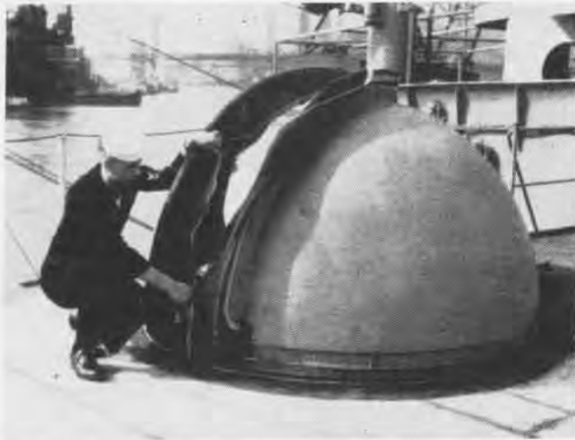
CREWMAN UNZIPS the canvas covering to inspect a star tracker located topside of experimental ship Compass Island while in port.
