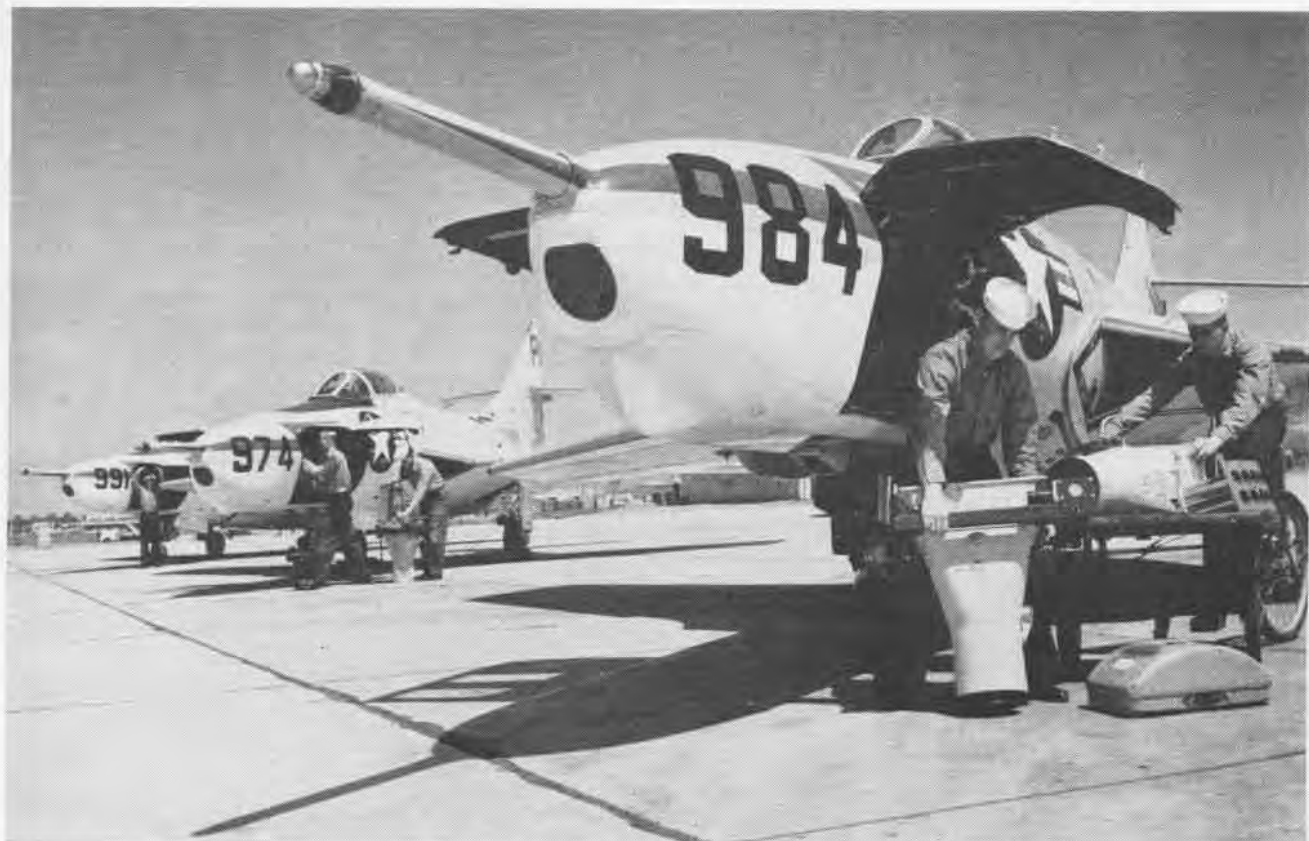
MODERN F9F-8P COUGARS ARE LOADED WITH AERIAL CAMERAS IN PREPARATION FOR AN IMPORTANT RECONNAISSANCE MISSION
