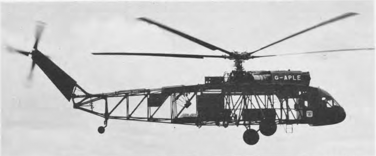
WESTMINSTER CRANE/TRANSPORT VERSION WHICH CAN LIFT LOADS OF SIX TONS OR MORE, HAS COMMERCIAL AND MILITARY CAPABILITIES
