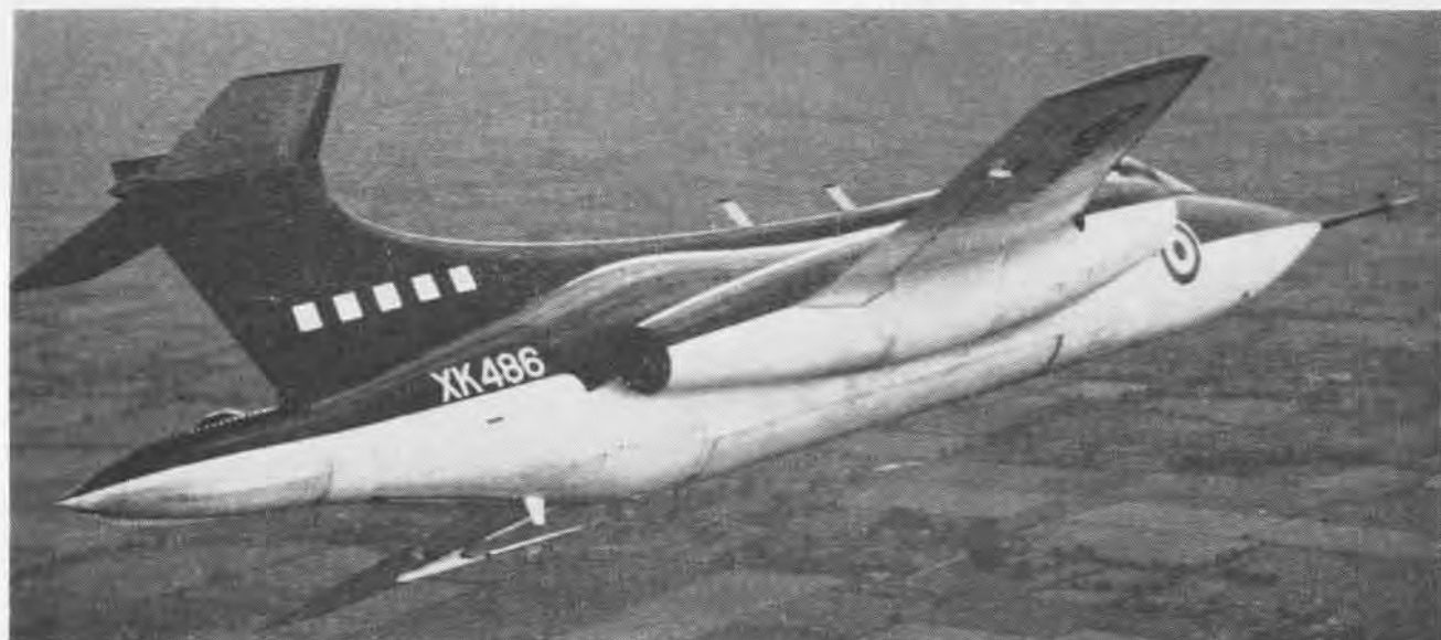
'AREA RULE' AND BOUNDARY LAYER CONTROL GIVE N.A.39 HIGH SPEED AT LOW LEVEL, FLEXIBLE SPEED RANGE FOR CARRIER USE
