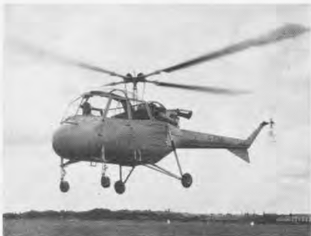
P.531 IS POWERED BY BLACKBURN TURMO GAS TURBINE ENGINE
