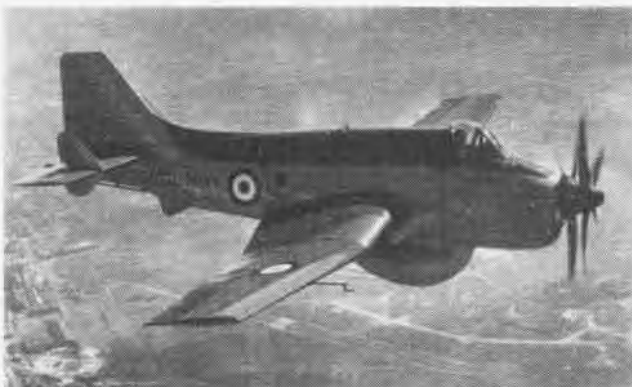
GANNET ASW PLANE FEATURES RADAR POD UNDER ITS FUSELAGE
