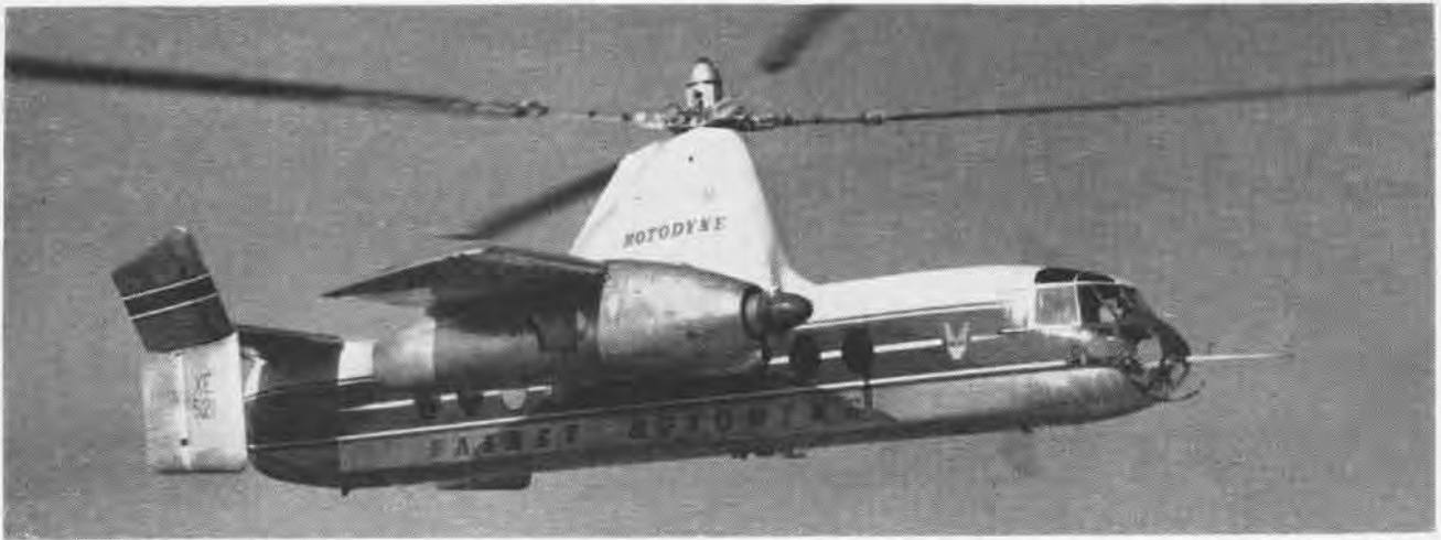
ROTODYNE DIMENSIONS ARE IMPRESSIVE: CRUISE SPEED, 185 MPH; 48 PASSENGERS; ALL-UP WEIGHT, 18 TONS; ROTOR DIAMETER 90 FEET
