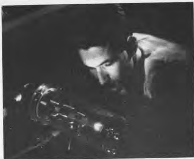
AN ION ACCELERATOR IS USED TO STUDY EROSION BY PARTICLES
