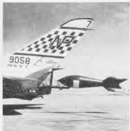
NEW DELMAR target system, attached to F4D Skyray at Moffett Field, is introduced on West Coast by VF-213. System is used in lead collision interceptions in which intercepting fighter approaches the target at head-on angle.
