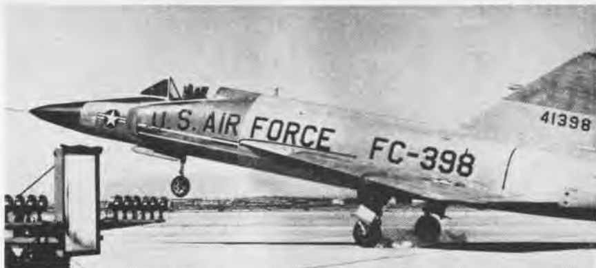
NAVY MIRROR LANDING SYSTEM was adapted by Convair to facilitate recent tests of its F-102A Delta Dagger. System's glide path feature permitted completion of gear loading tests in 67 landings instead of 200 landings expected if the mirror-controlled flight testing had not been used. Test pilot C. E. Myers, Jr., former Navy pilot, in checking 60 different landing configurations with canopy removed, established vertical sink rates varying from three to ten feet per second. Tests also involved single-wheel touchdowns. In all, test series wore out 20 sets of tires.
