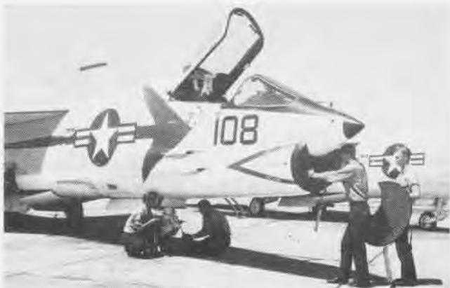
LINE CREWS TAKE CARE OF TIE-DOWN AND INTAKE DUCT COVERS
