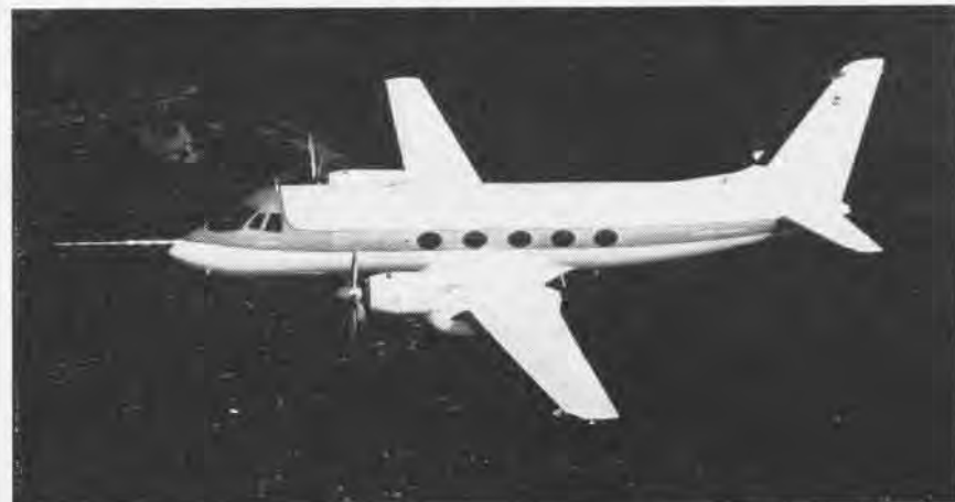
NEW BIRD in the sky is Grumman's executive transport, the Gulfstream, shown here on its initial flight. Powered by two Rolls Royce Dart engines, the prop-jet, pressurized aircraft has a maximum cruise of 370 mph at 25,000 feet and a range of 2200 miles. Designed to operate from runways as short as 4000 feet, the Gulfstream can carry from 10 to 19 passengers. Other commercial aircraft produced by Grumman in the past were the Gray Goose, Wildgeon and the Mallard.
