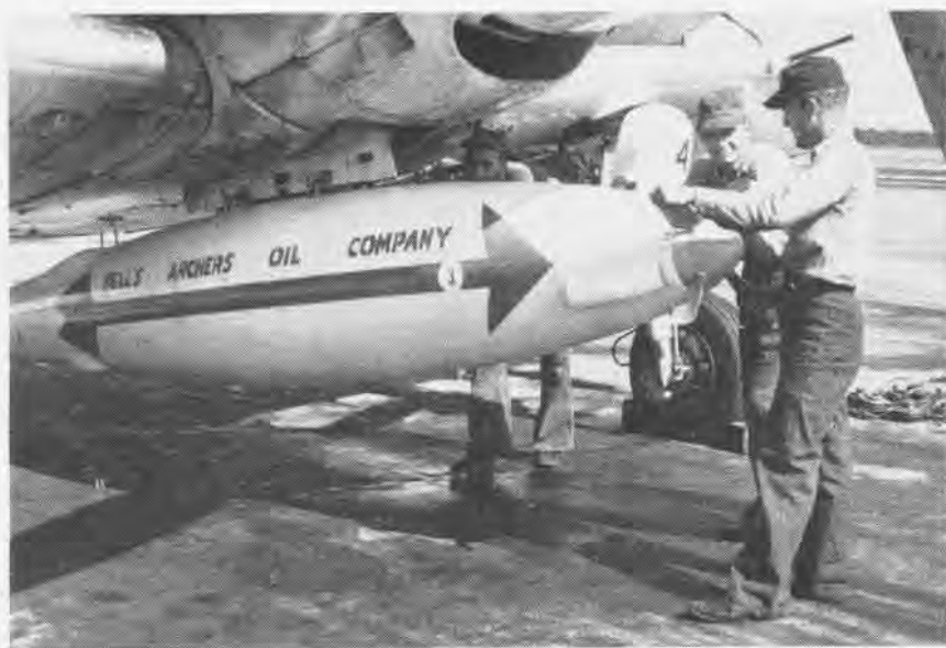
LINE CREWMEN INSTALL IN-FLIGHT REFUELING TANK ON BELLY OF AD-6 SKYRAIDER
