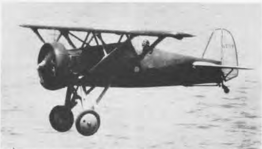
ALL-METAL, STRUT-BRACED, PARASOL-WING BOEING XF5B-1 POSED WEIGHT PROBLEM
