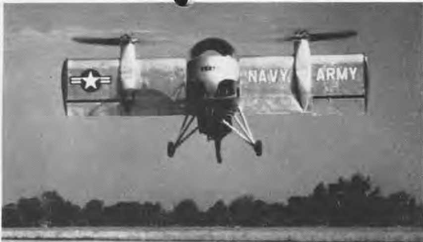
WITH ITS WING IN THE VERTICAL POSITION, VERTOL VTOL HOVERS IN HELICOPTER STYLE
