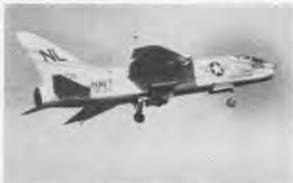
F8U CRUSADER IN LANDING CONFIGURATION
