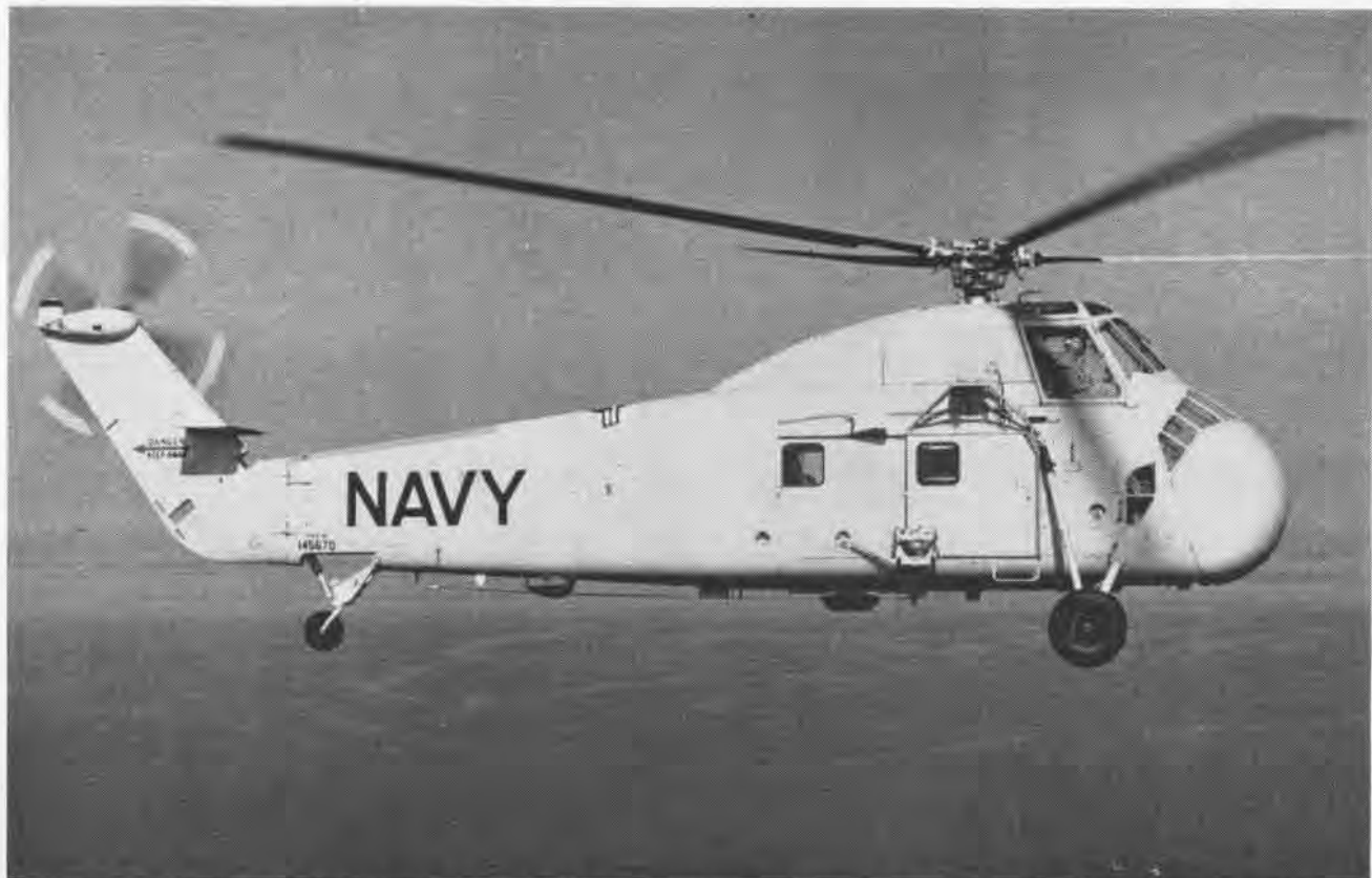
SIKORSKY HSS-1N HELICOPTER WILL GIVE THE FLEET AN UNPRECEDENTED POTENTIAL BY VIRTUE OF ITS NIGHT HOVER CAPABILITY
