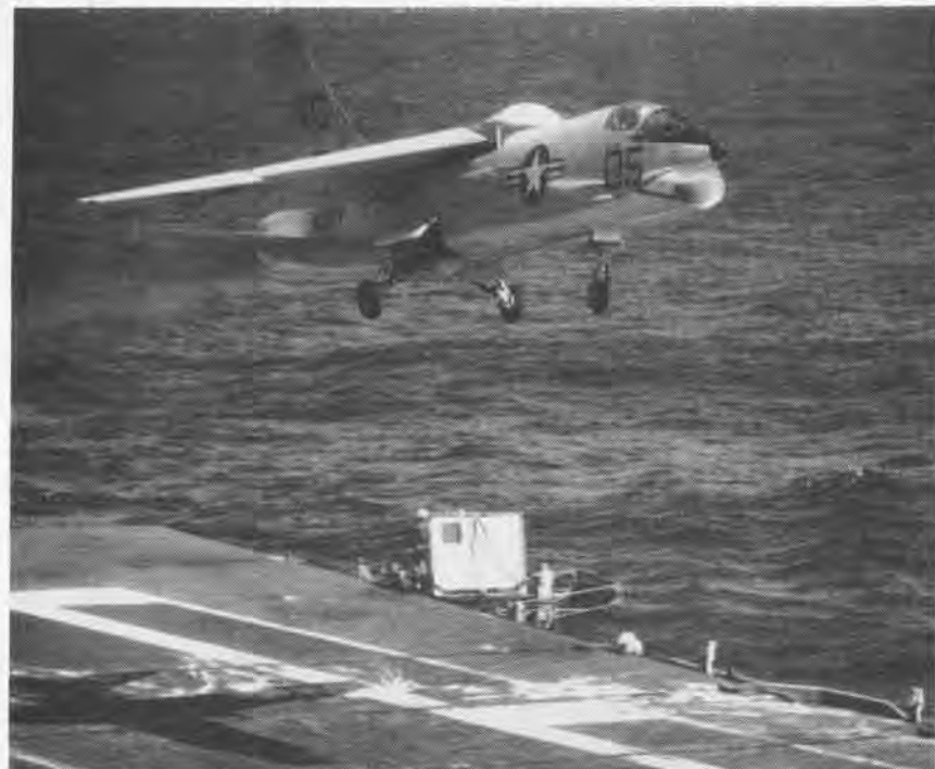
CRUSADER'S HIGH-WING DESIGN WAS NECESSARY TO GET VARIABLE INCIDENCE WING
