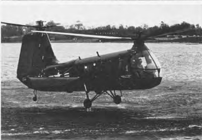
'SEACOPTER' GOES through its paces at NATC Patuxent River. The Navy's first bull type amphibious helicopter completes a low speed water landing, top picture, during hydromatic evaluation tests. Second photo shows the seacopter rising from the seaplane basin after the demonstration. A standard Vertol HUP-2 was modified by the EDO Corporation to include a reinforced hull bottom, all-metal outrigger floats, and a re-ducted engine cooling air system.
