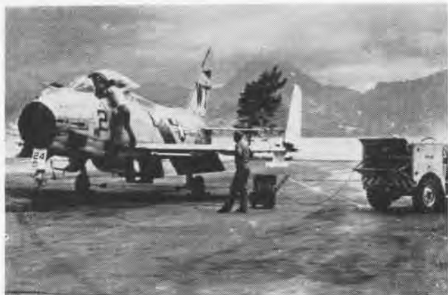
VMF-232 MECHS GIVE J65 JET POWERPLANT PERFORMANCE CHECK
