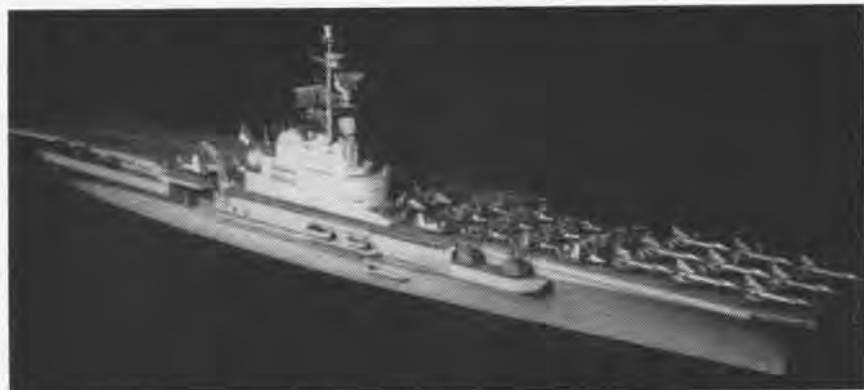
CLEMENCEAU , largest warship to be built in France since 1939, is nearing completion at the Brest Navy Yard. Trials are scheduled to start soon. Built by Chantiers de l'Atlantique, the 846-foot carrier compares to British Hermes/Centaur class in size but is faster (32 knots max.). Powerplant is rated at 120,000 b.h.p.; cruising radius is 7,500 miles at 18 knots. Flight deck and bridge structure are armored. (Photograph of the model by France Actuelle.)
