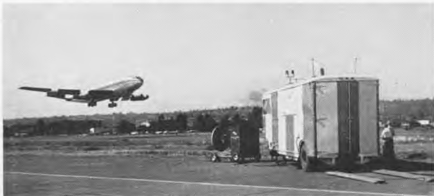
GIANT BOEING 707 prototype, four-engine jet transport, is brought to a perfect landing at Boeing Field, Seattle, Washington, by Bell Aircraft automatic all-weather landing system in right foreground. In a series of flight tests, the system's radar picked up the jet transport two to four miles from end of the runway and controlled it through automatic pilot all the way to touchdown.
