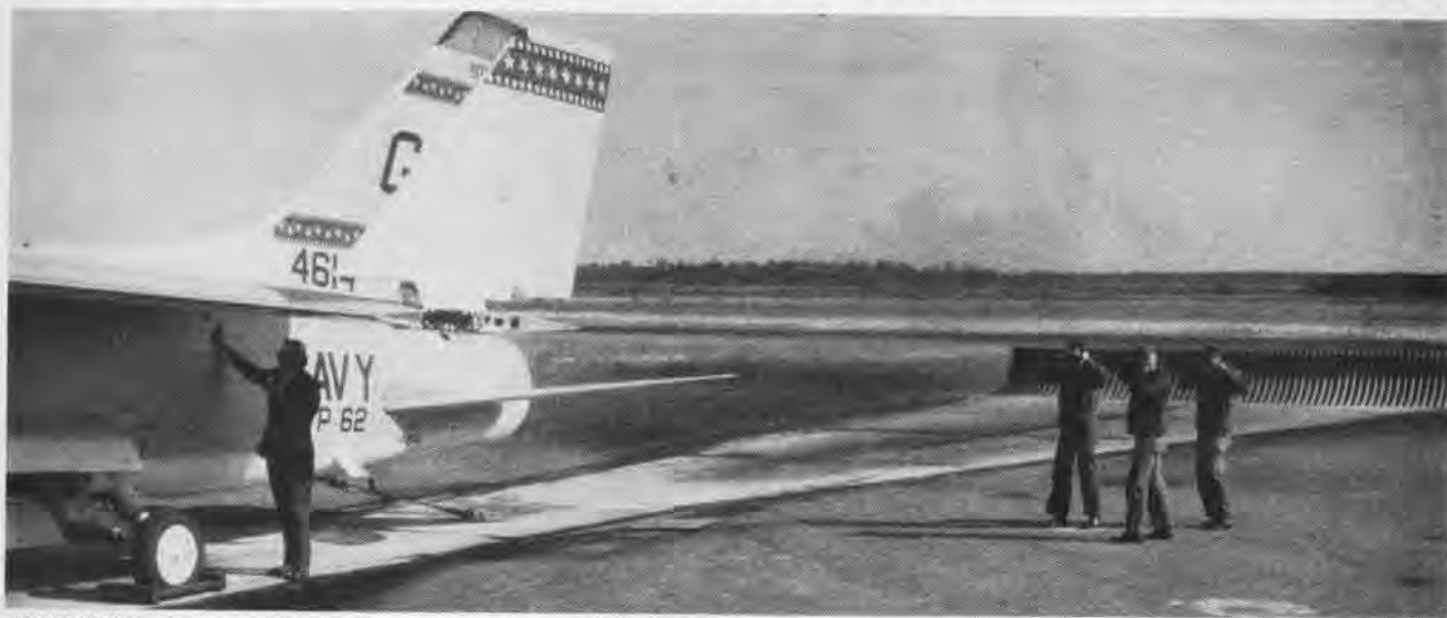
HIGH DECIBEL output of FSU-1P during static turnup at NAS Jax is attenuated in various ways. Man under wing wears ear muffs while
