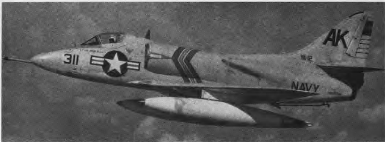
CLOSE-UP OF A 'SERGEANT-STRIPED' A4D-2 OF ATTACK SQUADRON 12, WITH THE 300-GALLON WING TANKS AND REFUELING GEAR
