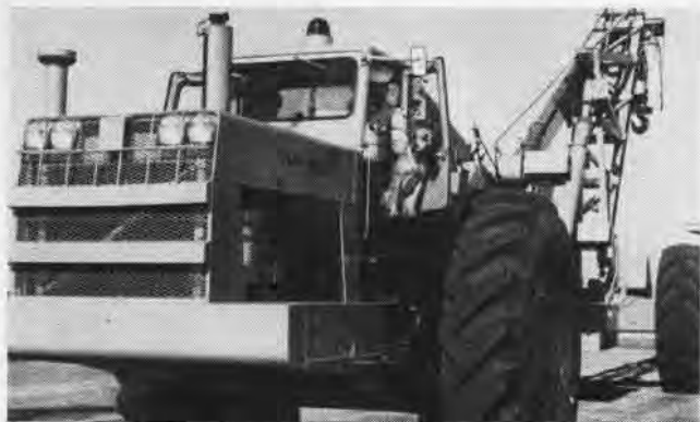
'CHERRY PICKER,' A 50-TON CRANE, IS USED TO LIFT PLANES
