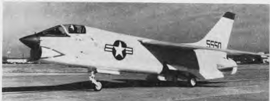
FIRST F8U-2 delivered to Navy arrives at Naval Air Test Center, Patuxent River where it will be given further testing. Crusader was flown by Lt. J. J. Chambers. Two long ventral fins below rear fuselage and twin air scoops atop tailpipe are main external recognition features. Still another version of the Chance Vought supersonic, carrier-based fighter, the F8U-2N has been ordered by the Navy for limited all-weather and night operations. (See story, page 3.)
