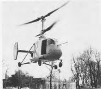
GYRODYNE IS MARKED BY COAXIAL DESIGN
