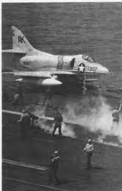
ENVELOPED in steam, the catapult officer gives final launch signals to the A4D pilot.
