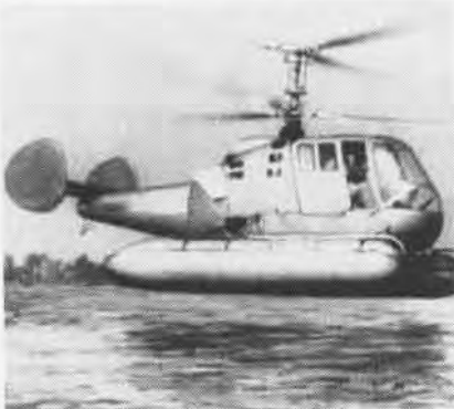
USSR'S COAXIAL 3-BLADED ROTOR COPTER
