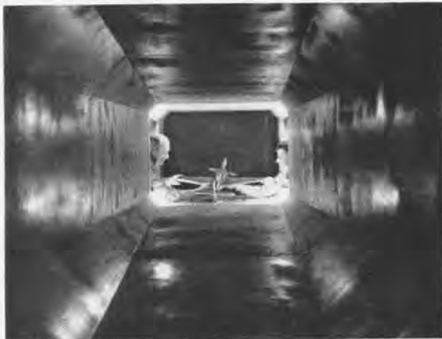
AIRCRAFT MODEL IS READIED FOR SUBSONIC WIND TUNNEL TEST
