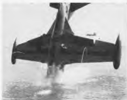
A SPECIALLY INSTRUMENTED F9F 'CRASHES'
