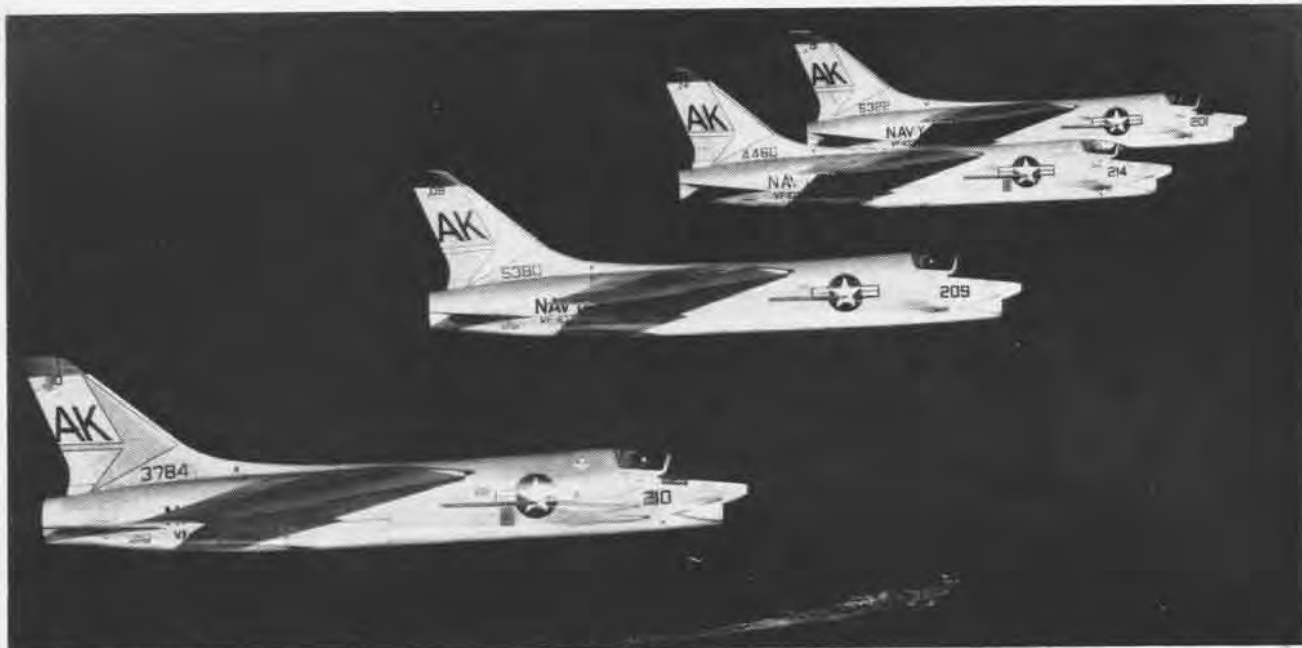
THE ATTACK CARRIER striking force normally contains two large carriers and about 200 aircraft. These four F8U Corsairs are shown as they make their approach to the Forrestal prior to landing. The Crusader lands on Forrestal's 720-foot landing runway at about 140 mph.
