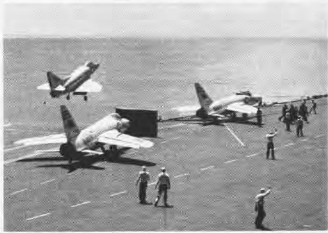
FOUR CATAPULTS make Forrester launchings faster than on small carriers. Here an A4D is catted as two F4F aircraft are readied for launch.
