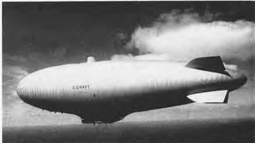
WORLD'S LARGEST non-rigid airship, the Goodyear ZPG-3W, flies from Akron to Lakehurst for delivery to the Navy. One of four blimps built at a total cost of $48-million, the first ZPG-3W will enter service with ZW-1 on the Atlantic Barrier in October. The other three will join the squadron by late spring next year. The 3W's have 1½-million-cubic-foot helium envelope, use two 12-man crews, measure 403 feet overall, and cruise at some 70 knots plus.
