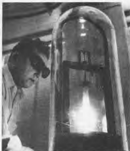
NIOBIUM BAR is purified in a vacuum having four billionths the pressure of atmosphere.
