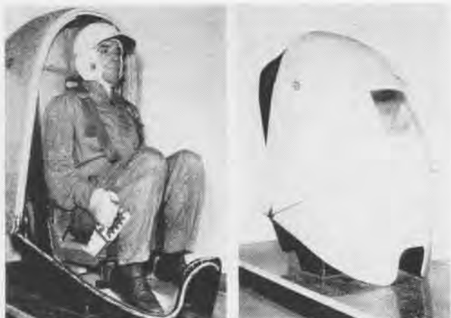
CAPSULE DURING NORMAL FLIGHT, LEFT, AND AFTER EJECTION
