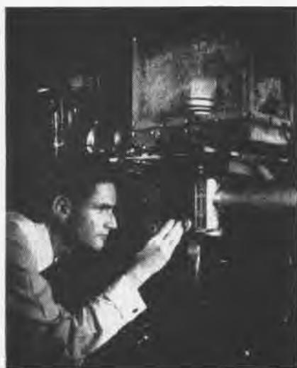
NASA PARTICLE accelerator produces same effect as ions striking materials in re-entry.
