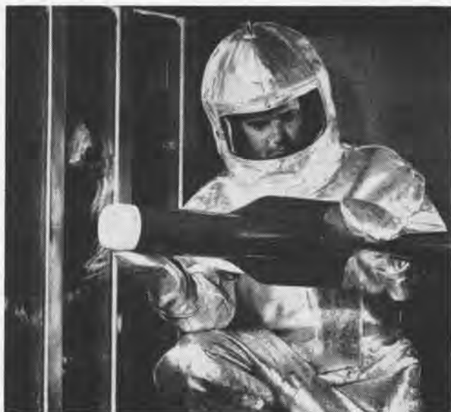
PLASTIC MODEL of rocket motor is tested in NASA wind tunnel at 400°F. In aluminized suit mechanic can withstand the high heat.
