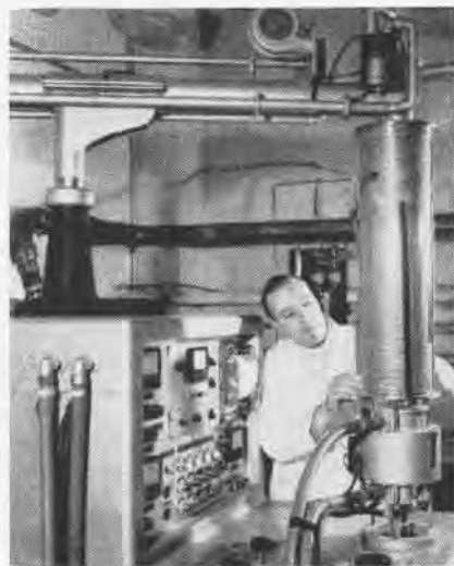
MAGNETIC REFRIGERATOR cools samples to near absolute zero (-273.1 C.) to test properties.
