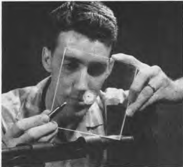
PROJECTILE FIRED at high velocity is used to measure the resistance of Plexiglas to impacts that might be met in space flight.
