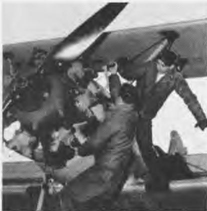
INERTIA STARTER IS WOUND UP BY CRANK
