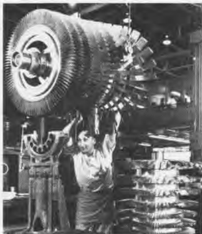
TITANIUM ALLOY compressor for Pratt & Whitney engine is 443 pounds lighter than steel.
