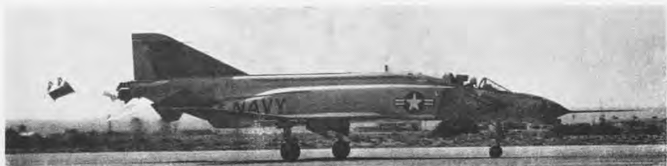
SPIN RECOVERY tests on the McDonnell F4H-1 are conducted at Edwards Air Force Base, Calif. Before test flight, the emergency spin recovery chute is tested by deploying it during high speed taxi runs. The recovery chute is installed in modified aft fuselage.
