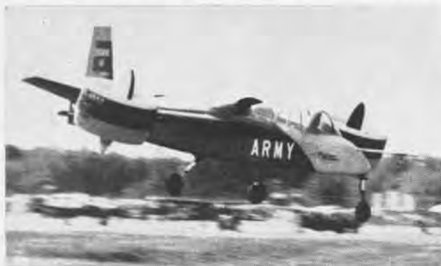
BEFORE TOUCHDOWN, DUCTS ARE SHIFTED TO NEARLY 90 DEGREES
