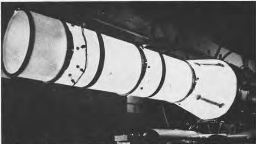
COATED MOLYBDENUM turbine blades and other innovations make it possible to operate G.E.'s Hot Rod research engine at ultra-high temperatures to test materials for engines of tomorrow.
