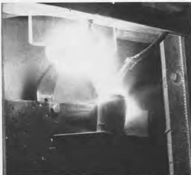
MAN-MADE LIGHTNING triggers underwater explosion. Resulting shock wave is converted into the force needed to form space age metals.
