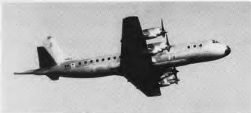
PROTOTYPE P3V-1 long-range Navy ASW plane makes first flight. The Navy awarded Lockheed a $10,000,000 pre-production contract for work on the four-engine sub-hunter in October. This test bud will make it possible to do evaluation work and carry on in-flight systems development.
