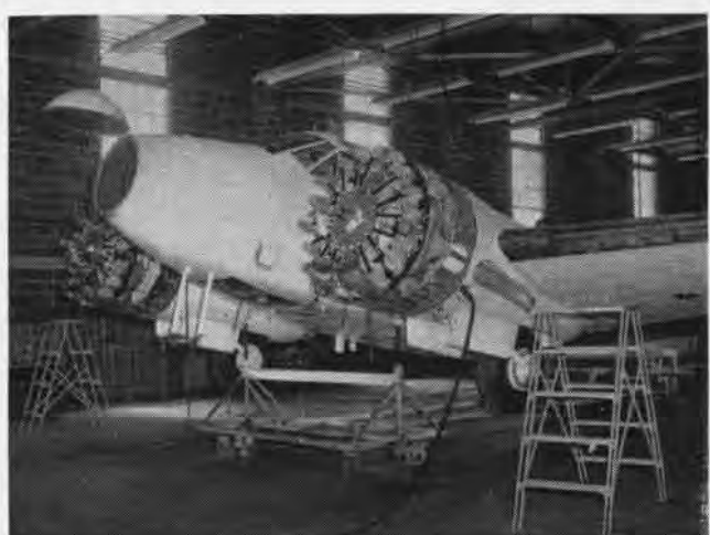
LANDING GEAR IS DROP-CHECKED BEFORE THE PLANE IS RELEASED
