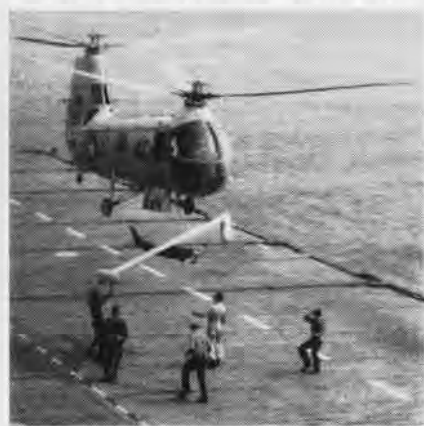
TARGET DRONE recovered from sea by helicopter of HU-2 is returned to deck of USS Leyte. Crewman was lowered into water from copter to cut away parachute and attach hoist cable directly to the drone's parachute harness.
