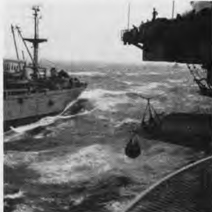
STORES in cargo nets are transferred by high-line from provision ship to the Forrestal .
