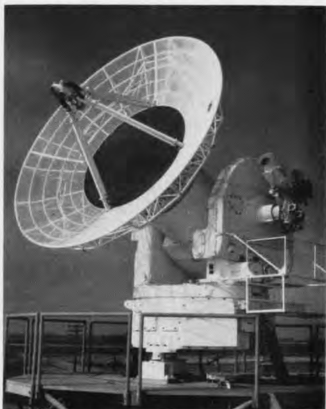
TRACKING RADAR WITH 300-MILE RANGE IS ACCURATE TO 1/10 MIL
