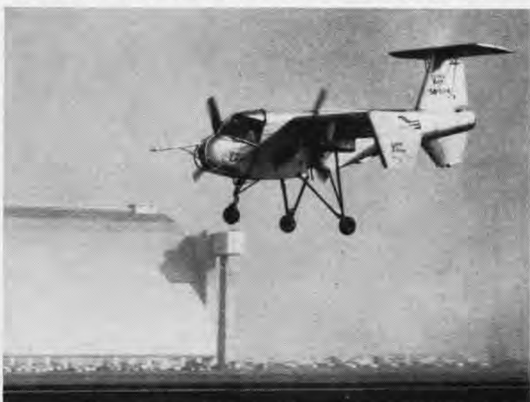
stration, shows flaps in fully deflected position. Prop slipstream is bent downward by flaps to provide lifting force which allows Vertiplane to take off vertically or hover in flight. The aircraft, which flew at altitudes in excess of 5500 feet and speeds up to 100 knots, is powered by a single Lycoming T-53 gas turbine engine.
