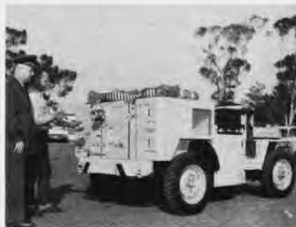
CAPT. LAWLER checks NC-3-AIR, an all-purpose starting and electrical service vehicle.
