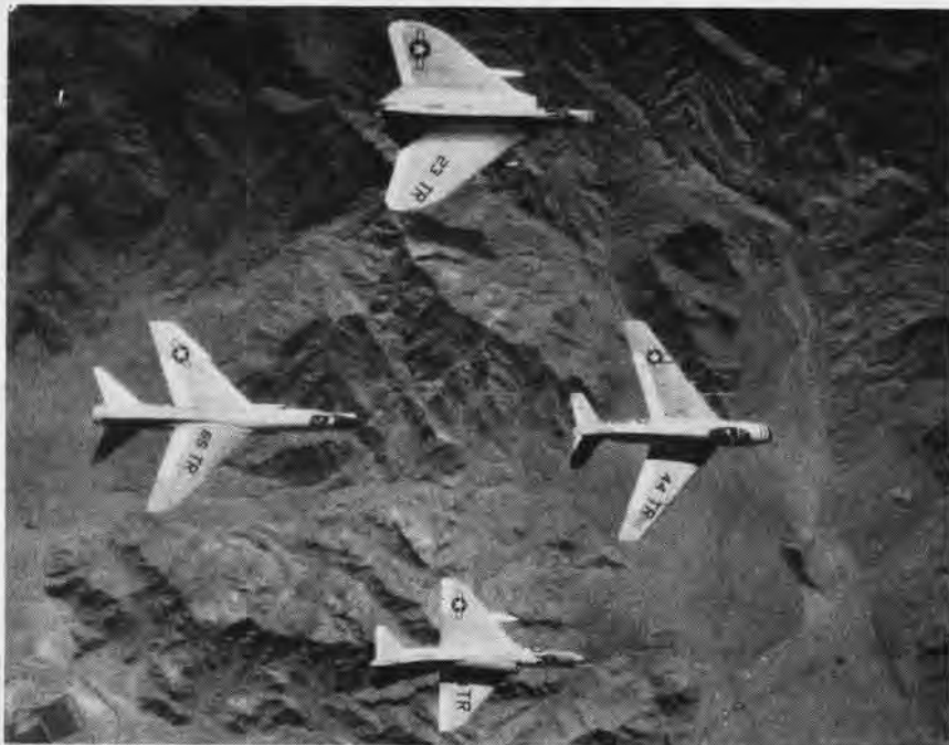
FAGU PARADE: FJ-4B IN LEAD, F4D-1 ON LEFT, A4D-2 ON RIGHT, AND F8U-1 IN SLOT
