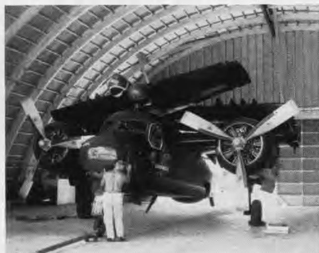
COMBINATION of unique "noise free" aluminum hangar and negligible iron content in Florida soil afforded optimum MAD test conditions.
