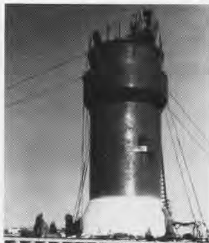
MISSILE TEST equipment comes king-sized these days. Gigantic underwater-bousing for Polaris test launcher was later towed into position off California for use in "Operation Pop-up." The firings were simulated.
