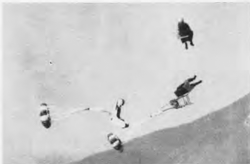
DUMMY IS FIRED IN TEST. NOTE SEPARATION OF MAN AND SEAT, AIDED BY DROGUE
