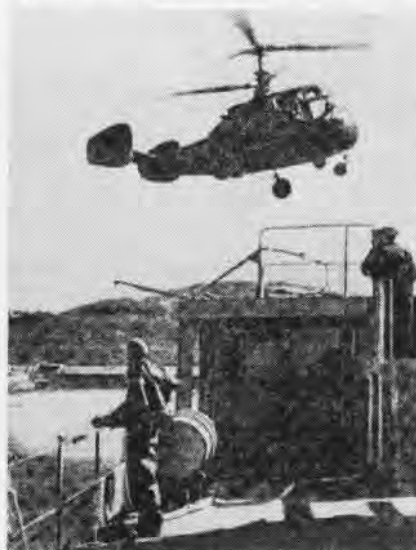
THE RUSSIAN publication, "Soviet Fleet," carried this picture of a Hen helicopter preparing to land on a destroyer. The article stated that these copters are for search and destruction of submarines by bombing.
