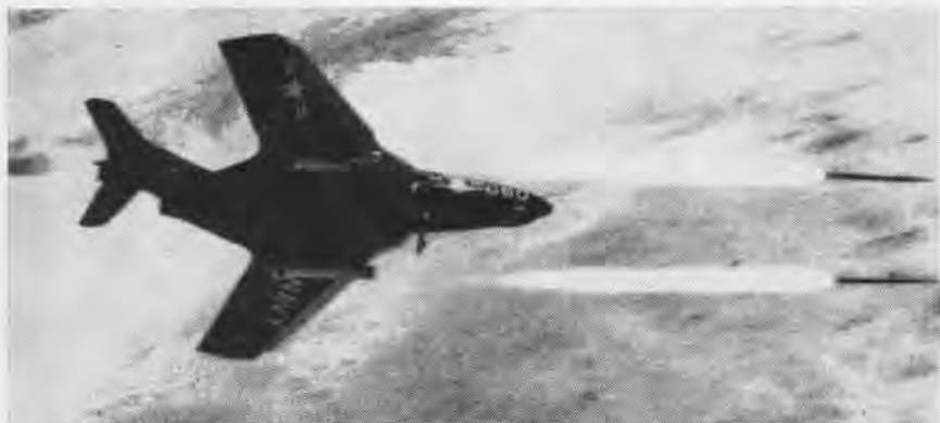
AN F9F-8 COUGAR FIRES A PAIR OF ZUNI ROCKETS DURING NOTS CHINA LAKE TESTS
