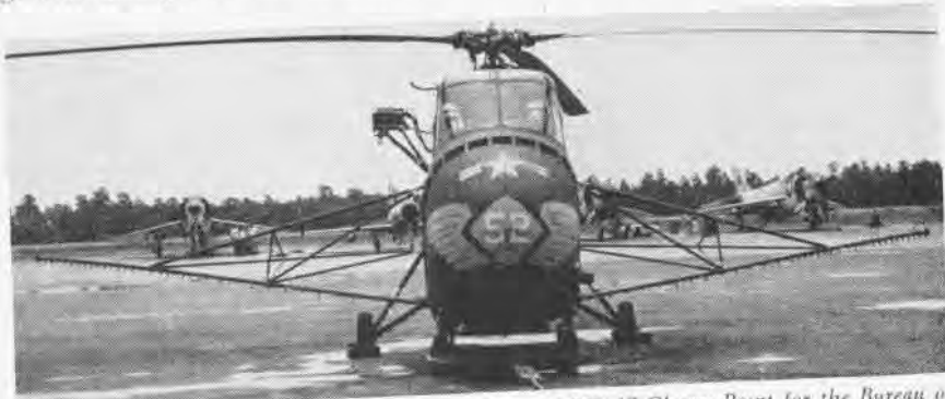
THE GIANT BUG KILLER , designed by O'R workmen at MCAS Cherry Point for the Bureau of Aeronautics is dubbed the "HIDAL" (Helicopter Insecticide Dispenser Apparatus Liquid). The HRS is armed with two 55-gallon tanks of insecticide and two spraying booms. The copter, capable of wiping out the mosquitoes in a large area, will be evaluated at Patuxent River. Once approved, it will be used in swamp areas near Navy and Marine installations.
