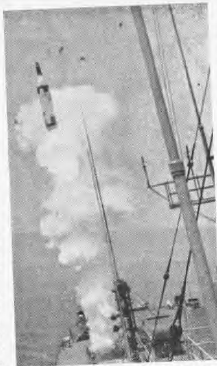
POLARIS test vehicle was fired for first time from a surface ship, USS Observation Island , August 27. Objects around missile are launching shoes used to separate vehicle from tube. All test objectives were met.
