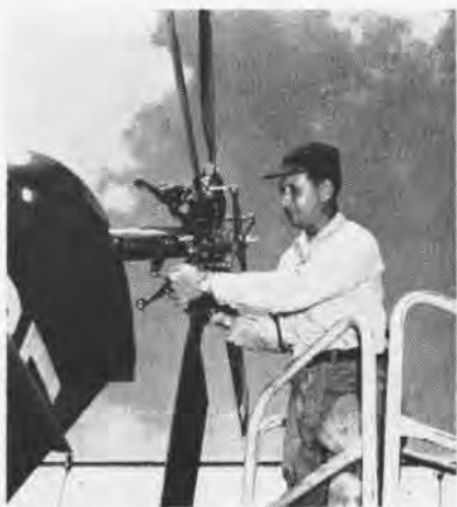
TAIL ROTOR adjustment is made by Alianell, AD1, during HS-741 training cruise at Jax.
