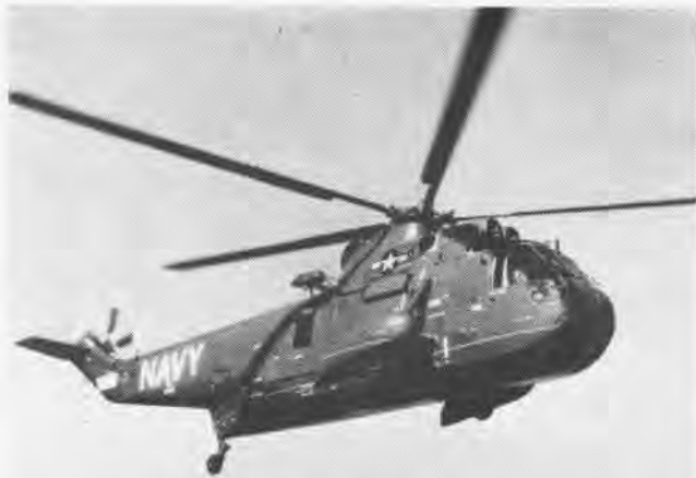
NEW SIKORSKY HSS-2 HAS TURBINE ENGINES, FLYING BOAT HULL
