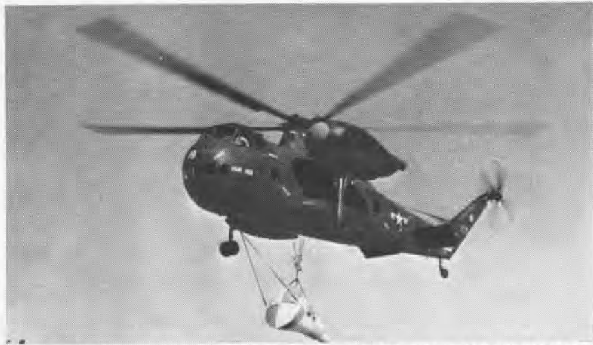
MARINE HR25-1 LIFTS MERCURY CAPSULE FROM ITS PAD AND HEADS OUT TO DROP AREA
