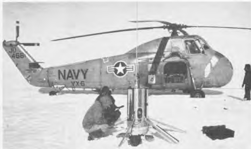
DEEP FREEZE MEN check electronic "Grasshopper" used in Antarctica to gather and transmit weather reports from outlying scientific stations. Navy-designed and still in the developmental stage, units are battery-operated, and should last four weeks, broadcasting signals four times daily.
