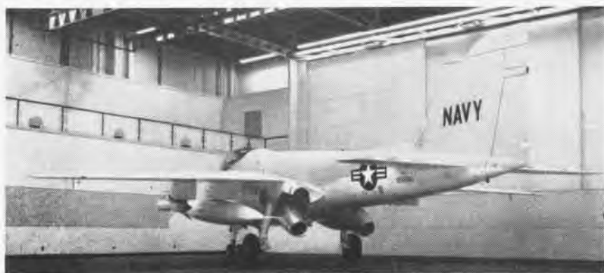
A2F HAS TILTING PIPES FOR SHORT FIELD TAKEOFFS, CAN ATTACK IN ANY WEATHER
