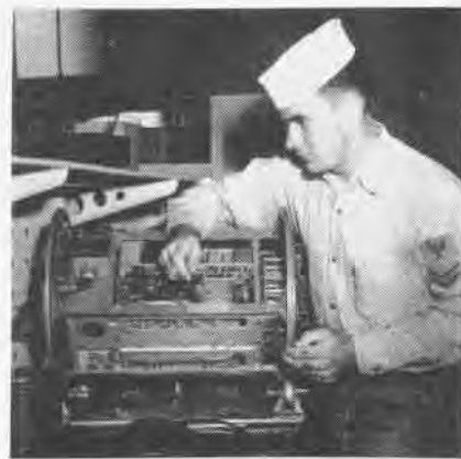
CHARLES R. WARMACK, AQ2, repairs an ARC-1 transmitter in squadron electronics shop.
