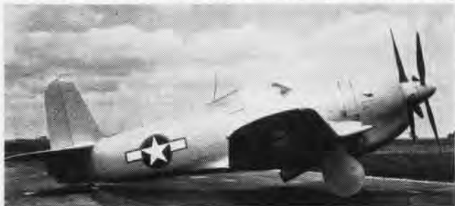
CURTISS XF14C-2 used 2500 hp turbo-supercharged Wright R-3350; speed of 398 mph was reached by this 14,950-lb high altitude fighter.
