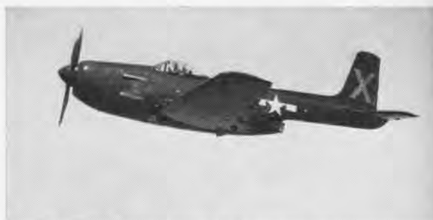
CURTISS XF15C-1 , last of Curtiss-Navy fighters, had composite power 2300 hp Double Wasp Plus Halford H-1B 2700-pound thrust jet.
