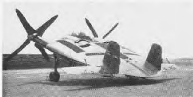
VOUGHT XF5U-1 would currently qualify as STOL. A speed of 476 mph was expected with two turbo-supercharged 1600 hp R-2000's.
