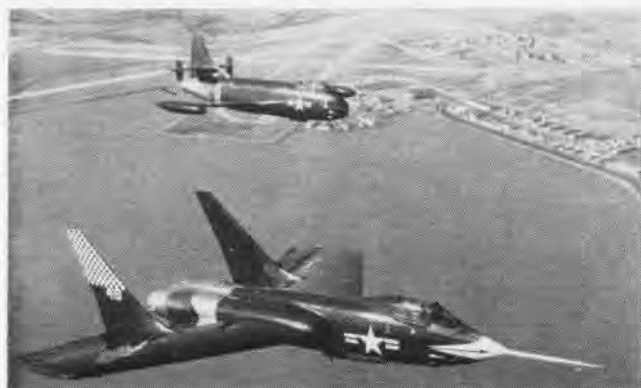
EARLY VOUGHT jets were F6U-1 Pirate and F7U-1 Cutlass, both using J-34's with afterburners. Later -3 Cutlasses saw wide service use.
