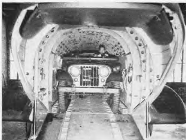
IN DEMONSTRATIONS using mock-up, a radio jeep is backed up rear ramp of the HRB-1. Stowed cargo booms serve as guides for jeep driver.
