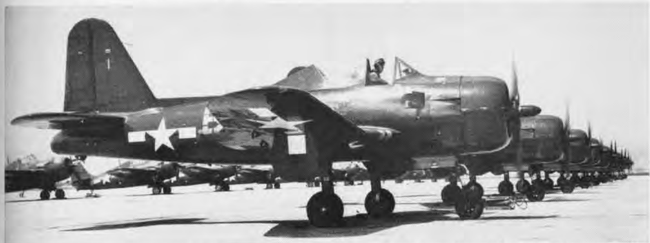
RYAN FR-1 FIREBALLS , composite powered with a 1400 horsepower Cyclone and a 1610-pound thrust General Electric jet engine, weighed
