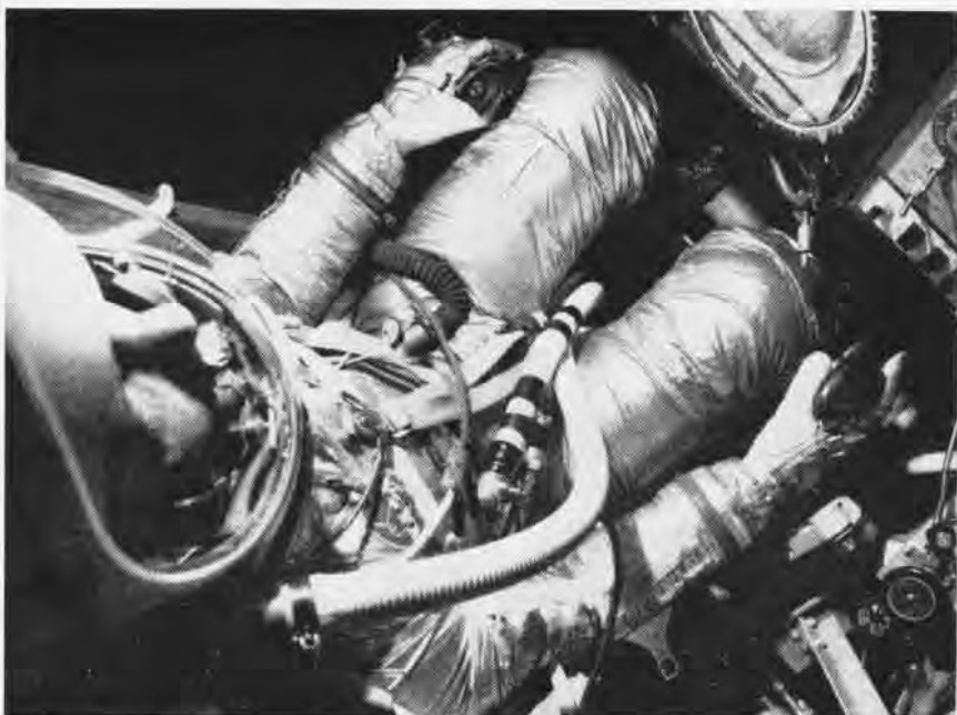
LT. COL. JOHN GLENN, USMC, Mercury Astronaut, attired in full space regalia, is subjected to Mercury type acceleration and low pressure profiles in gondola of Navy's human centrifuge.
