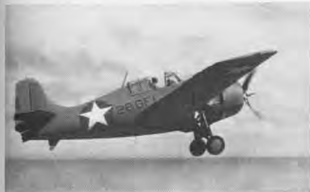
TYPICAL of World War II F4F/FM's, Grumman F4F Wildcat with 1200-hp Twin Wasp weighed 7400 pounds, attained 318 miles per hour.
