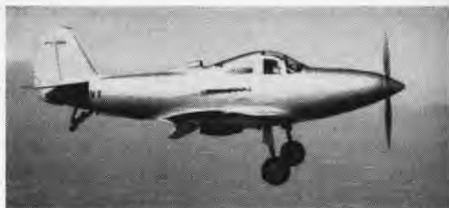
IN 1941 TESTS, Bell XFL-1 'Airbonita' with 1150 horsepower liquid-cooled Allison V-12 engine reached 333 mph; weight was 6740 lbs.
