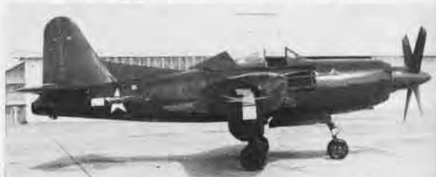
RYAN XF2R-1 was all-turbine powered version of FR Fireball; GE TG-100 turboprop rated at 1700 shaft hp replaced Cyclone in nose.
