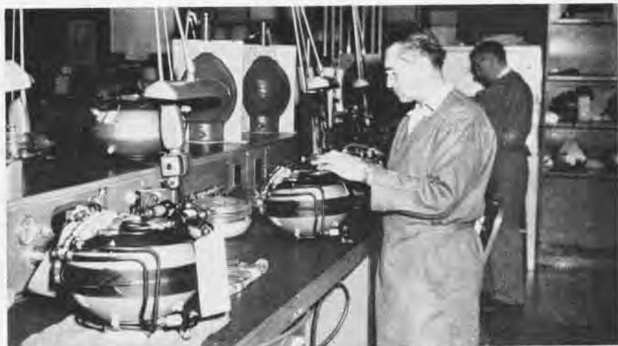
ALAMEDA HAS SUCCEEDED IN REBUILDING LIQUID OXYGEN CONTAINERS FOR $50 EACH
