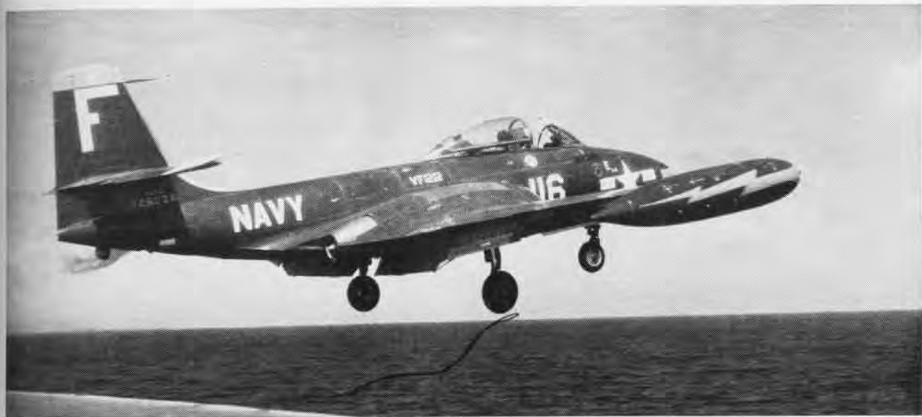
MCDONNELL F2H-2 Banshee saw extensive service in Korea. With two 3250-lb Westinghouse J-34 engines, it reached a speed of 590 mph
