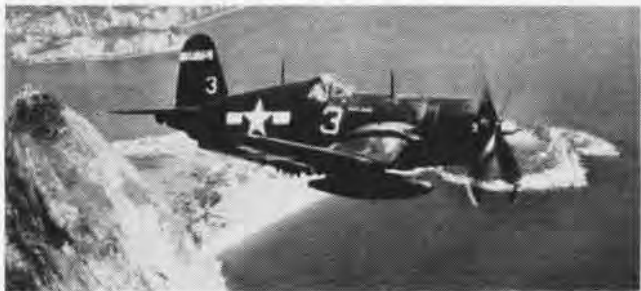
CORSAIRS SHARED honors with F6F's. F4U-4 served from late WW II on. Its speed was 446 mph; weight, 12,420 lbs; horsepower, 2380.
