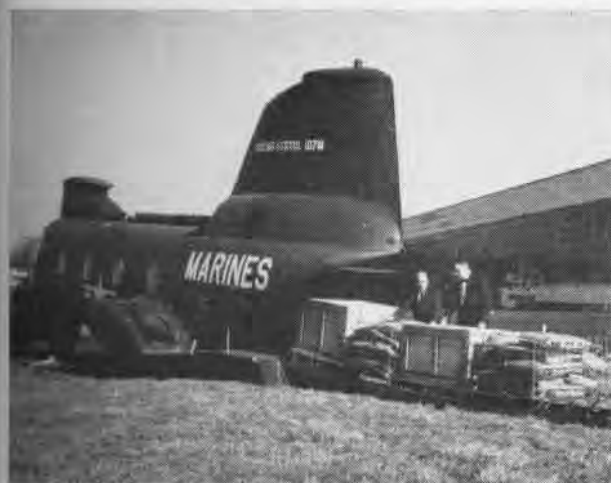
CARGO ON STANDARD pallets or litters can be pulled aboard by hydraulic winch at a rate of two tons in three minutes, by one operator.
