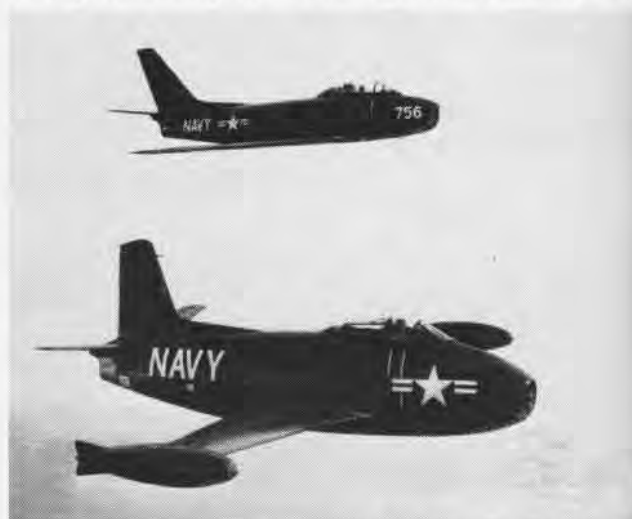
NAA F1-1 did 588 mph with 4000-lb J-35; XF1-2B, modified F86E prototype for sweptwing Furies, attained 678 mph with 6000-lb J-47.
