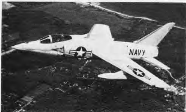
F11F-1 TIGER , Grumman's supersonic fighter, has A/B J-65. This one ran into shell fired from its own guns, "shot itself down."
