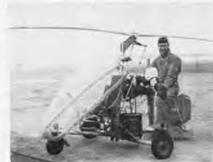
LCDR. GURLEY demonstrates bird on deck. Note two 5-gallon cans which carry supply of fuel.
