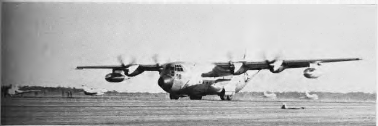
GIANT GV-1 TANKER ROARS DOWN MOBILE RUNWAY; 520-FOOT TAKE-OFF ROLL IS SAME DISTANCE REQUIRED FOR ITS LANDING
