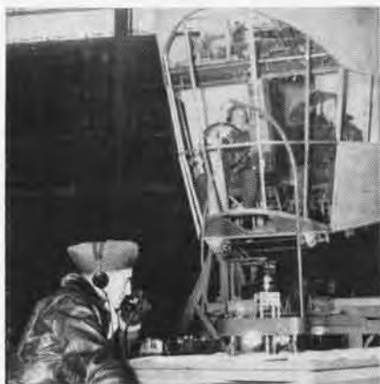
BOGUS BLIMP is trainer at Lakehurst in 1943. Operator could create various flight effects.
