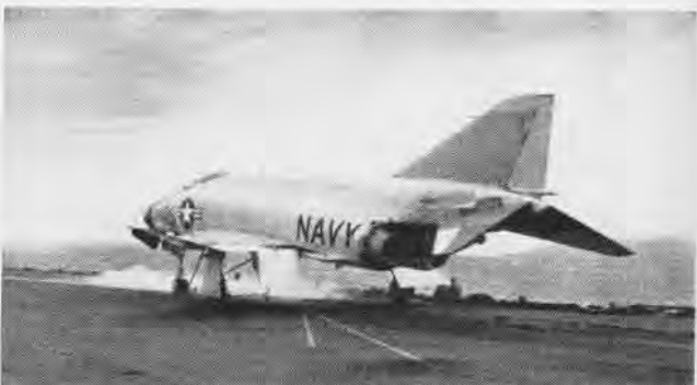
MCDONNELL'S PHANTOM II , two-place Mach 2-plus fighter with twin J-79's, can fly strikes in addition to all-weather fighter role.
