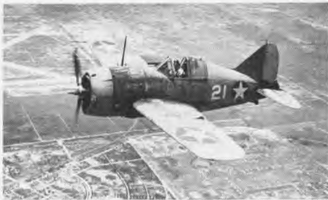
CYCLONE-POWERED Brewster F2A-2, used for fighter training in 1942, weighed 5940 lbs. Its speed was 325 miles per hour with 1200 hp.
