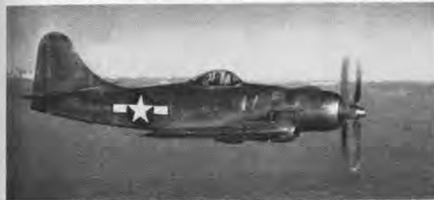
BOEING XF8B-1 was a 17,500-pound long-range fighter. It did 411 mph with a Wasp Major driving contra-props, had internal bomb bay.
