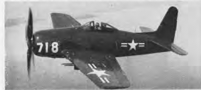
F8F-2 WAS IMPROVED Bearcat; weight was increased to 10,426 lbs, speed was 388 mph with 2500 hp Double Wasp. F8F-1 did 421 mph.
