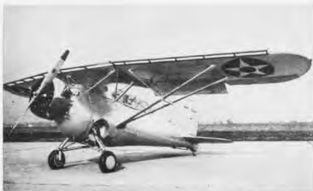
CURTISS XF12C-1 of 1933; with 625 hp twin-row Wright, this 5630 pound fighter reached 213 mph. It was later redesigned as XSBC-1.
