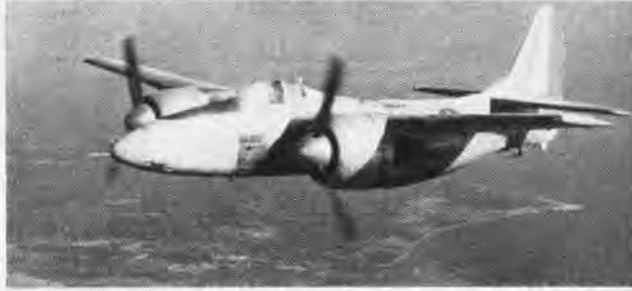
GRUMMAN XF7F-1, 19,500-lb Tigercat prototype, reached 398 mph with two 1800 hp Wrights; production F7F's had Double Wasps.
