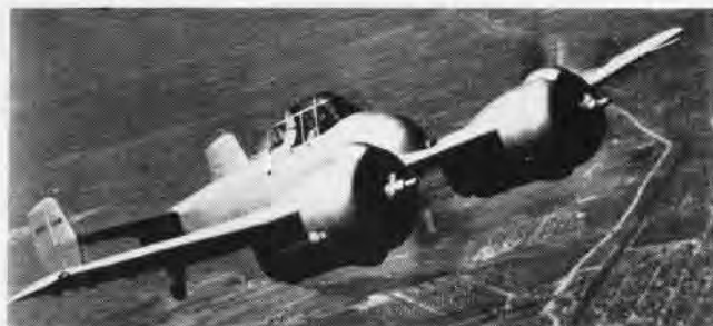
GRUMMAN 'SKYROCKET,' the experimental XF5F-1, had two 1200 hp Cyclones. With 9750 pound weight, it reached 348 miles per hour.
