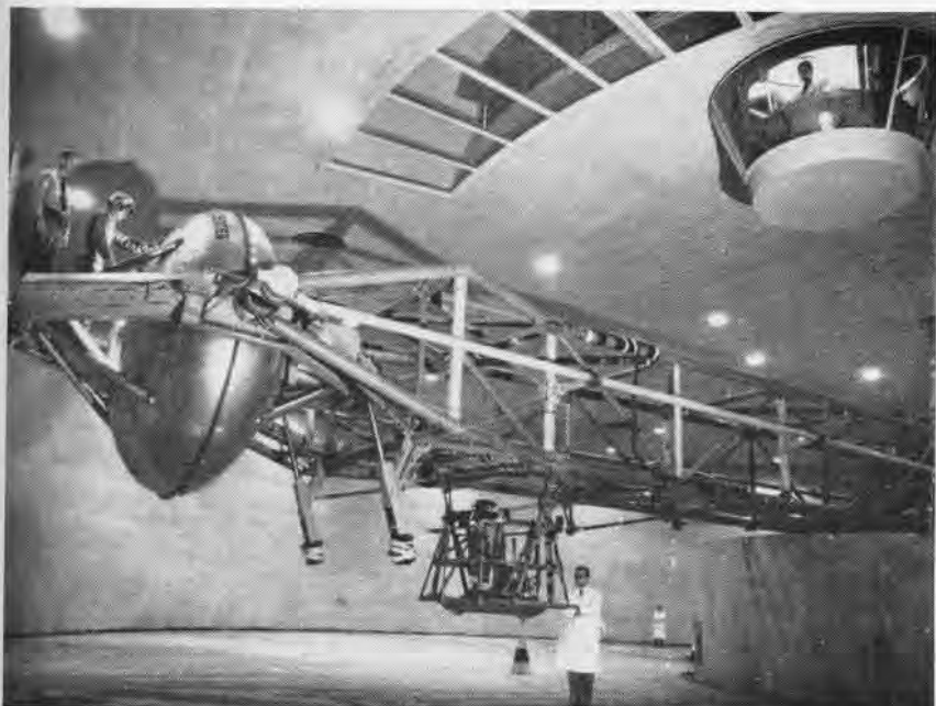
SUPER SIMULATOR at NADC Johnsville is world's largest human centrifuge. By linking it with "Typhoon" computer, flight profiles were enacted for NASA's X-15 and Mercury programs.
