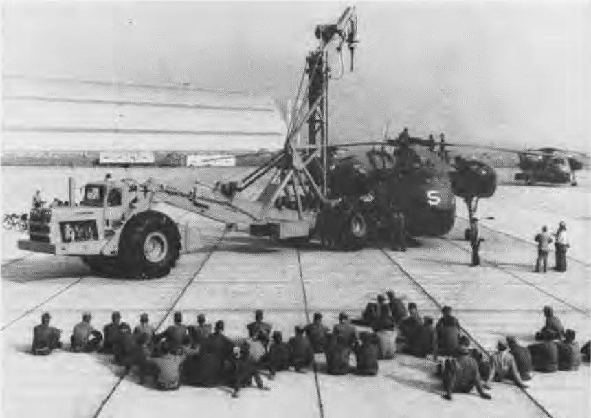
MCAF SANTA ANA crash crew demonstrates capability of new mobile crane which has just arrived. The 150,000-pound crane prepares to lift a 26,000-pound HR2S-1 helicopter. It can lift and move a 40-ton load. Faster and more efficient than the smaller one now in use to clear runways of accidents, the LSW crane will be used for helicopter repair and construction work. Santa Ana Marines received schooling on the crane's operation from a factory representative.
