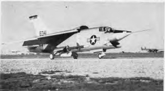
CRUSADER III , Chance Vought F8U-3, was single-place, missile armed Mach 2-plus all-weather fighter, powered by P&W J-75 engine.
