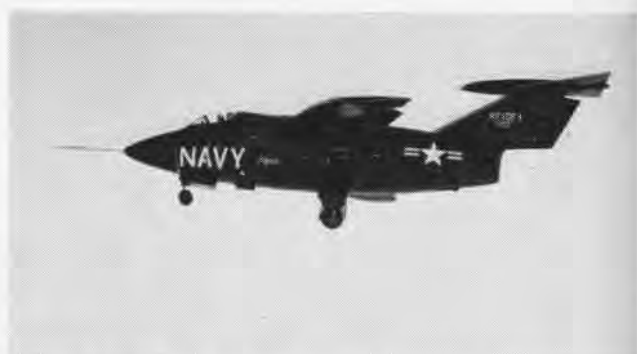
VARIABLE SWEEP wings were a feature of transonic Grumman XF10F-1 Jaguar. Designed around Westinghouse J-40, it flew in early 50's.
