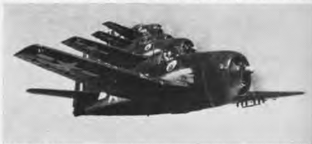
F6F HELLCATS were standard WW II carrier fighters; F6F-5 weighed 12,740 lbs, reached 380 mph with 2250 horsepower Double Wasps.
