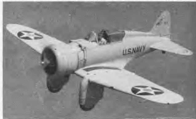
NORTHROP XFT-1 was early experimental low-wing fighter. High speed was 231 mph in 1935 tests with 625 hp Wright, 3840-pound weight.
