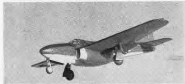
NAVY TESTS of the AAF YP-59's in 1944 showed 386 mph speed. Each had G.E. 1620-pound thrust engines. Weight was 10,500 pounds.
