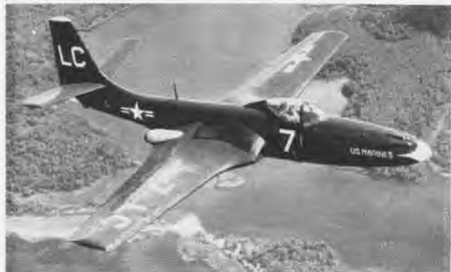
McDONNELL PHANTOM , the FH-1, with two J-30's, was production version of first jet design for Navy; weighed 9970 lbs, flew 485 mph.
