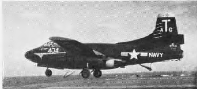
DOUGLAS SKYKNIGHT , the 2-place F3D-2 night fighter, reached 530 mph at a combat weight of 21,370 lbs with two 3400-lb J-34's.
