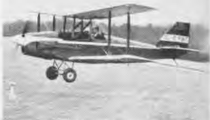
LATEST TURBINE-POWERED aircraft is flown. It is a British "Currie Wot," powered by Rover Co. Ltd. TP60 engine designed for automobiles. Company's 60 and 90 hp engines are said to be world's smallest turboprop acft. engines.
