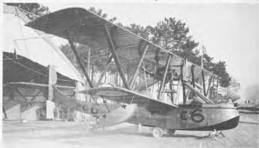
TELLIER FLYING BOAT, TYPE USED BY ENS. SMITH, WAS FRENCH SINGLE-MOTORED SEAPLANE
