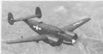
LOCKHEED PV-2 Harpoons were revised PV-1's in which wing and tail areas were increased.
