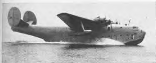
PROTOTYPE MARS was Martin XPB2M-1 which flew before our entry into WW II. It was powered by four 2000-hp Wright R-3550 engines.
