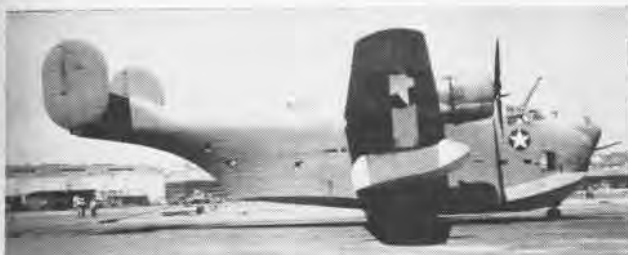
EXPERIMENTAL FLYING BOAT was early WW II Consolidated XP4Y-1, modified from twin-engine commercial type. Engines were R-3550's.
