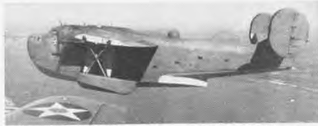
CONSOLIDATED XPB2Y-3 Coronado , powered by four 1200-horsepower Twin Wasps, was generally typical of 6 models of this flying boat design.
