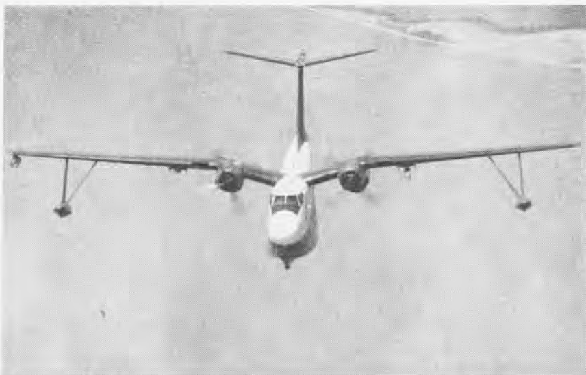
CURRENTLY, ONLY FLYING boats in service are the Martin P5M Marlin. P5M-2 has a T tail and both models have been modified with latest ASW equipment installed. Engines are two R-3350's.
