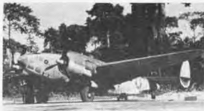
MARINES USED Vega PV-1 Ventura as night fighters; others were Navy patrol bombers.
