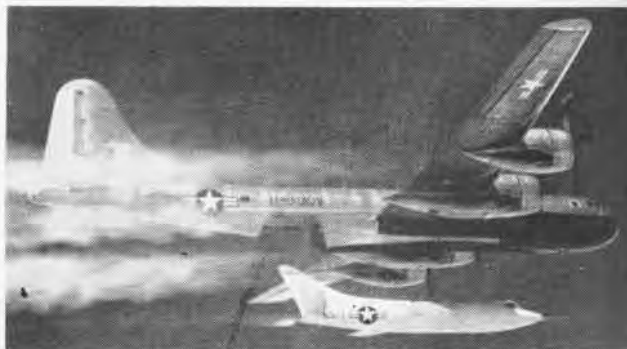
LAUNCHING A D-558-II Skyrocket is one of the four B-29's initially acquired by Navy as P2B's in order to evaluate them as ASW airplanes.
