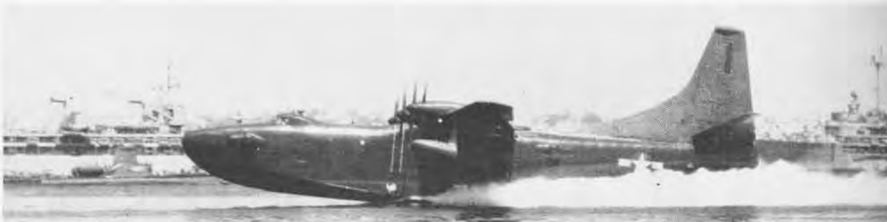
CONVAIR XP5-1 was one of the most ambitious projects being pursued by the Navy after World War II. With four Allison T-40's rated at
