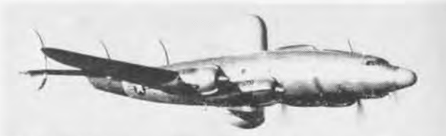
LOCKHEED PO-1W followed success of PB-1W's. Two of these were evaluated, leading to full scale production and service of WV-2's.
