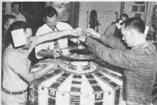
SCIENTISTS at Applied Physics Laboratory mask out solar cells during last minute circuitry tests which preceded the launch of Transit 4A .
