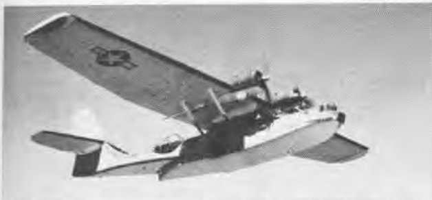
LAST VERSION of the Catalina produced by Consolidated was the PB4Y-6A amphibian, incorporating the PBN type tail, new radio and radar.
