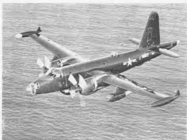
LOCKHEED P2V-7 Neptune is mainstay of VP squadrons' current ASW capability. Armament of earlier models is gone; latest ASW gear installed.
