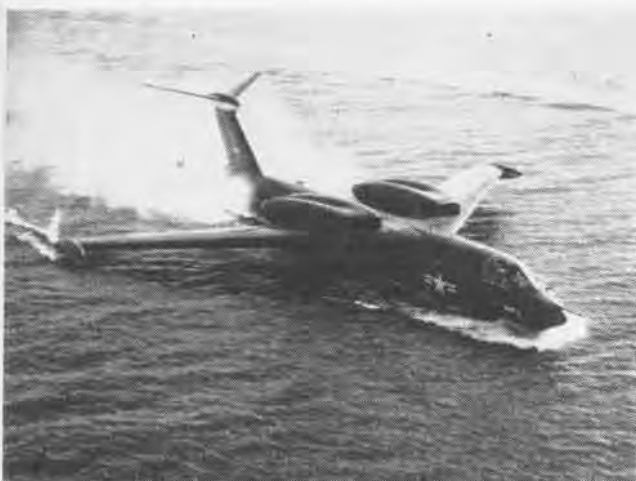
MARTIN P6M-2 was to be Seamaster production version, powered by four P-5W J-7's, capable of high speed bombing and mining missions.
