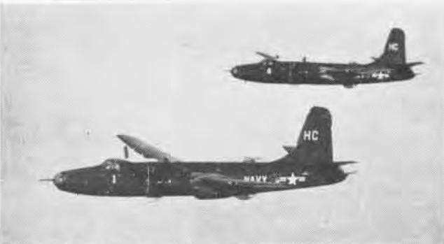
MARTIN P4M-1 Mercators had 3250-hp P&W Wasp Majors plus 4600 lb. thrust Allison jets for high speed in mine laying and attack missions.
