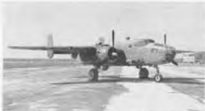
NAVY VERSION of B-23 Mitchell, NAA PBJ-1, featured ten .30 calibre guns and a radome.
