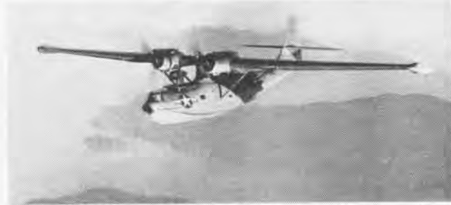
BOEING/CANADA-BUILT model of Catalina was PB2B-2, similar to PB4Y-6A but a flying boat. All Catalinas were powered by Twin Wasps.
