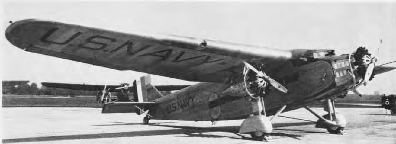
NAVY HAS generally depended on already developed transport aircraft. Thus Ford all-metal tri-motors, used by most U.S. airlines, were used as the JR (later RR) series. This JR-3 and its sisters were among Navy's first operational all metal cantilever monoplanes.
