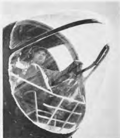
PLEXIGLAS nose of P2V houses a lookout who adds Mk. 1 eyeball to electronic search gear.
