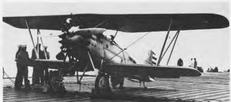
WITH THE INTRODUCTION of the air-cooled Pratt & Whitney Vash engine, a number of new carrier-based designs, such as the Boeing XF3B-1 aboard the Langley, were developed in the 20's.
