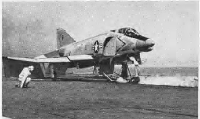
THE F4H-1 Phantom II, breaker of two world speed records at set distances, during carrier suitability trials on USS Independence.
