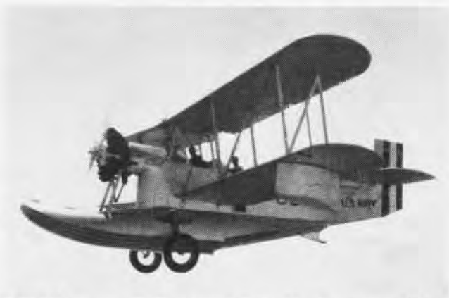
THE OL-8 was one of the series of outstanding Loening amphibians. Their versatility for many operational and utility missions led
