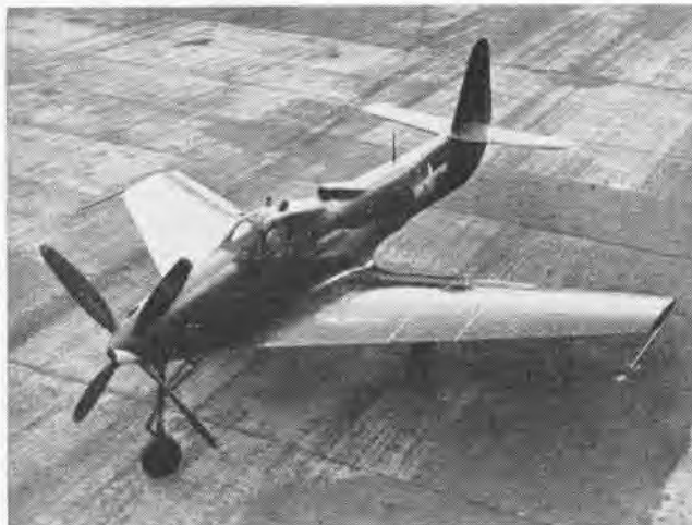
Bell L-39-2 , a contemporary of the XBT2D-1, was used to study low-speed characteristics of sweptwing designs during that period.
