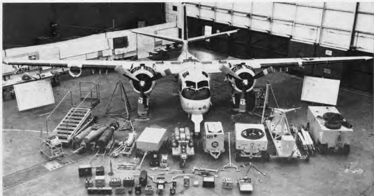
S2F-3, LATEST ASW aircraft, requires extensive support equipment. Quantity, cost, complexity, and bulk of equipment required to keep
