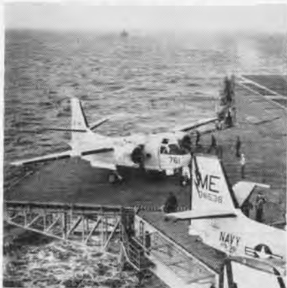
ELEVATOR DELIVERS S2F TO FLIGHT DECK
