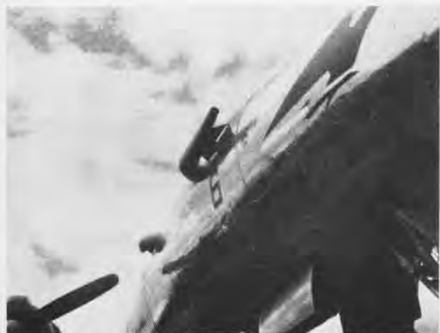
'BUG CATCHER' INTAKE PROTRUDES FROM FUSELAGE OF THE R7V
