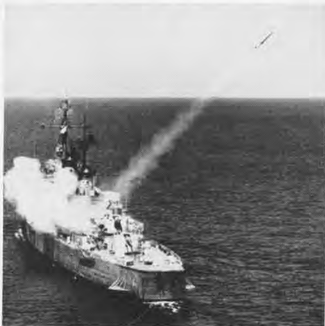
ASROC antisubmarine missile, featuring a homing torpedo, is fired from USS Norfolk during technical evaluation tests off Key West.
