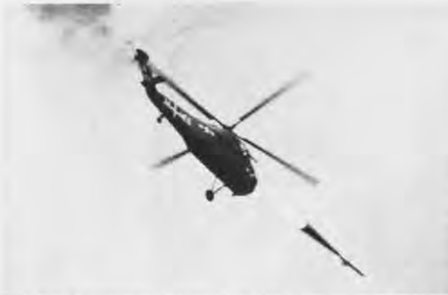
THE BULLPUP air-to-surface missile is fired from an HUS-1 Marine Corps helicopter in a series of tests conducted at NATC Patuxent.
