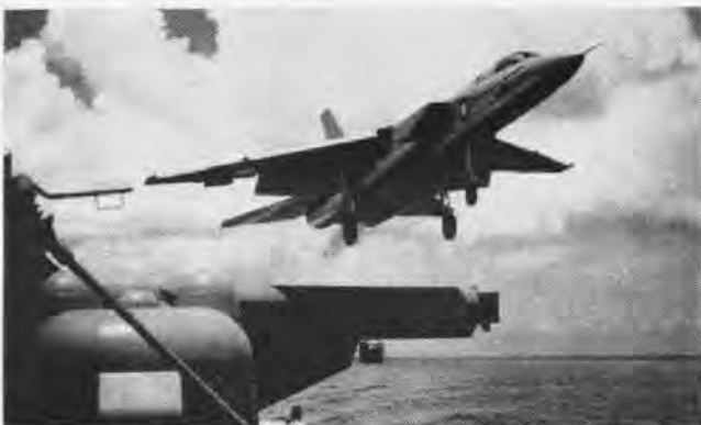
THE A3J Vigilante carrier attack plane on a touch-and-go landing during its carrier trials on the USS Saratoga early in the year.
