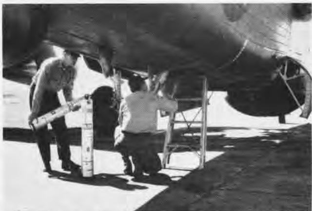
SONOBUOYS are loaded into the belly of a P2V Neptune by ground crewmen before the VP-812 plane takes off to hunt elusive subs.
