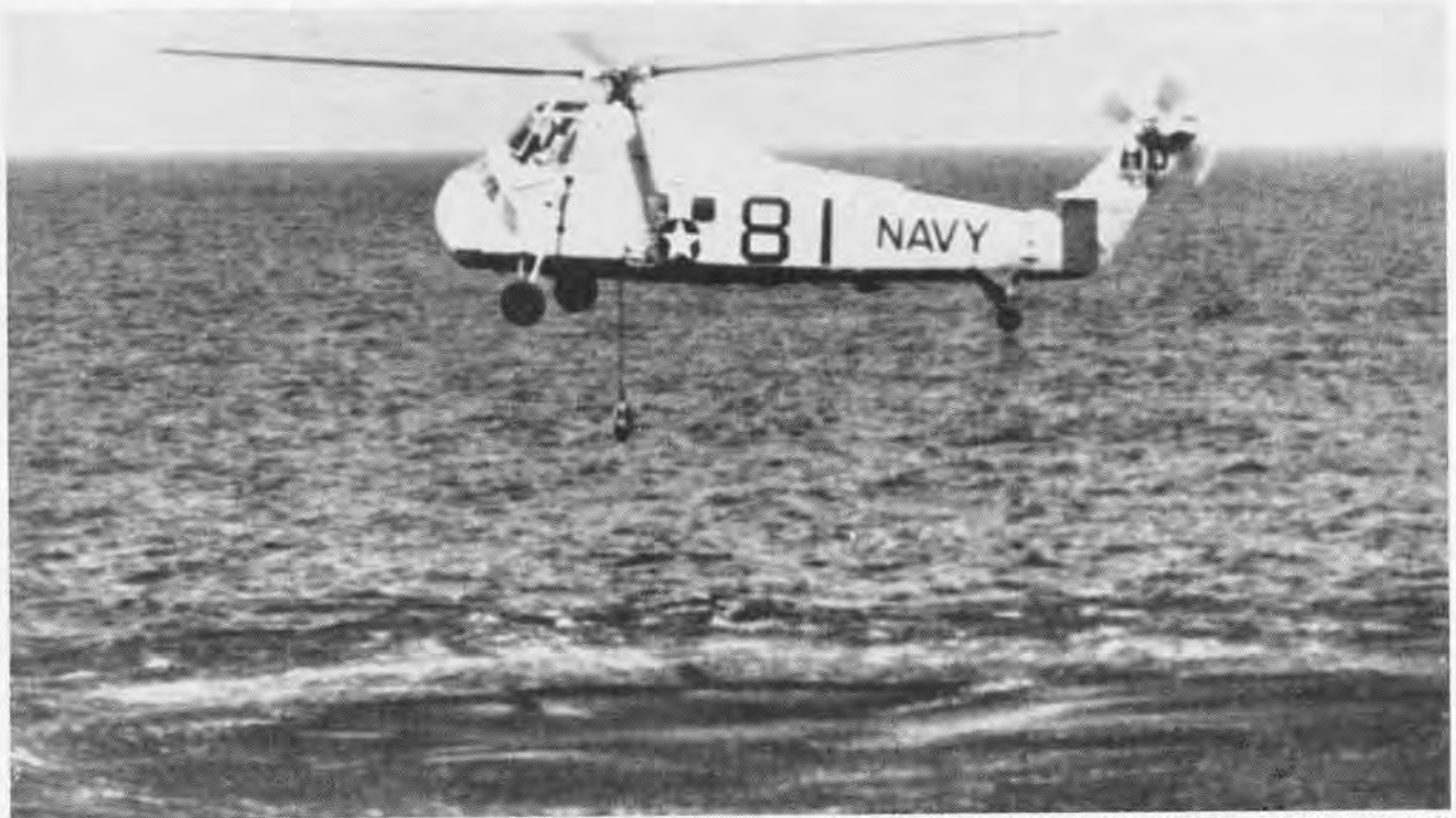
HSS HELICOPTER LOWERS SONAR EQUIPMENT INTO WATER. COPTER'S ABILITY TO HOVER WITH SEARCH EQUIPMENT IS BOON TO ASW
