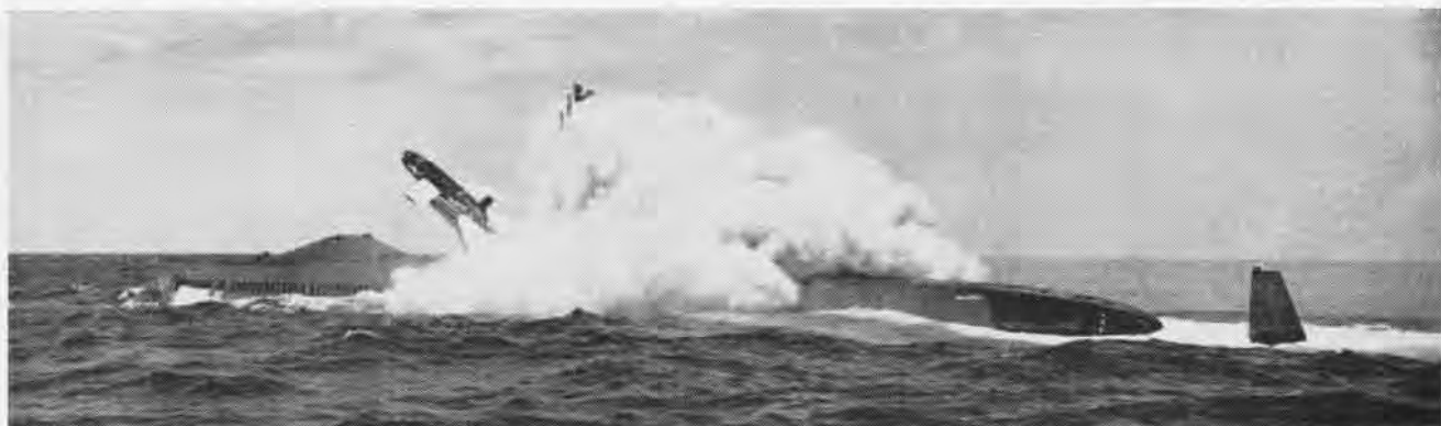
THE USS HALIBUT, SSG(N)-387, fires the Regulus I bombardment missile in training exercises off Oahu. This was the first firing of a
