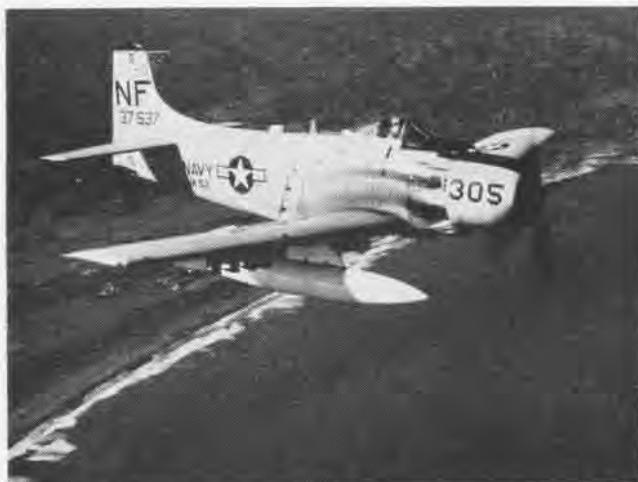
THE AD-6 , typical of the AD's which are still a mainstay in carrier ops, was evolved from the XBT2D-1 of the WW II period. The
