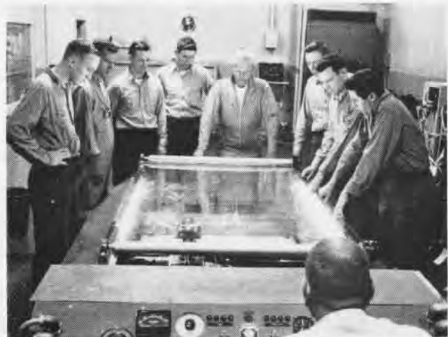
RADAR TRAINER is used to send signals to training scopes so the hunters can learn to detect subs and keep track of their position.
