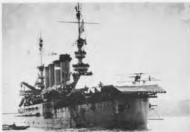
THE 120-FOOT PLATFORM , built on the stern of the USS Pennsylvania, was the forerunner of today's flight deck on Navy's aircraft carriers.
