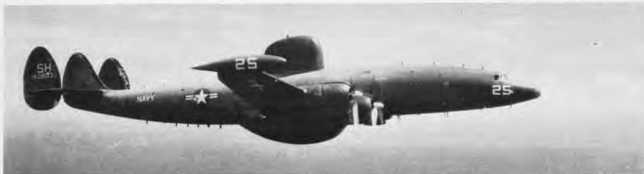
WEATHERMEN have had for several years a sturdy ally at sea, the Navy's WV-2, a Lockheed Super Constellation which can ride out a storm. Fully equipped with electronic gear, it is virtually a flying laboratory for meteorologists and is used by the Hurricane Hunters.
