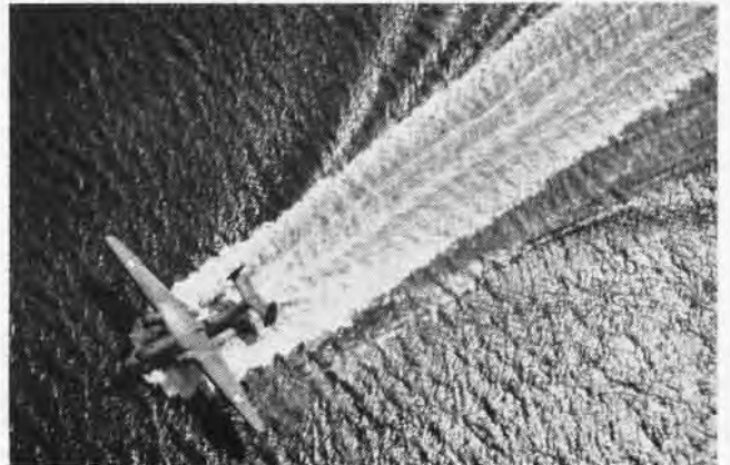
MARTIN MARINER, a twin-engine, gull-wing seaplane, was used for ASW patrol, convoy guard, over-water reconnaissance and cargo carrier.
