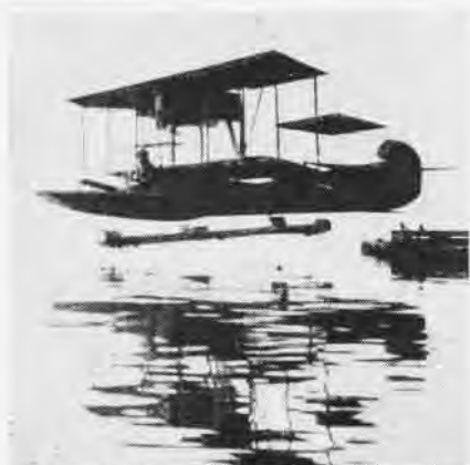
CATAPULT DOLLY (1912), once flying boat was successfully launched, went on its way.
