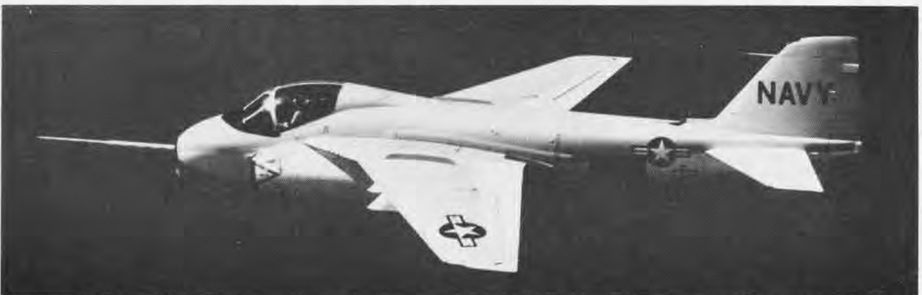
GRUMMAN'S A2F INTRUDER , a two-place, twin-jet, subsonic, carrier-based aircraft was designed for close support. It is the first Navy
