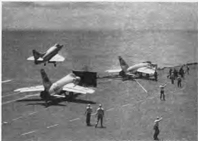
WHILE AN A4D Skyhawk is launched from angled deck, two F11F aircraft are readied for launching from port cat on USS Forrestal.
