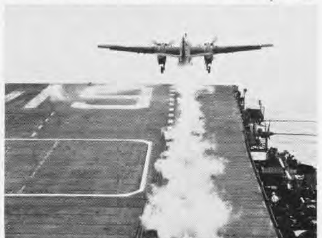
ELEVEN YEARS later, in 1954, USS Hancock showed the modern steam catapult in action for the first time by launching a Grumman S2F.
