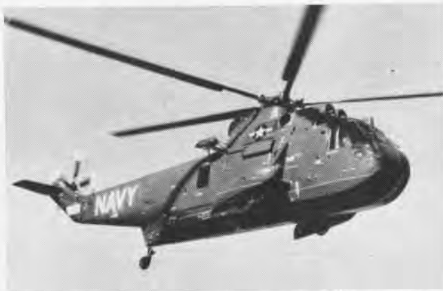
THE WORLD'S largest amphibious helicopter, the HSS-2, is a turbine-powered, all-weather aircraft developed for the Navy by Sikorsky.
