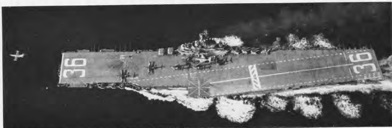
USS ANTIETAM (CVA-36) has the great distinction of being the first carrier in the world on which the angled deck was installed. Shown
