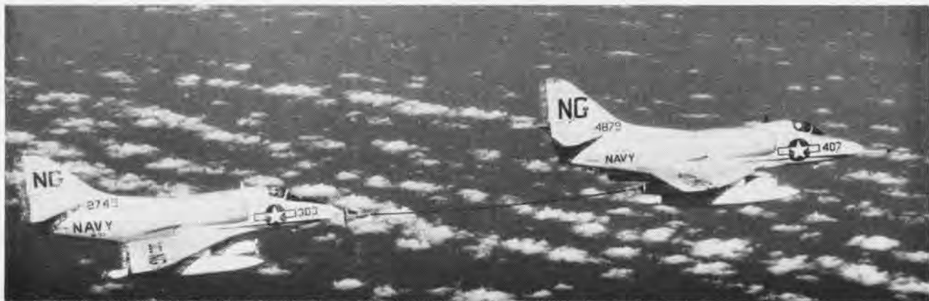
BUDDY REFUELING BY A PAIR OF A4D SKYHAWKS PROVIDES EXTENDED RANGE. LEAD PLANE RETURNS TO CARRIER, OTHER CONTINUES
