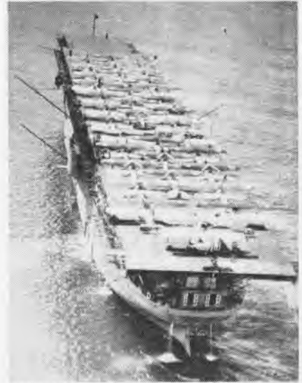
HER FLIGHT DECK , 534' x 64', about the size of World War II's famed "baby flattops."
