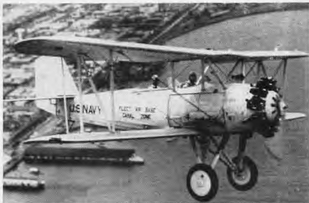
THIS CHANCE VOUGHT O2U-3 plane, assigned to Fleet Air Base, Canal Zone, represents the scout-observation types used in 1928-1933 period.
