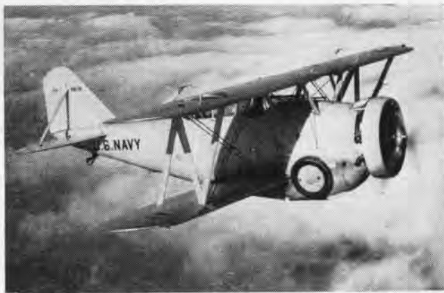
DELIVERED in 1933, the Grumman FF-1 was the first of an illustrious line and the first Navy fighter equipped with retractable landing gear.
