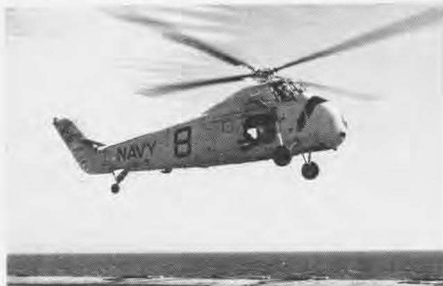
IN ANTISUBMARINE warfare, helicopters especially designed for search are proving themselves, as typified by this HSS-1, skilled participants.
