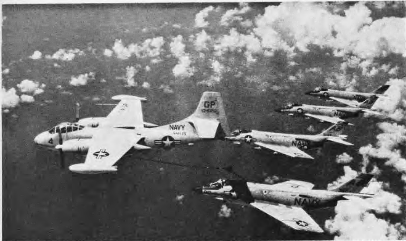
ORIGINAL NAVY TANKER WAS AJ-1 SAVAGE, SHOWN REFUELING FLIGHT OF VF-14'S F3H DEMONS IN 1958. AJ HAS BEEN RETIRED
