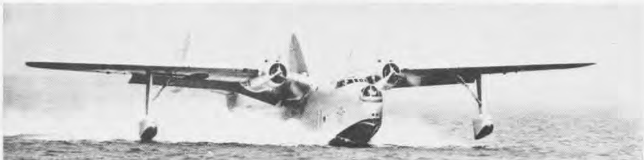
GULL WING of Martin XPBM-1, which initially flew in 1937, is still familiar on the P5M Marlin operated in VP squadrons today. Prototype of the WW II Mariners was powered by two 1600-hp Wrights. With normal take-off weight of 40,500 lbs, max speed was 223 mph.
