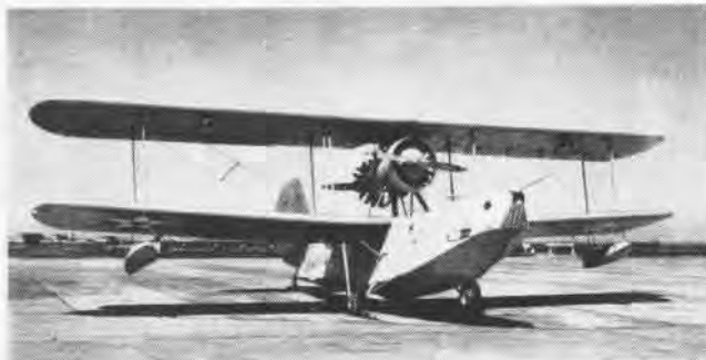
BUAER DESIGN for VP amphibian served as basis for experimental tandem engine Sikorsky XP2S-1 of 1932. Engines were P&W Wasps.
