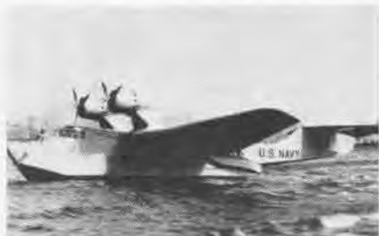
COMPETITIVE with XP3Y-1 was XP3D-1 using same engines. Wing was hull mounted.
