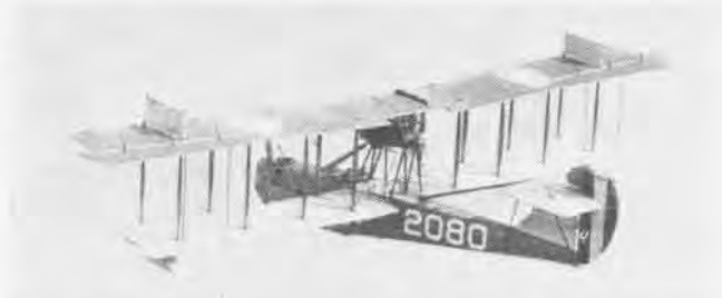
ANTI-SUBMARINE patrols off European coast were flown by Curtiss HS's. HS-2L had 350 hp Liberty, weighed 6400 lbs., reached 82 mph.
