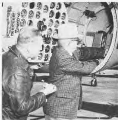
BAROGRAPH is started and sealed in the nose of F4H by observers prior to the record try.
