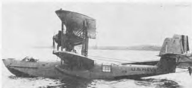
WRIGHT CYCLONES powered this 1930 XP4N-1, one of the last Naval Aircraft Factory series of flying boats. Its range with take-off weight of 17,900 lbs. was 1510 miles, its maximum speed was 115 mph.
