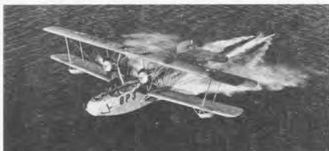
TOUCHING DOWN is Martin PM-1, one of 53 PM's built in early Thirties. With 525-hp Cyclones, 15,800-lb take-off weight, maximum range was 1330 miles. Later PM-2's had enclosed cabin for pilots.
