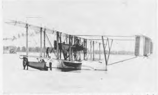
NC-9 , one of six NC's, built by NAF after 1919 trans-Atlantic flight. With four Liberties, its weight was 28,000 lbs., its speed 85 mph.
