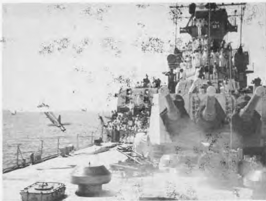
KD DRONE TARGET IS LAUNCHED FROM FANTAIL OF USS ST. PAUL FOR MISSILE SHOOT
