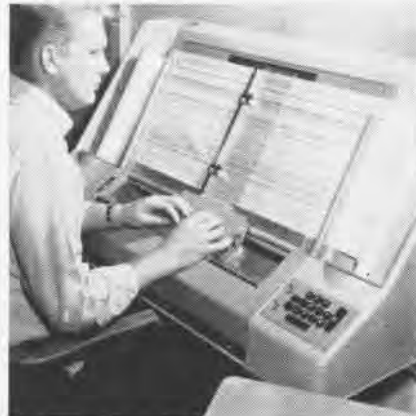
DATA ENGINEER reduces instrumented data after pre-Bendix tune-up flight by F4H-1.
