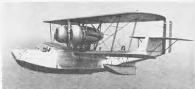
HALL-ALUMINUM XPH-1 was prototype of lighter weight biplane design. Later production versions were in Coast Guard service in early WW II. Note beaching gear carried in rear cockpit and between wings.
