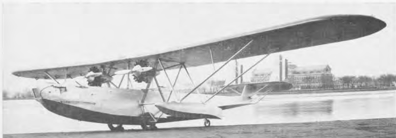
MAJOR ADVANCEMENT in flying boat design was seen in Consolidated's XPY-1 in 1929. It was a parasol-wing monoplane, powered by two 450-hp P&W engines. Alternate power plants were three Whirlwinds,
