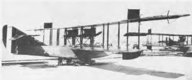
TYPICAL CURTISS H-series flying boat design, the H-12 of 1917 vintage was used by both the British and the U.S. Navy in WW I.
