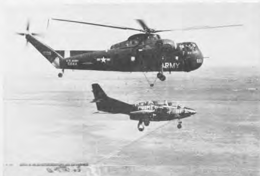
LOW AND SLOW , this 5800-lb T2J Buckeye jet trainer is carried by an Army HH-37 Mojave helo from NAAS Kingsville to NAS Corpus Christi. Disabled jet was then loaded aboard USS Antietam and transported to NAS Pensacola for repair. Cooperative effort which saved dismantling and lengthy floundered move of jet was arranged by Army Maintenance Center and 45th Helo Battalion of Fort Sill upon the request of Leo Emmert, BuWeps Fleet Support Representative.
