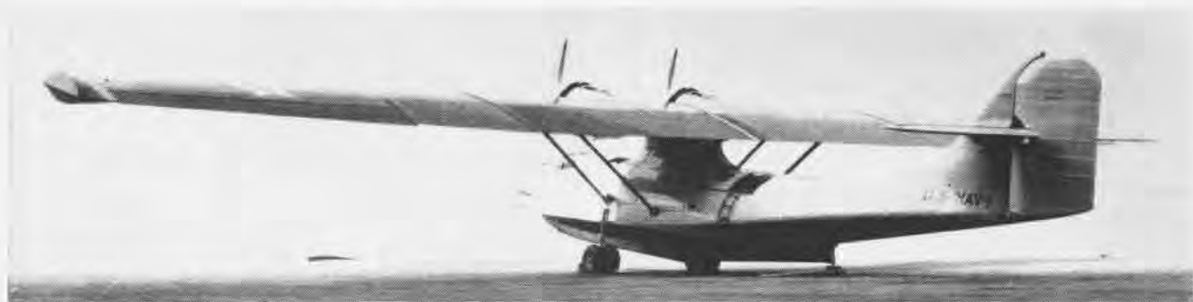
PROTOTYPE of the Catalinas of WW II fame was the Consolidated XP3Y-1 of 1936. Featuring the then-new P&W Twin Wasp of 800-hp, its maximum speed was 169 mph. Weight was 19,800 lbs. Range of streamlined boat was demonstrated in several distance record runs.
