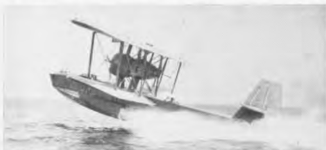
STREAMLINED NACELLES and cowlings were features of Keystone PK-1. Open cockpits remained. With Wright Cyclones rated at 575 hp, speed was 120 mph. Eighteen of these boats entered Navy service in 1931.
