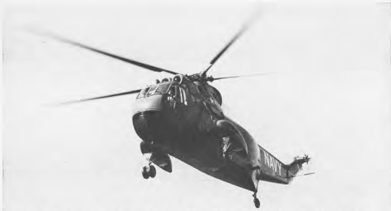
BOAT-HULLED, TURBINE-POWERED SIKORSKY HSS-2 WHICH BROKE RECORDS WILL SOON ENTER FLEET SERVICE WITH THE ASW FORCES
