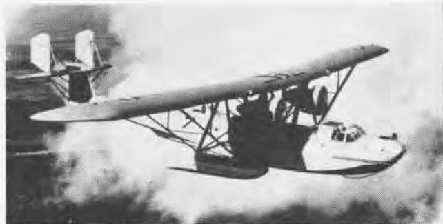
MARTIN P3M-5 were production versions of XPY-1. The P3M-2 shown above had 525-hp P&W Hornets in place of Wasps in the -1 models.
