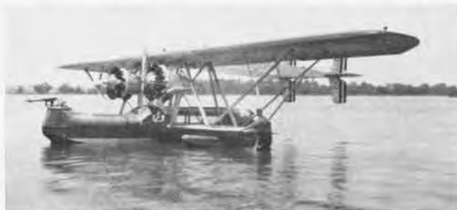
SIKORSKY AMPHIBIANS , adapted as VP types from commercial S-38 design, included PS-3 of 1929. Engines were P&W 450-hp Wasps. PS's became RS's with armament removed; served utility squadrons.
