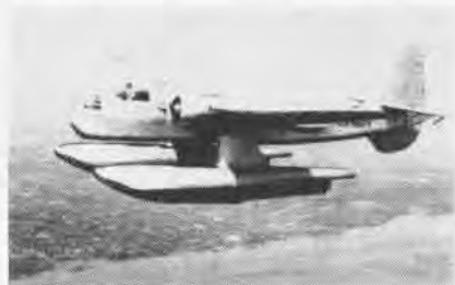
TORPEDO-BOMBER was principal mission of 1937 twin-float Hall Aluminum XP7B-1.
