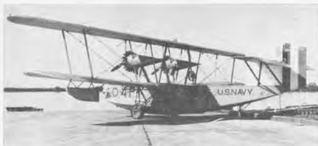
PRODUCTION flying boat based on PN series was Douglas PD-1. First of 25 was delivered in 1929. With 525-hp Cyclones, its maximum speed was 121 mph. Detachable beaching gear replaced early cradles.
