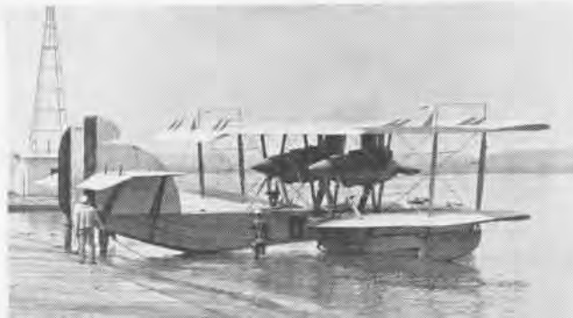
WRIGHT T-2'S of 325-hp powered the NAF PN-7 of 1923. Speed was 104 mph, its weight was 14,400 lbs., its range about 700 miles.
