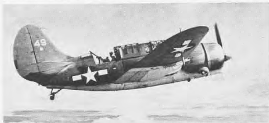
CURTISS SB2C Helldiver series underwent many changes before entering combat in late 1943. SB2C-1C and later versions replaced almost all SBD's in dive bomber squadrons by war's end.
