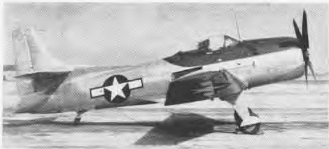
MOST STREAMLINED appearing and smallest of the late WW II VBT prototypes were Kaiser-Fleetwings XBTK-1's with P&W Double Wasps.
