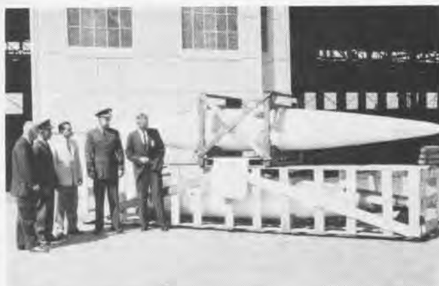
COST-CUTTING TEAM inspects drop tank packaging exhibit; old type packaging in full crate as against sensible picture frame type.
