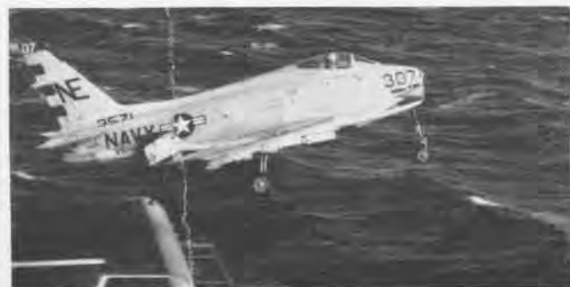
JET FIGHTERS were regularly assigned to VA squadrons. FJ-4 was specially modified for this role as FJ-4B with increased strength.
