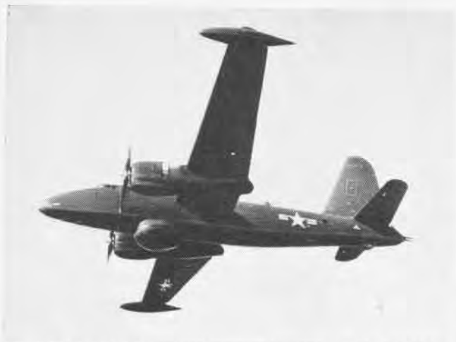
HALLMARK OF -4 WAS TURBO-COMPOUND ENGINES, BIG RADOME
