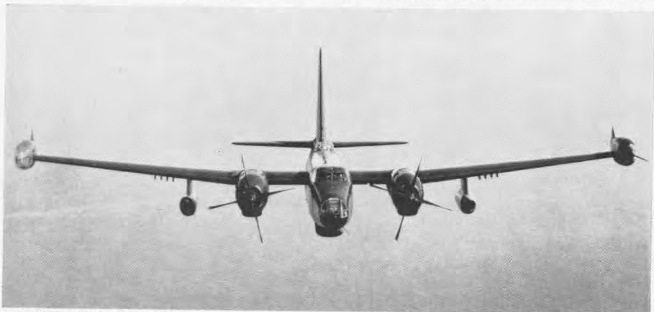
PILOT OF THIS P2V-5F DEMONSTRATES USE OF WESTINGHOUSE JETS ONLY, WITH PISTON ENGINES SHUT DOWN, PROPS FEATHERED
