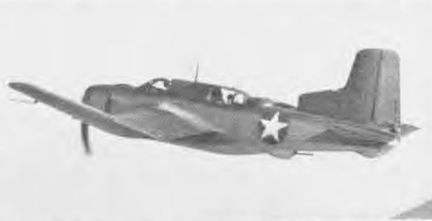
DESTROYER was name given early WW II Douglas XSB2D-1, a heavy attack plane prototype with remotely controlled aft power turrets.
