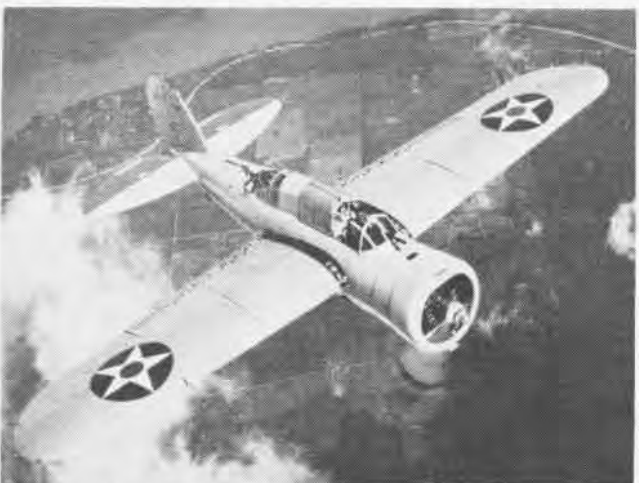
FIRST AIRPLANE designed and built by Brewster, previously a float manufacturer for Navy, was the XSBA-1 powered by an 850-hp Cyclone.
