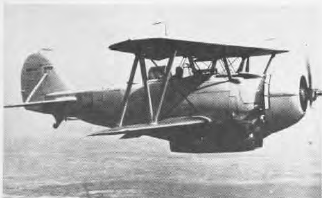
IMPROVED Great Lakes design of 1935 was XB2G-1, which competed with XBT-1. Retractable gear and internal bomb bay were features.
