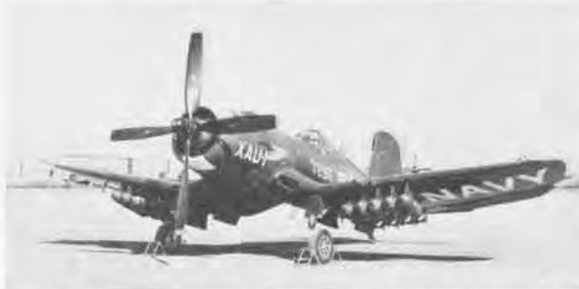
VOUGHT CORSAIRS that were used for ground attack in Korea led to production of the AU-1 version with increased wing store stations.
