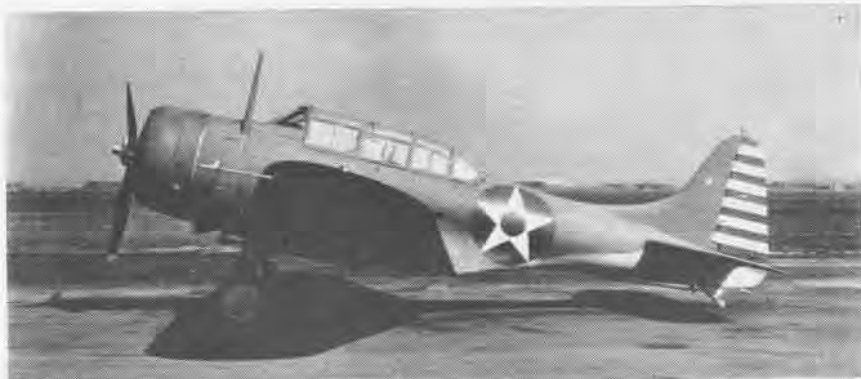
DOUGLAS SBD-4 was production version of Dauntless series at the outset of WW II. It is shown with early WW II markings. Powered by a 1000-hp Wright Cyclone, its top speed was 250 mph.
