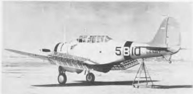
NORTHROP BT-1 entered service in 1938, hit 225 mph with 825-hp P3W. Perforated split-flap dive brakes typify WW II dive bombers.
