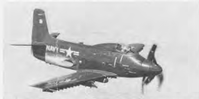
TURBOPROP POWERPLANT , 5000-hp Allison T-40, was feature of Douglas A2D-1 Skyhawk. Program was terminated in favor of AD's, jets.
