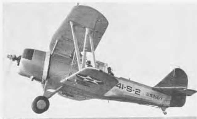
FIRST SCOUT-BOMBER in service was Vought SBU-1. Capable of delivering 500-pound bomb, its speed was 205 mph with a 750-hp P3W.
