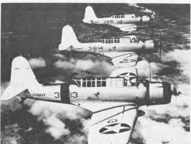
VOUGHT VINDICATORS fought in early WW II; first entered service as SB2U-1 in late 1937. With 825-hp P3W, their speed was 250 mph.
