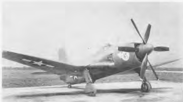
CONTRAPROPS were feature of the Curtiss XBTC-2, first single place attack design. It was powered by a 3000-hp P&W Wash Major.
