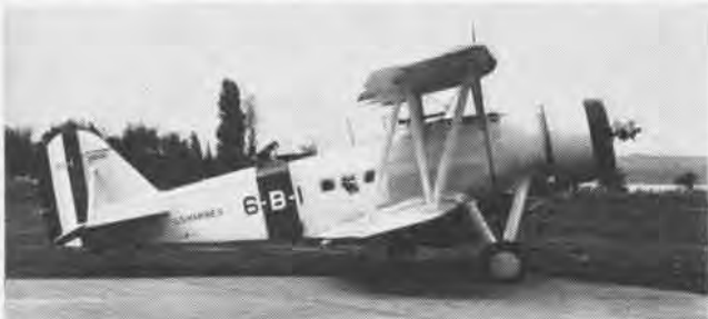
MARINES still flew Great Lakes BG-1's in 1940. Entering squadron service in 1934, they were powered by 700-hp P3W Twin Wasp Jr.'s.
