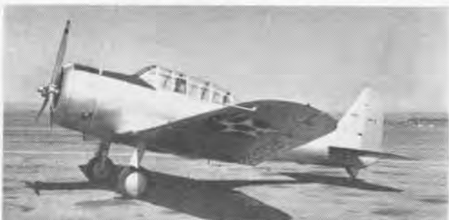
1000-HP CYCLONE in place of 825-hp P3W and fully retractable landing gear were improvements in XBT-2, prototype of SBD Dauntless.
