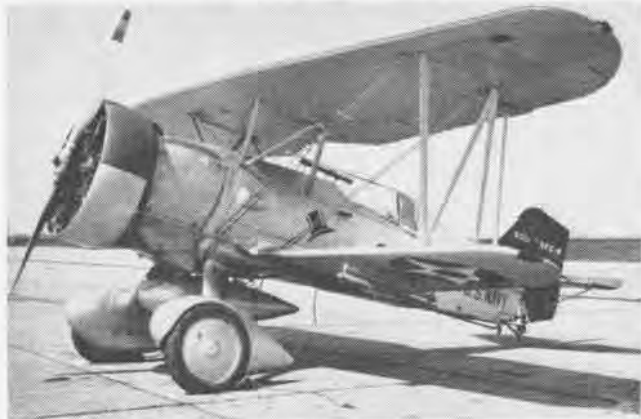
MOST FIGHTERS doubled in attack role. Curtiss F11C-2's were redesignated BFC-2's for bombing squadrons; used 600 hp Wright Cyclone.
