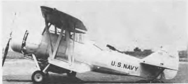
CONSOLIDATED XB2Y-1 prototype competed with XBG-1. Both were based on BuAer design, were capable of delivering 1000-lb bombs.
