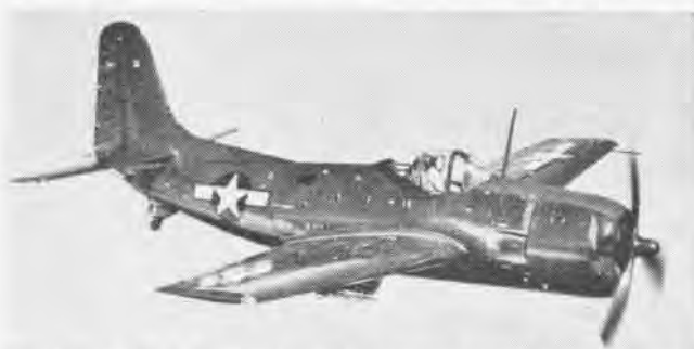
CURTISS XBT2C-1 was based on SB2C design modified to use R-3350. Unlike other late WW II VBT's, it retained an internal bomb bay.
