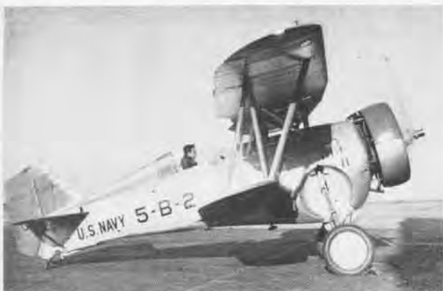
CURTISS BF2C-1 was final Navy model of famed Hawk series. Metal wing structure and retractable gear were improvements over BFC-2.
