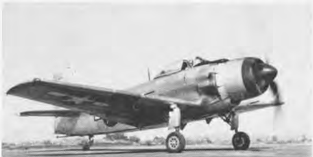
MOST SUCCESSFUL of the late WW II designs was the Douglas XBT2D-1. With Wright R-3350's, 25 XBT2D-1's preceded the AD Skyraiders.
