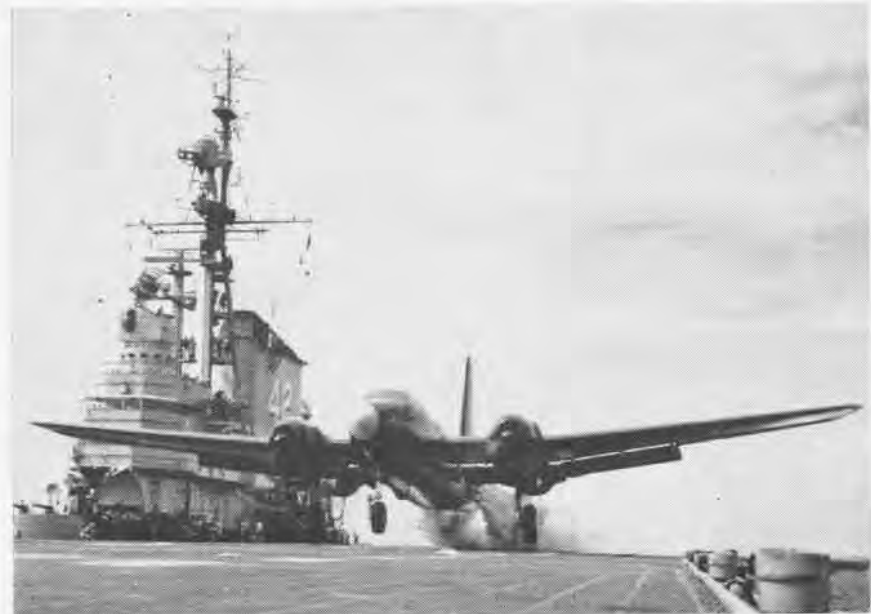
P2V-3C'S USED JATO THRUST TO TAKE OFF FROM USS FRANKLIN D. ROOSEVELT IN 1950
