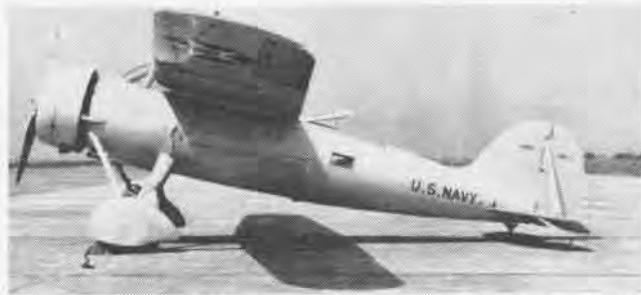
CONSOLIDATED Fleetster commercial design was adapted into XBY-1 carrier based horizontal bomber; was powered by a 600-hp Cyclone.
