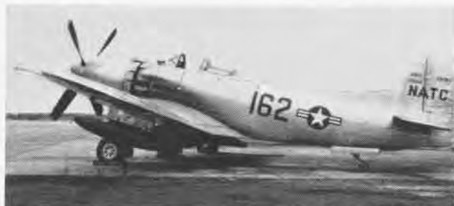
PROTOTYPES of the Martin AM-1 Maulers were the XBTM-1's, largest of the VBT designs, powered by the Pratt & Whitney Wash Major.
