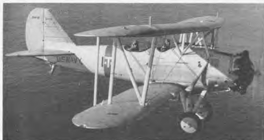
MARTIN dive bombers, including this BM-2, were capable of delivering a 1000-pound bomb. Entering service in 1932 they had metal fuselages, reached 145 mph with 600-hp P&W Hornet.
