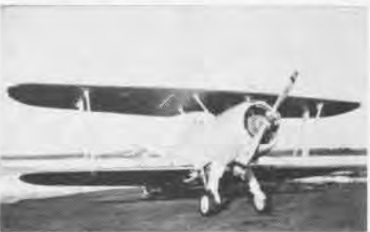
RETRACTABLE landing gear version of the SBU was the XSB3U-1 prototype built in 1936.
