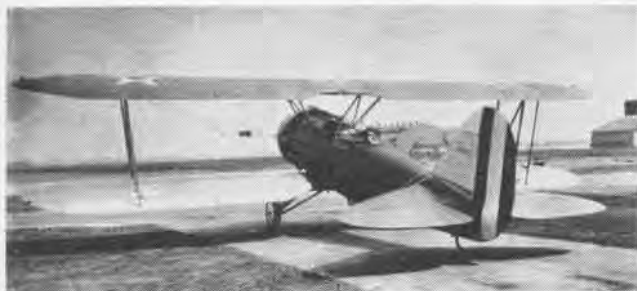
NAF XT2N-1 dive bomber was tested together with similar Martin XT5M-1, prototype of BM series. Both were based on BuAer design.
