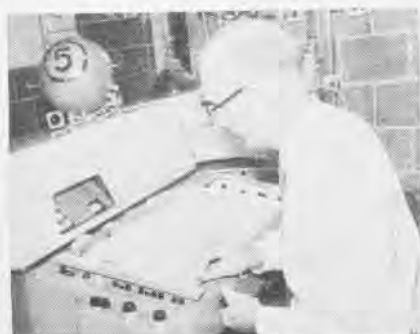
CHEMIST Rufus A. Whitmire tests a liquid oxygen sample using an infra-red photospectrometer at O&R Pensacola Materials Testing Laboratory. All continental U.S. O 2 supplies are monitored by a test lab.
