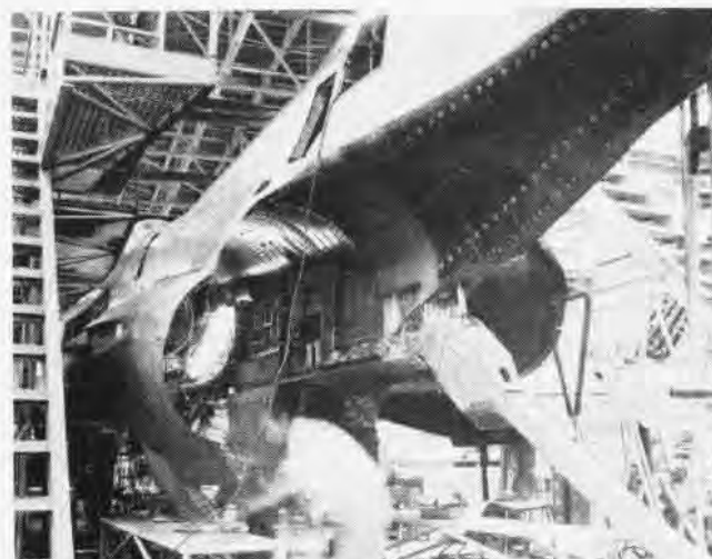
SHOWN HERE are left engine compartment details. Forward fuselage assembly is accomplished by fabrication of left and right halves.
