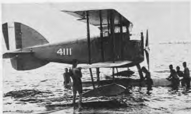
TWO-PLACE Curtiss HA "Dunkirk Fighter," seaplane of 1918, weighed 3620 lbs. to del., did 127 mph with 380 horsepower Liberty engine.
