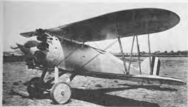
WRIGHT F3W-1 Apache of 1926 became famous for altitude record flights, reached 162 mph with early 375-hp Wasp, weighed 2130 pounds.
