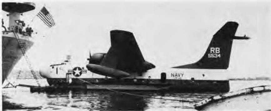
USS SALISBURY SOUND has inaugurated a new "fill 'em up" and maintenance service station which it describes as the "only trailer hitch afloat." The fueling dock allows the 15,000-ton seaplane tender to speed up greatly the refueling and servicing of her P5M Marlin seaplanes. The 42-foot dock can be placed in operating condition in from 30 to 45 minutes. AV-13 commanded by Capt. J. D. Ramage, serves as the flagship of Commander, Taiwan Patrol Force.
