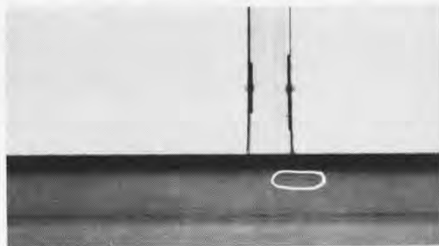
ROTOR BLADE failure can begin with defects, such as this bit of wire imbedded in the spar interior which causes stress concentration.
