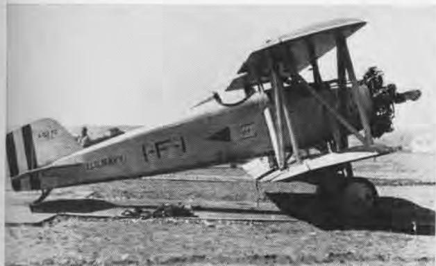
EARLY CARRIER fighter, the TS-1, was built by Curtiss and NAF in 1923, did 125 mph, weighed 1920 lbs., 200 hp Lawrence/Wright J-1.
