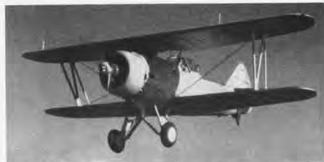
BASED ON same BuAer design as XFD-1 was Vought XF3U-1. With same engine, it weighed 4620 lbs., reached speed of 214 miles per hour.
