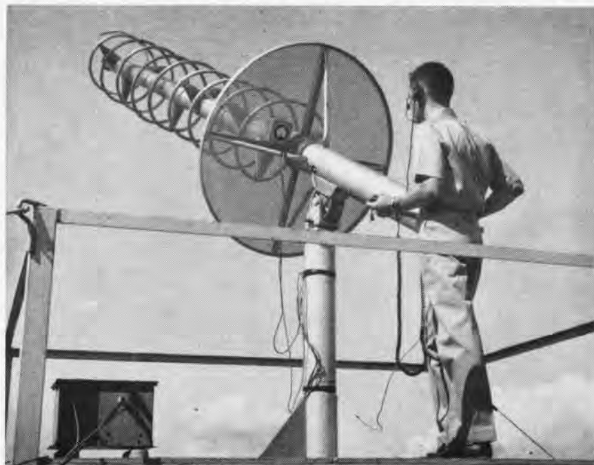
SIGNALS FROM SPACE are monitored aboard PMR range ship, USNS Longview, as Discoverer capsule descends from orbit. Year 1960 saw installation of Transit and Mercury tracking gear.
