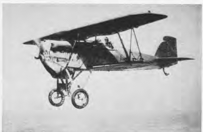
CONTEMPORARIES of the Hawks, were the Boeing FB series; FB-5 used 520 hp Packard 2A-1500, weighed 3290 pounds, reached 170 mph.
