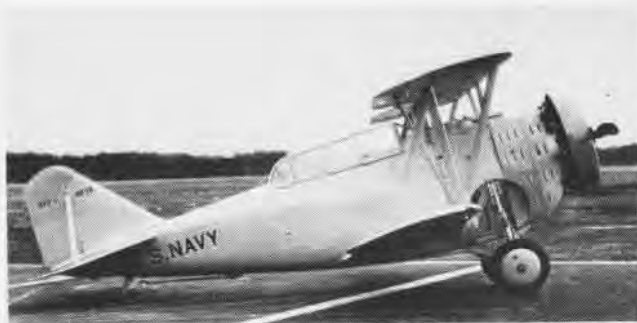
FIRST GRUMMAN airplane as it originally appeared in 1931, the XF-1, weighed 4470 lbs., later reached 208 mph with 600-hp Cyclone.
