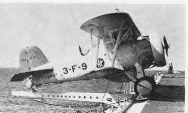
SHOWN ON RANGER outrigger, F4B-4 with 500-hp Wasp entered Navy and Marine service in 1932; weight was 3090 lbs., speed 184 mph.
