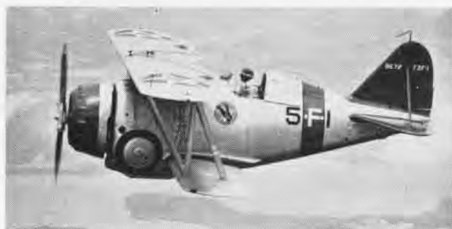
SERVICE F2F-1'S were delivered in 1935. These Grumman's weighed 3800 lbs., were powered with 650-hp Twin Wasp, Jr. ; made 231 mph.
