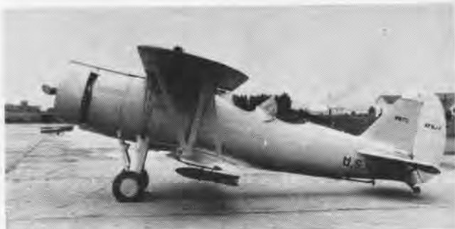
B/J XF2J-1 was 4320-lb., two-place prototype of 1932. With two-row 623-hp Wright, it made a top speed of 196 miles per hour.
