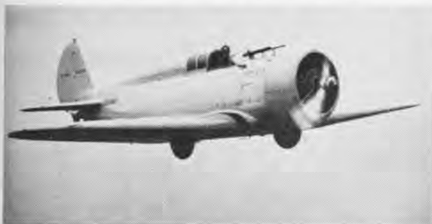
ONE OF FIRST Navy low-wing fighter prototypes was 1934 Boeing XF7B-1. Speed of 231 mph was reached with a 550-hp Wasp engine.
