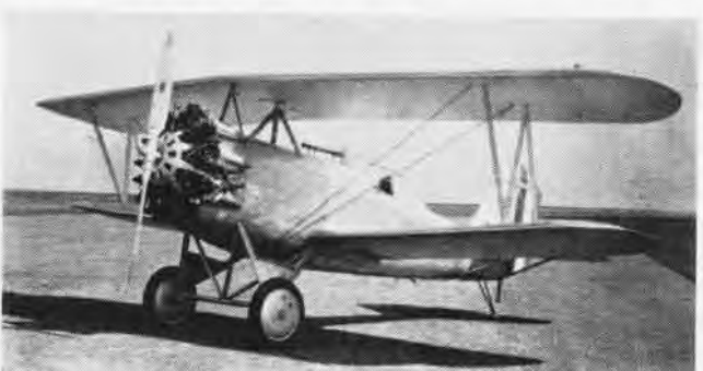
HALL-ALUMINUM XFH-1 was an experimental type in 1929. It weighed 2520 pounds, reached 153 mph with its 450 hp Wasp powerplant.
