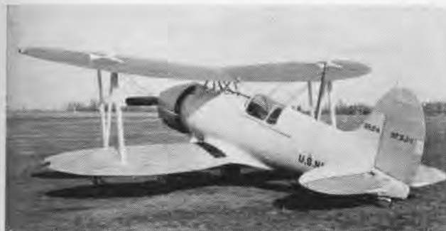
LAST B/J fighter prototype was "butterfly winged" XF3J-1 of 1933. With 625 hp twin-row Wright, its speed was 209 mph, weight, 4000 lbs.
