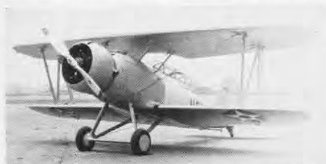
FIRST DOUGLAS fighter, 1933, was the XFD-1. Powered by a 700 hp Twin Wasp Jr., this two-place fighter made speed of 204 miles per hour.
