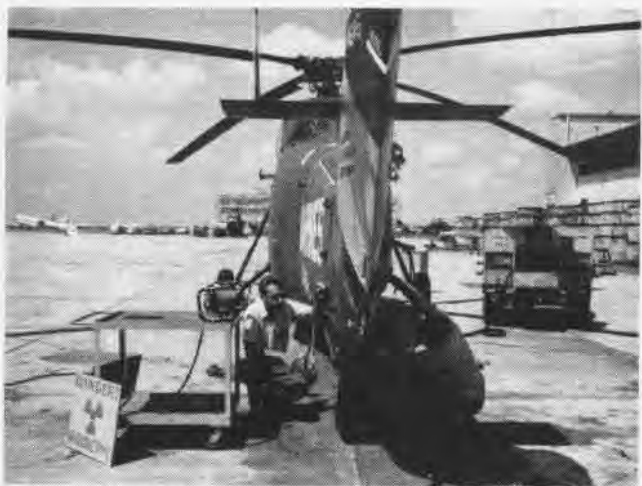
FILM IS MOUNTED for x-ray of belo tail pylon. When energized, camera on stand will project the x-rays through tail structure to film.
