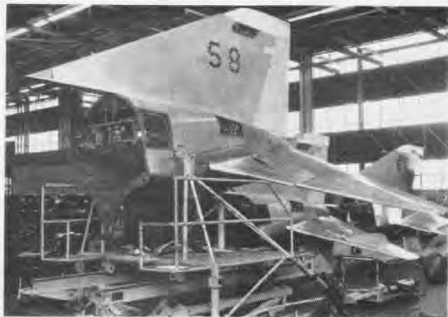
AFT SECTIONS are completed and ready for splicing. Fabrication begins with production of components, joined to form a subassembly.
