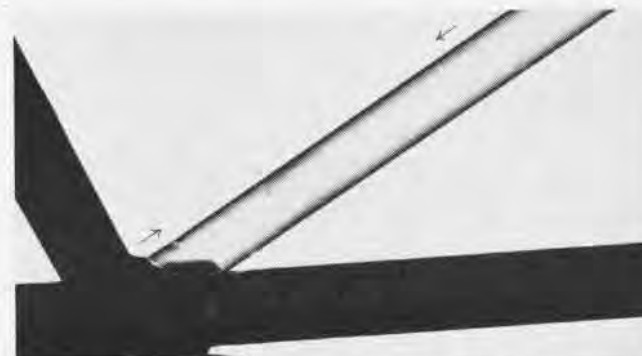
CORROSION INSIDE the tubular steel frame of HTL helicopter, while clearly revealed by x-ray, would be difficult to detect visually.
