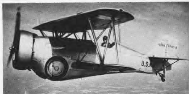
WITH RETRACTABLE gear, 645-hp Cyclone, XF11C-3 served as 1933 prototype for BF2C-1's, last of the Navy Hawk types: speed 216 mph.
