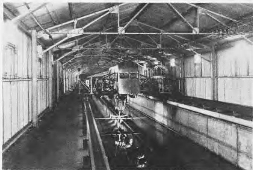
FLYING BOAT MODEL ATTACHED TO TOWING CARRIAGE IS TESTED IN SALT WATER TANK
