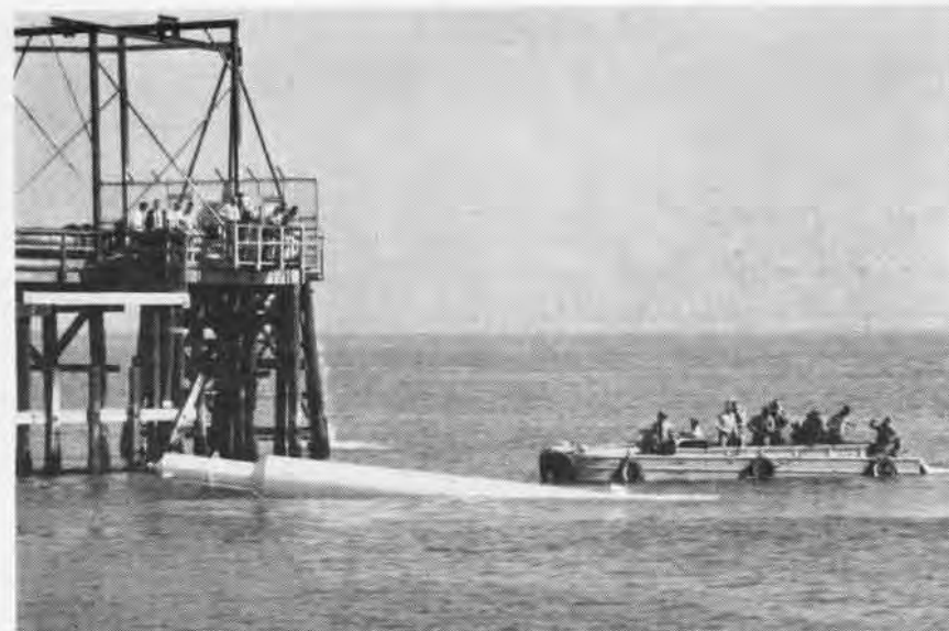
HYDRA DEMONSTRATED the Navy's safe and economical way to launch heavy space boosters from any part of the 72% of earth's surface which is water. In first view, the test vehicle is towed to launch site. Bottom (R), it floats like spar buoy, then rises—and soars away!
