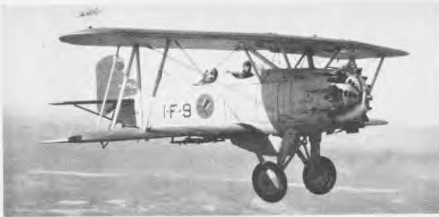
CURTISS F8C-4 Helldiver , as it is seen in TV movie of that name advanced dive bombing tactics. Weighing 3730 lbs., powered by 450-hp Wasp , it made top speed of 139 mph in 1929.
