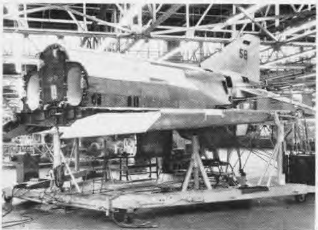
NEXT STEP is the splicing of the aft fuselage. Here three major assembly parts are shown in something that begins resembling an F4H.
