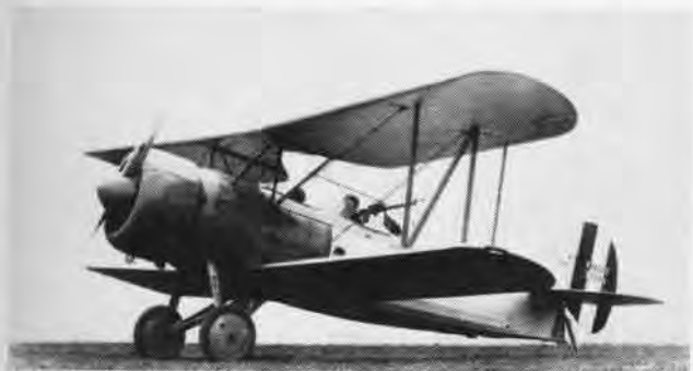
FEATURING a streamlined cowling around its Wasp engine, the two-place XF2U-1 of 1928 weighed 3890 lbs. and had a speed of 146 mph.
