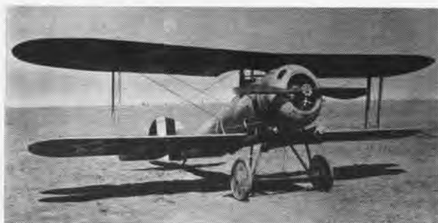
WW I FRENCH fighters, such as the 1625 lb, 122 mph Nieuport 28C-1 powered by a 168 hp Gnome rotary, were used back in early Twenties.
