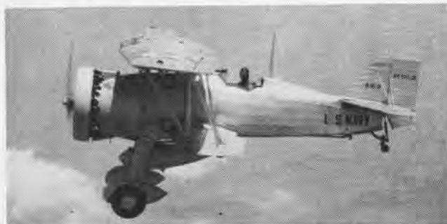
CURTISS XF11C-2 was 1932 prototype of F11C-2, redesignated BFC-2. With 600-hp Cyclone, this 4080-lb. Hawk had 192 mph top speed.
