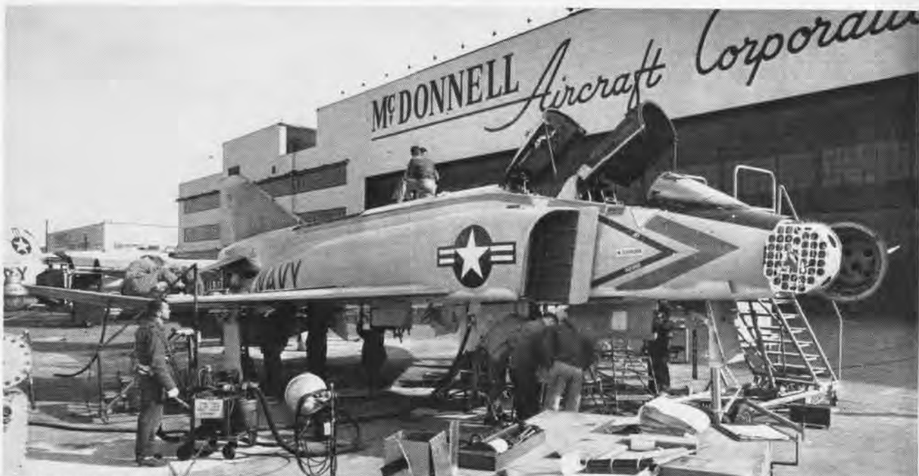
MCDONNELL'S FLIGHT Test Department conducts a thorough "shaking down" of the aircraft's systems. Check-out of electronic equipment
