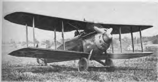
THOMAS-MORSE MB-3 obtained under Army contract in 1921 for Marines, reached 154 mph with 320 hp Wright-Hisso, weighed 1818 lbs.
