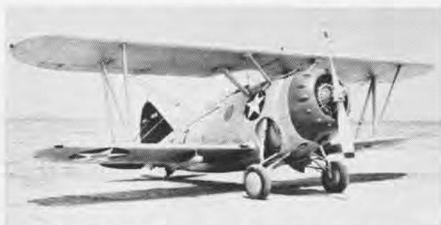
SHOWN WITH 1940 "Neutrality Star," F3F-1's were first delivered in 1936; weighed 4150 lbs., had same engine, speed as F2F-1.
