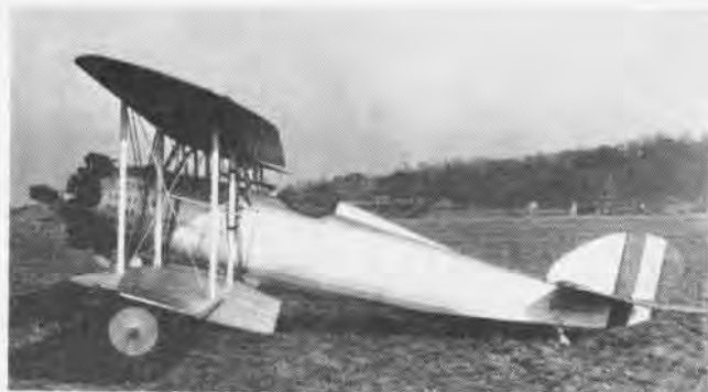
INTERIM FIGHTER was 1926 Vought FU-1, using 220-hp Whirlwind. It was designed from Vought VO series and had top speed of 124 mph.
