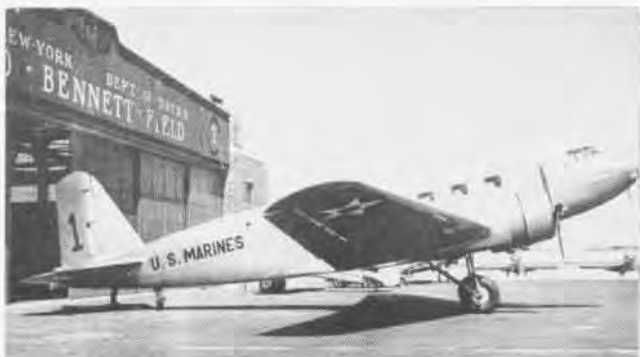
FIRST DOUGLAS transport to enter wide airline use was the DC-2. Both Navy and Marine Corps flew them as R2D-1's with Wright Cyclones.
