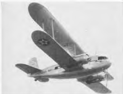
MARINES USED Cyclone powered Curtiss Condor biplane transports as R4C-1's in mid-30's.
