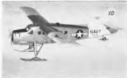
DEEP FREEZE service was reason for purchase of UC-1 Otters built by de Havilland, Canada.
