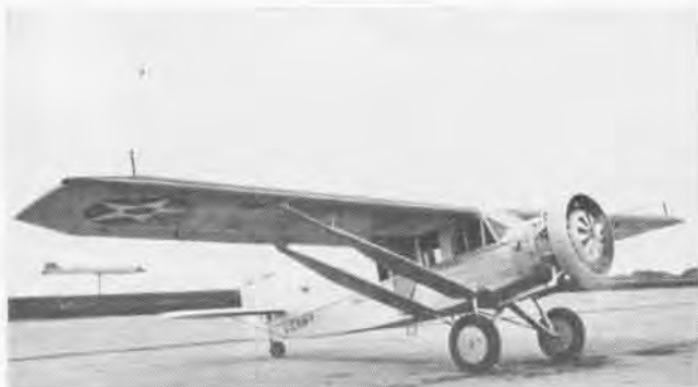
FIRST OF THREE Wasp-powered Bellanca's purchased as RE series was the XRE-1. It served as a radio test airplane at NAS Anacostia.
