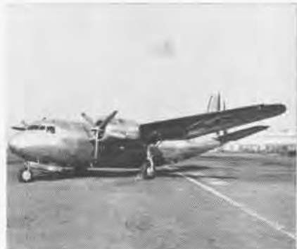
DOUGLAS DC-5 high-wing transport served Navy as R3D-1, Marines as R3D-2 (shown).
