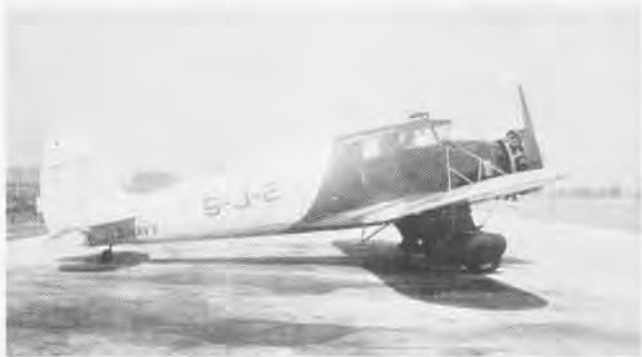
KINNER ENVOY , an early low-wing commercial model, was tested; three purchased as XRK-1's. They were extensively modified during service.
