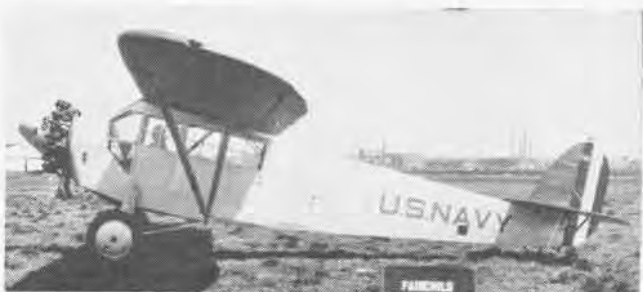
POPULAR COMMERCIAL design of late Twenties was Fairchild 71. Whirlwind-powered Navy XJQ-1 operated on wheels or twin-float gear.
