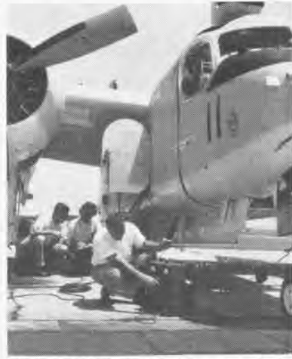
FINAL ELECTRONICS test determines whether S2F is ready for another operational tour.
