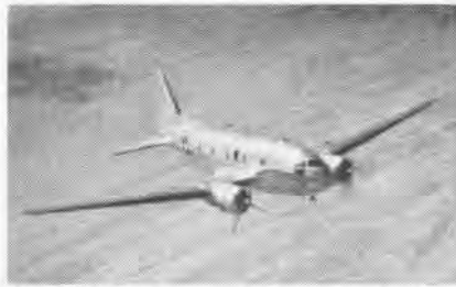
MARINE CORPS used AAF Curtiss C-46 as RVC-1. One engine was feathered for training.
