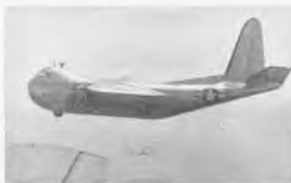
STAINLESS STEEL construction was feature of WW II Budd RB-1 Conestoga cargo plane.
