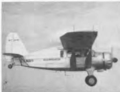
SINGLE NAVY JE-1 light utility transport of 1938 was improved Bellanca commercial type.
