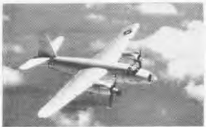
MARTIN MARAUDERS , AAF's WW II B-26 series, were Navy's JM-1 target-towing planes.
