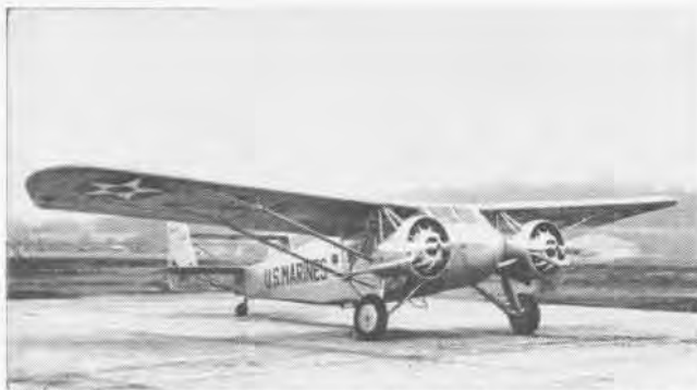
ONLY ONE Curtiss Kingbird was purchased. The twin-engine RC-1 served with Marines at Quantico and San Diego from 1931 to 1936.
