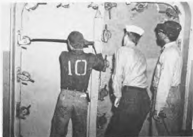
IN MATERIAL CONDITION 'ZEBRA,' MEN SECURE WATERTIGHT DOOR
