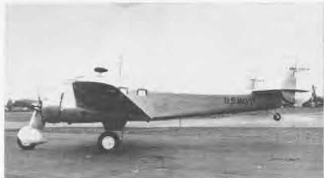
SMALLER LOCKHEED model 12's were used by Navy as JO series. XJO-3 with tricycle gear was experimented with as a possible carrier type.
