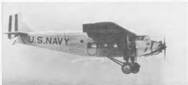
FORD TRI-MOTOR , purchased as XJR-1 in 1927, was Navy's first transport airplane. Other JRs, redesignated RRs, were bought later.
