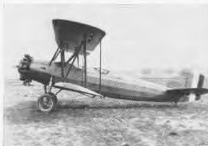
KEYSTONE NK-1 convertible trainers were heavier and powered by Wright Whirlwind.
