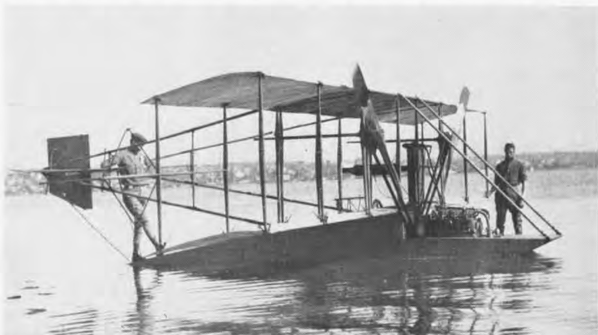
CALLAN INSPECTS CURTISS FLYING BOAT AT SAN DIEGO IN 1912, A TWO-PROPELLER TRACTOR TYPE WHICH FAILED
