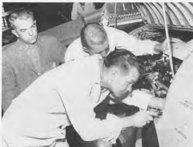
months 70 students completed courses ranging from two to five weeks. The pattern will be followed in factory maintenance training for the F4H, A3J, HSS-2 and other new models. Left, students bench check autopilot amplifier, right, work on electrical system of the F8U-2N.
