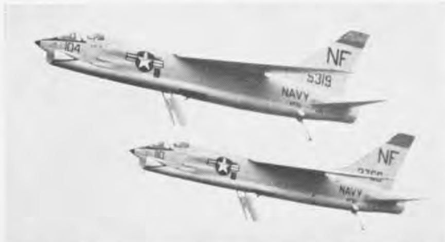
THIS UNUSUAL VIEW of F8U Crusader with speed brakes popped was made possible by pilots of Fighter Squadron 51. The lead aircraft is flown by Lt. D. L. Upton, and his wingman is Lt. T. R. McCool. As we go to press, VF-51 is deployed in the Western Pacific aboard the Ticonderoga .
