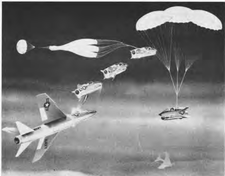
CHANCE VOUGHT CAPSULE WAS DESIGNED TO GIVE OPTIMUM SAFETY IN EMERGENCY
