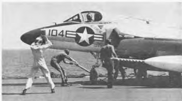
GETTING ANOTHER one ready, catapult crew member straightens nose wheel on catapult. Unbalanced plane may make fish tail take-off.
