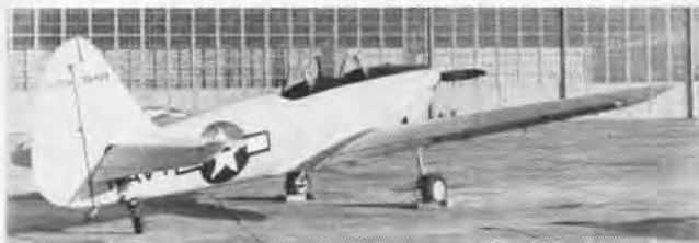
TIMM N2T-1's used in training had uncoupled radial engines. Prototype XN2T-2 with six-cylinder opposed, air-cooled Lycoming was tested.
