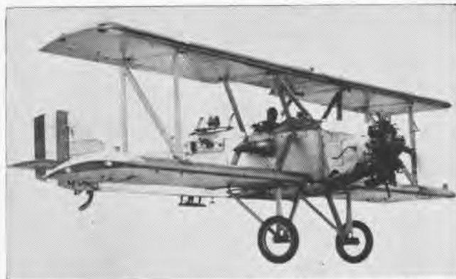
SELECTED FOR production, Boeing NB-1 could serve as a seaplane primary trainer or as gunnery trainer (shown). NB-2 had Wright-Hisso.
