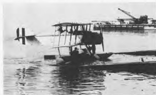
NAVAL AIRCRAFT FACTORY prototypes were the TG series of the early Twenties. They used different in-line engines in the models built.
