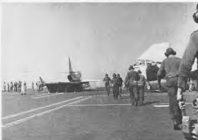
JET BLAST deflector screen up, A4D on catapult is hooked up, turned up and ready to go. Flight deck crew goes about assigned tasks.
