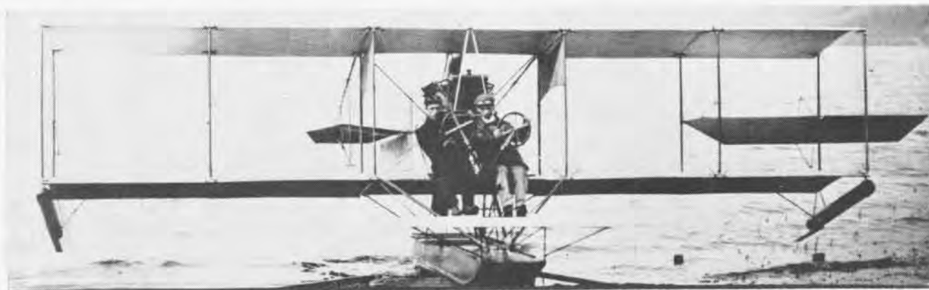
ACTUALLY TIED TO THEIR TASKS, AIRMEN WERE CONNECTED TO AILERONS BY CORDS: LEANED LEFT OR RIGHT TO BANK CRAFT
