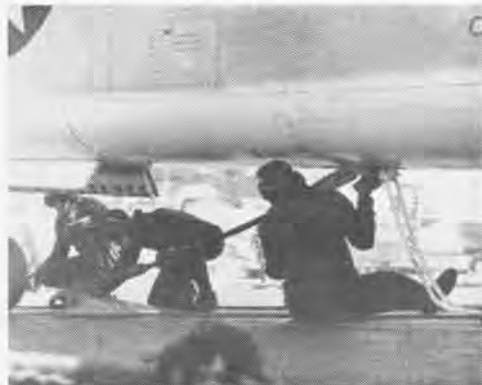
STRONG, CAPABLE, quick, these hands make the bridle connection between A4D and shuttle cock of cat.
