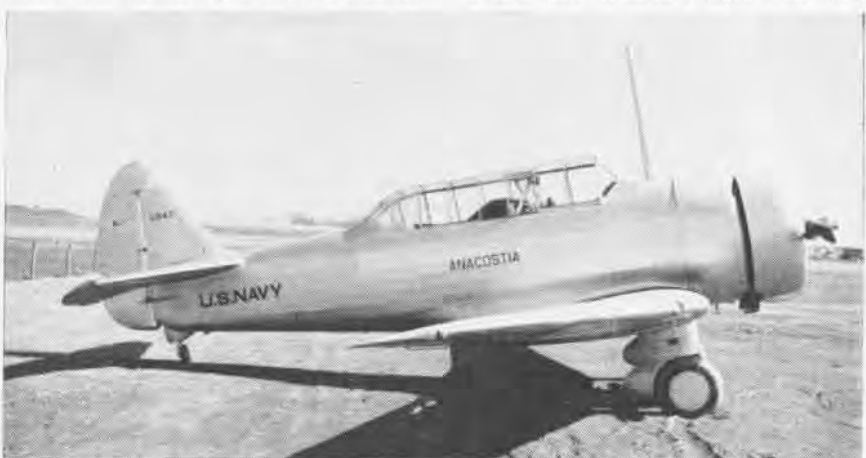
FIRST LOW-WING Navy trainers were 1933 North American NJ-1's. These were similar to the Army BT-9B basic trainer with fixed landing gear. Design was basis for later NAA airplanes.
