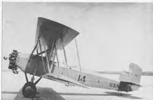
LIKE ALMOST all of the Navy trainer types of the late Nineteen-Twenties, the Curtiss N2C-1 was powered by a Wright Whirlwind engine.
