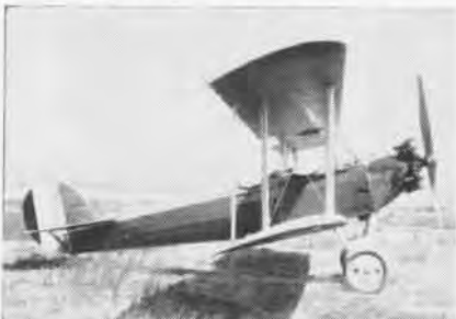
UNUSUAL ENGINE , the Caminez four-cylinder radial, was powerplant in XN2B-1 prototype.
