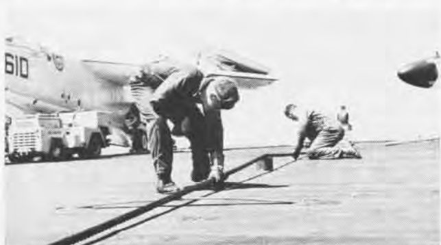
PREPARING FOR recovery, two important operations are accomplished by these hands: greasing the cable and checking for loose strands.
