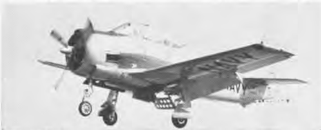
EQUIPPED FOR carrier operation, the North American T-28C was modified from the land-based T-28B. Both have 1425-hp Wright Cyclones.
