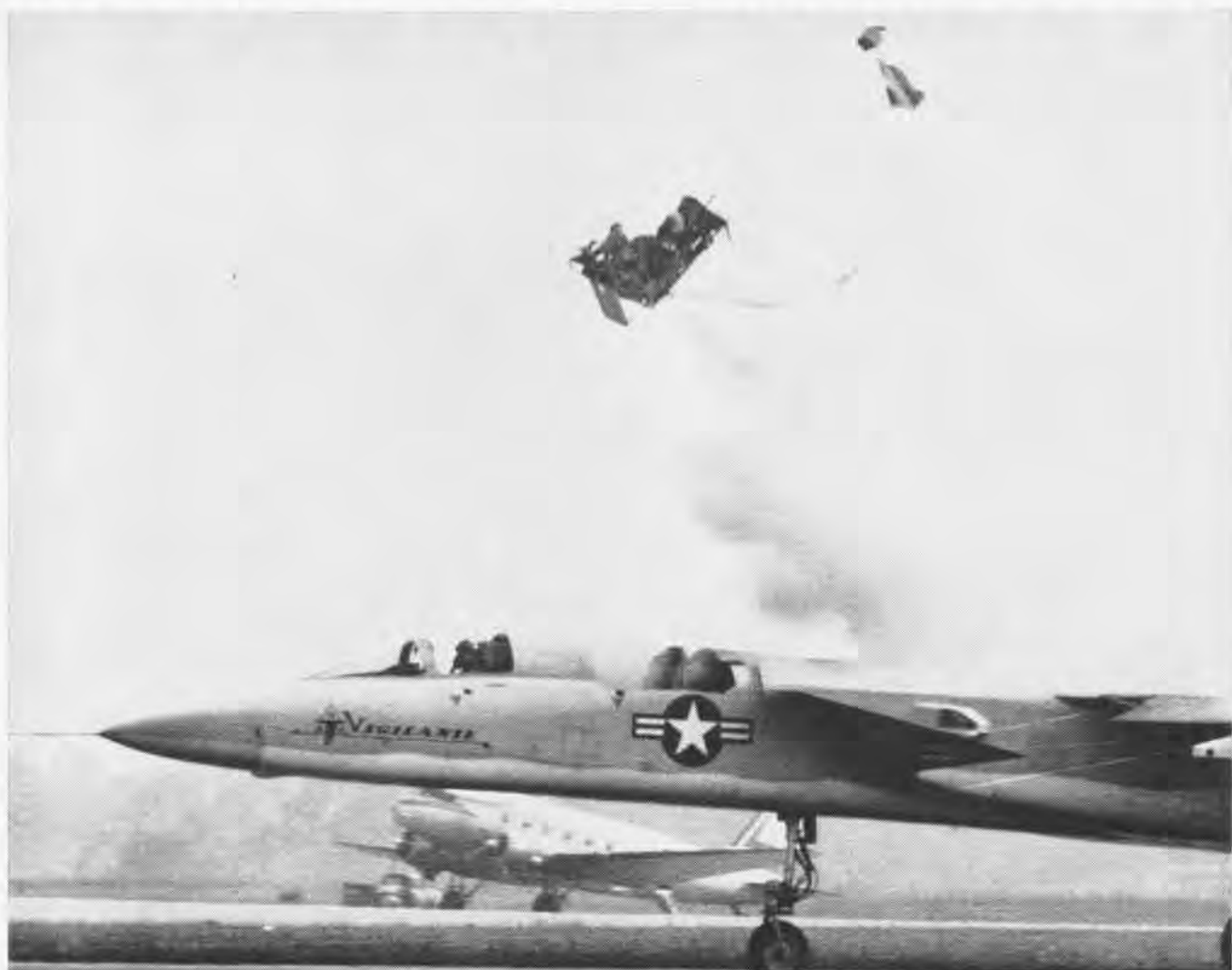
ROCKET PILOT ESCAPE SYSTEM PROPELS DUMMY CLEAR OF NORTH AMERICAN A3J. SIMILAR EQUIPMENT IS USED IN THE T2J BUCKEYE
