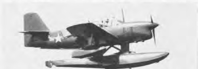
UNUSUAL TRAINER prototypes were Edo XTE-1 seaplane of late '40's. Powered by a Ranger engine, TE was to train capital ship scout pilots.
