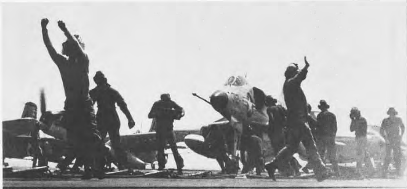
LAUNCHING AIRCRAFT is an important part of the vital mission of today's carrier. Preparing for launch, taxi man (left) hand signals "Hold those brakes" while catapult crew fastens plane on catapult. Man on right signals for the attention of the next plane up.
