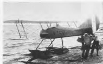
WW I SINGLE-SEAT "scout" type trainers included Thomas-Morse S-5 with rotary engine.
