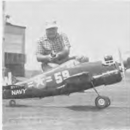
AN F6F MODEL ready for flight circuit, is powered by a .59-hp engine, hits 80 mph.
