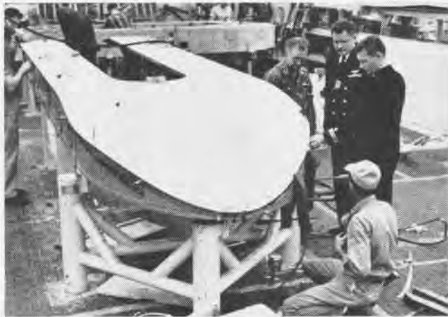
THE TRICYCLE SKI-WHEEL installation of the C-130BL Hercules is inspected by students at the factory. Plane lands on either skis or wheels.
