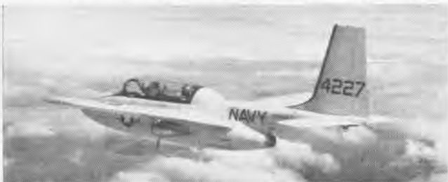
PRIMARY JET training was evaluated in program using Temco TT-1 Pin-tos, a small number of which were purchased by Navy for this purpose.
