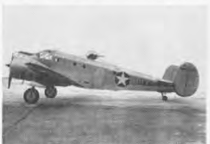
FIRST BEECH SNB-1's were Army's AT-11 bomber crew trainers; turret later eliminated.
