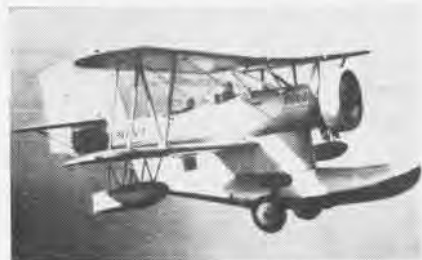
SUCCESS of Loening O1 series led to XO2L-2, which was all metal except for wing covering.
