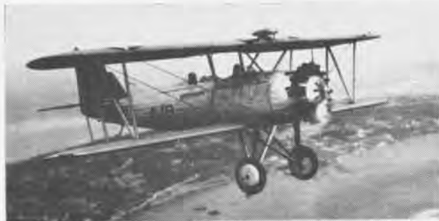
VOUGHT O2U Corsair was first airplane designed to use Pratt & Whitney Wasp engine; a long series of convertible Corsairs followed.
