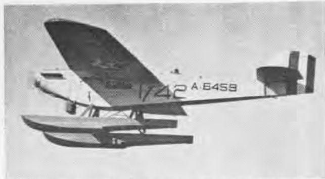
MARTIN MO-1 monoplane of 1925 had all-metal internal structure, cantilever wing. Speed as seaplane was 102 mph with 550 hp. D-12.
