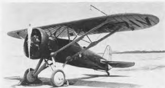
ALL-METAL CONSTRUCTION was feature of Boeing's 1935 Wasp-powered XF5B-1 monoplaner. Later F4B-3 and -4 used fuselage and tail design.
