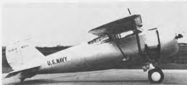
MONOPLANE OR BIPLANE wings could be fitted to 1933 Curtiss XF13C prototype. Final XF13C-3 monoplaner shown had modified vertical tail.
