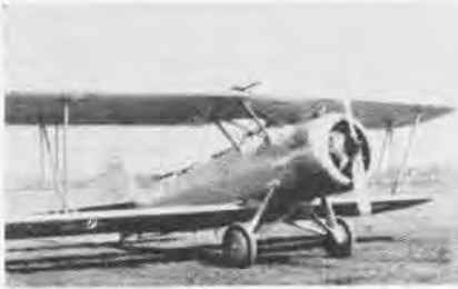
METAL CONSTRUCTION was also feature of Keystone XOK-1, with streamline cowling.
