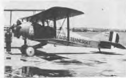
FIRST VO design with lighter engine was Vought VO-1 with 200-hp air-cooled engine.
