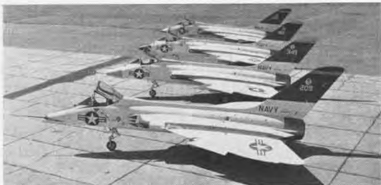
FIRST FOUR SKYLANCERS were in flight test when Douglas F5D-1 program was terminated. Based on F4D with thinner wings, supersonic F5D carried Sparrow II's.
