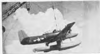
CURTISS SC-1 Seabawk was large, fast, catapult type, entered service in late WW II.
