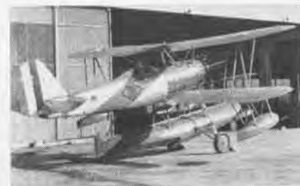
AMPHIBIOUS FLOAT installed on O3U-1 Corsair; O3U's also flew with floats or wheels.
