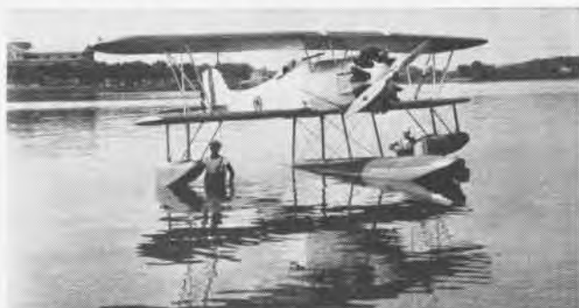
EBERHART COMANCHE was entered in 1927 "Battleship Fighter" competition. All of the competitors flew with wheels as well as float gear.
