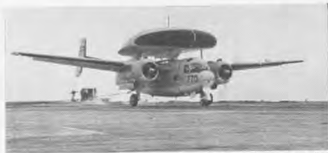
AIRBORNE EARLY warning versions of standard attack aircraft led to Grumman WF-2, based on S2F/TF. Turboprop W2F-1 will follow.
