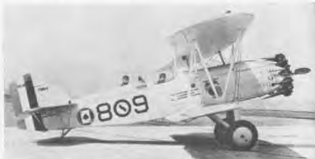
ORIGINALLY DESIGNATED as fighters were Curtiss OC observation types for Marines. OC-2 was based on Army attack plane, had Wasp engine.
