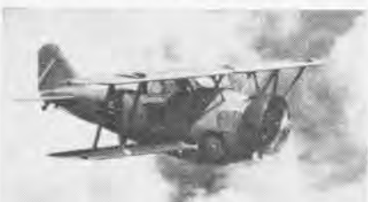
GRUMMAN SF-1 was carrier scout version of FE-1 fighter, the first Grumman airplane.
