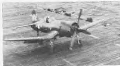
PROP AND JET fighters have been converted as photoplanes, including the Vought F4U-5P.
