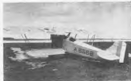
HUFF DALAND HO-1's modified from HN trainers, were early light observation types.
