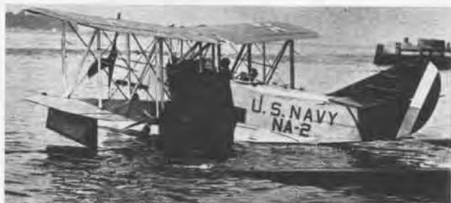
EARLY VERSION of successful Loening OL series was the OL-2, used on early Byrd Arctic trip. A 400-hp Liberty gave top speed of 121 mph.
