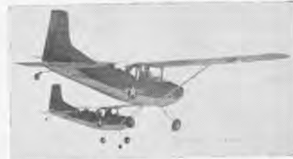
MARINE VMO squadrons currently fly Cessna OE-2's, the improved versions of OE-1/L-19.
