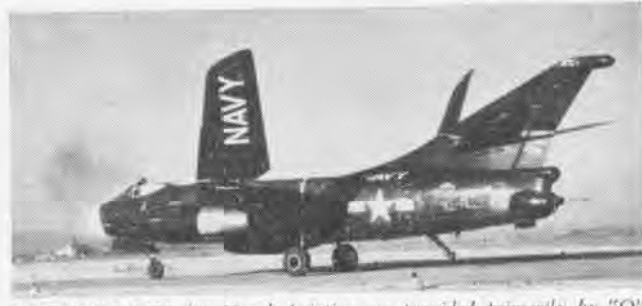
ELECTRONIC EARS for Naval Aviation are provided primarily by "Q" version of various designs. The A3D-1Q shown folding its wings.
