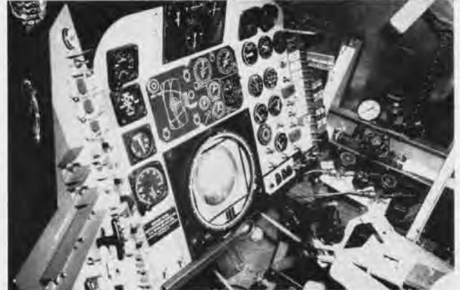
JOHNSVILLE SIMULATOR panel was used to give familiarization rides to astronauts. Glenn's special task was cockpit design and layout.
