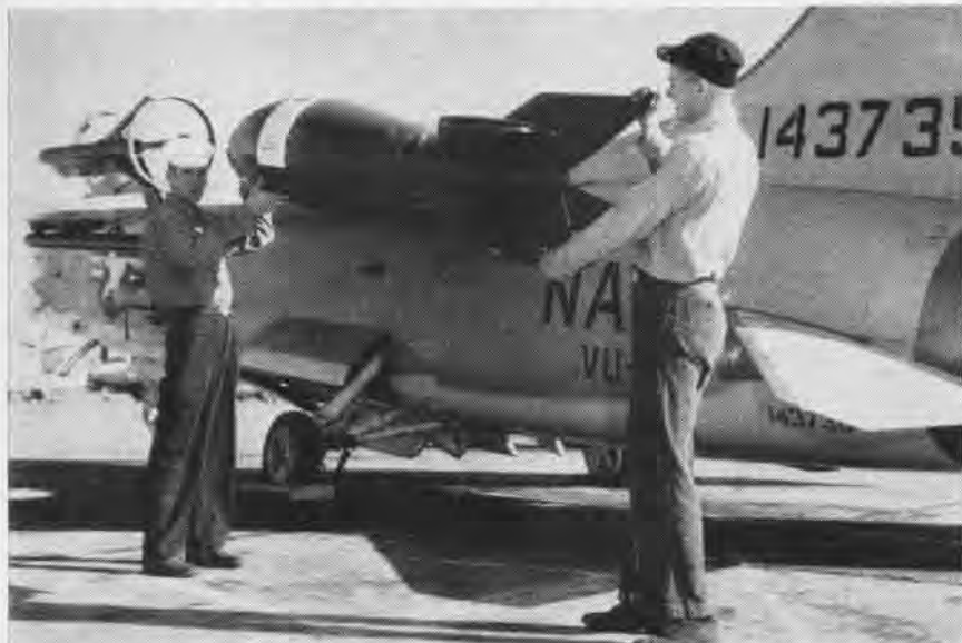
A VU-7 AERO-36 TARGET IS PLACED IN 'BASKET' MOUNTED ON WING OF A CRUSADER
