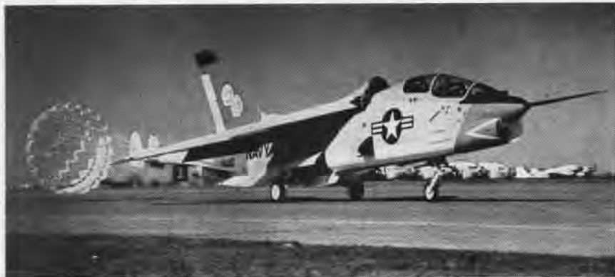
TWO-PLACE F8U-1T STREAMS ITS DROGUE CHUTE TO SLOW ROLL-OUT ON MAIDEN FLIGHT
