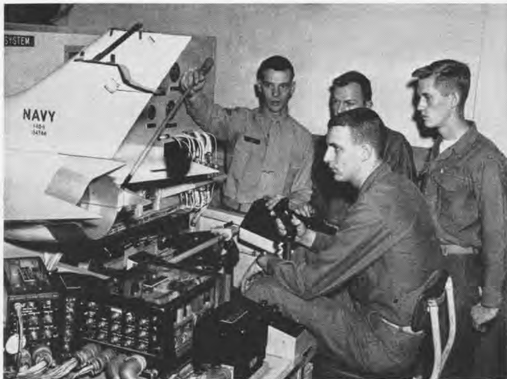
THE F4D-1 SKYRAY auto control panel enables the students to see, hear, and feel how a system works. A training panel is a prime tool of the Naval Air Maintenance Training Group as it "takes the school to the students."
