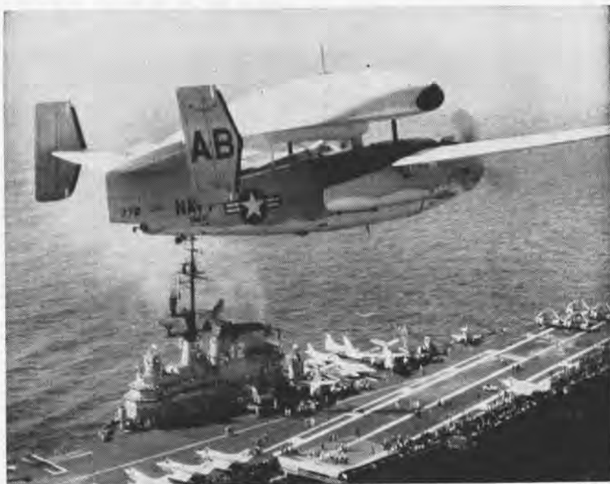
POTENT COMBINATION of APS-82 radar and "Mr. C," the NAO(C) controller, enables "Willy Fudd," shown passing Roosevelt, to give Fleet an early warning edge for effective air defense.
