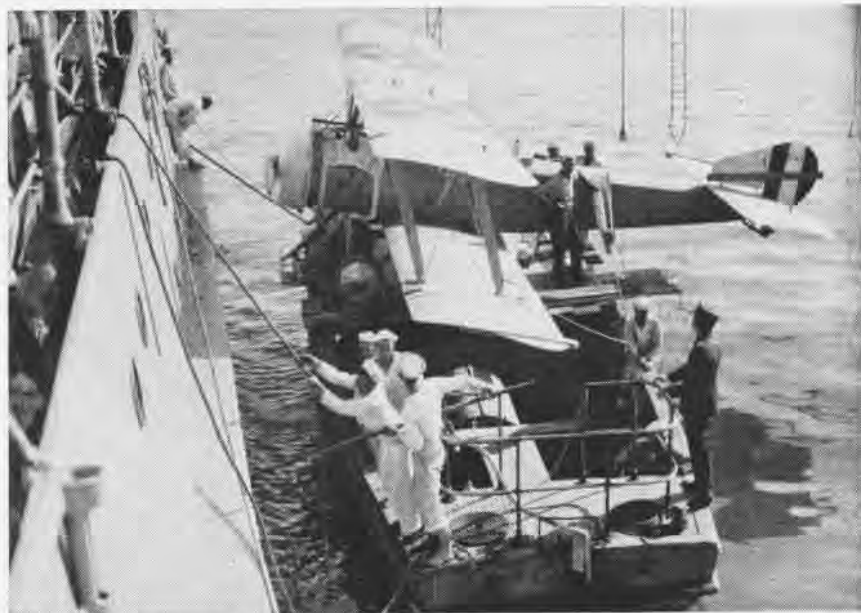
SOPWITH 1½ STRUTTERS, equipped with hydrovanes in the event of a forced landing in the water, were used by the air detachments in exercises with the Fleet immediately after World War I.
