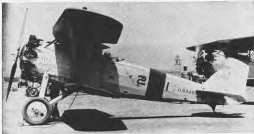
TYPICAL OF THE EARLY air-cooled engine carrier fighter, scout, and dive bomber types which flew from the Lex and Sara in Fleet Problem IX were the Boeing F2B-1's of Bomber Squadron 2.
