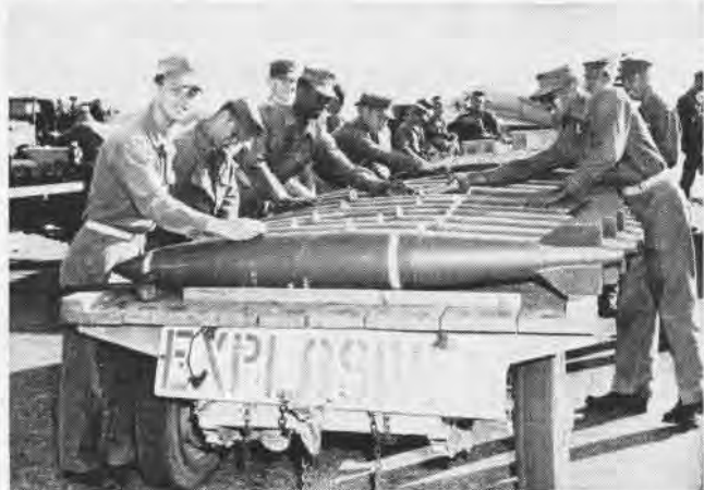
HERE MEN of the ordnance section carefully prepare a load of 250-lb. bombs which are to be mounted on the squadron's sleek A4D Skyhawks.
