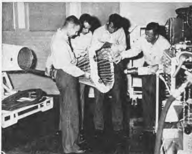
JOHN P. CONNOR , ADI, of the A4D detachment at NAS Jacksonville demonstrates operation of the probe and drogue of the "buddy" refueler.
