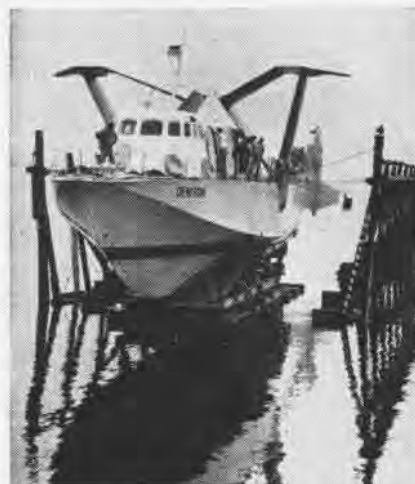
DENISON'S FOILS IN RETRACTED POSITION
