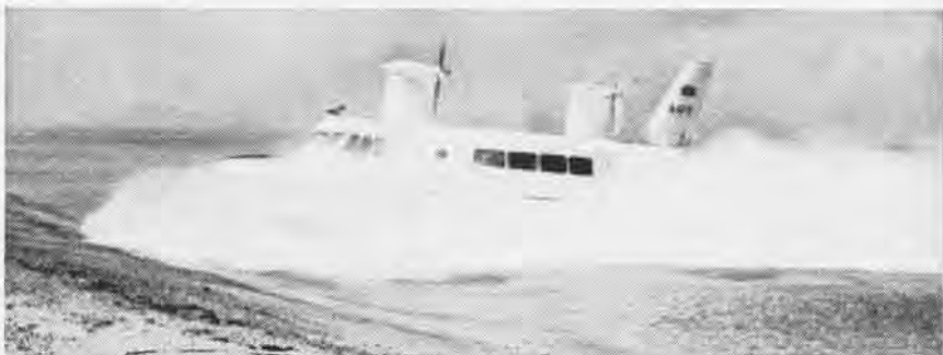
HALF SHIP, HALF AIRCRAFT , the British SR-2N hovercraft creates downwash as it commences trials in England. American observer, RAdm. R. K. James, BuShips, called the hovercraft ride "fantastic experience." Two fans push air downward, create air cushion between water and ship, topside engines provide forward speed. SR-2N speed is 60 mph, capacity is 68 passengers. American Craft, Bell "Hydroskimmer" is due to be introduced in mid-1963.
