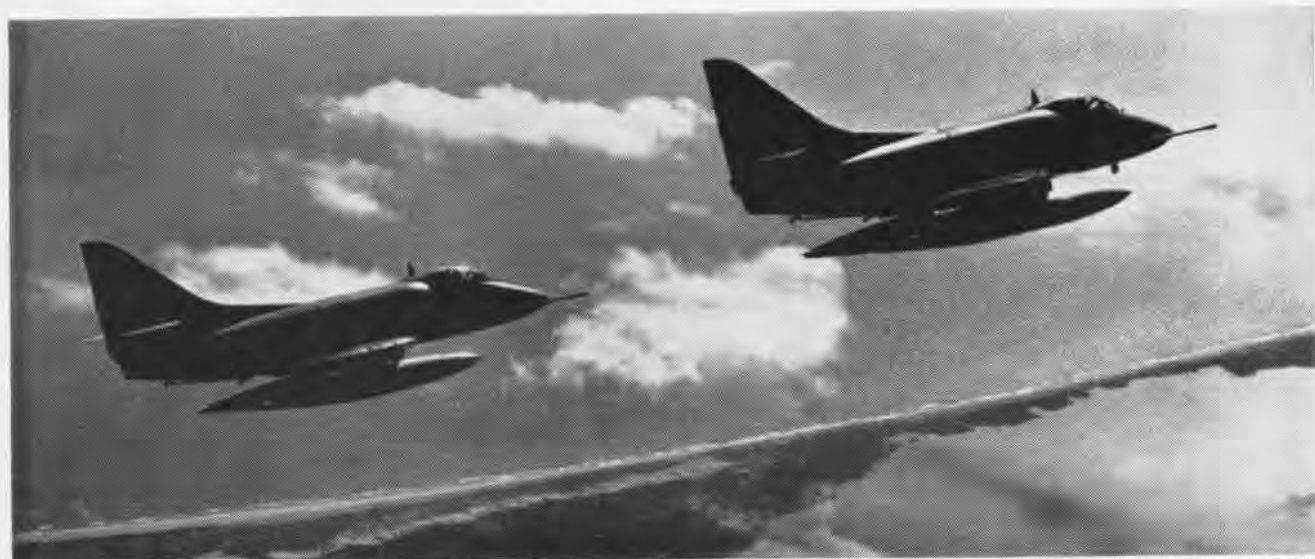
AIRPLANE NEEDING FUEL DROPS BEHIND THE TANKER IN ORDER TO CHECK MAIN STORE AND BE SURE THERE IS NO LEAKAGE
