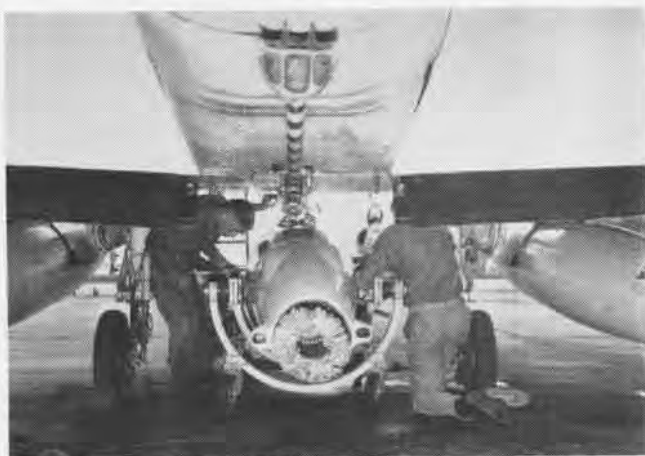
TANK IS THEN JACKED IN PLACE WITH HAND-POWERED WINCHES.
