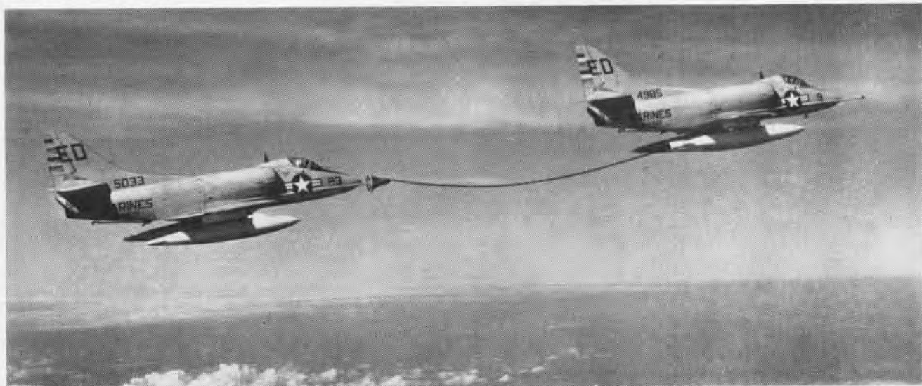
FOR PRACTICE TWO OR THREE DRY PLUG-INS ARE MADE IN ORDER TO TAKE NO CHANCES AND INSURE A GOOD, RELIABLE CONNECTION.
