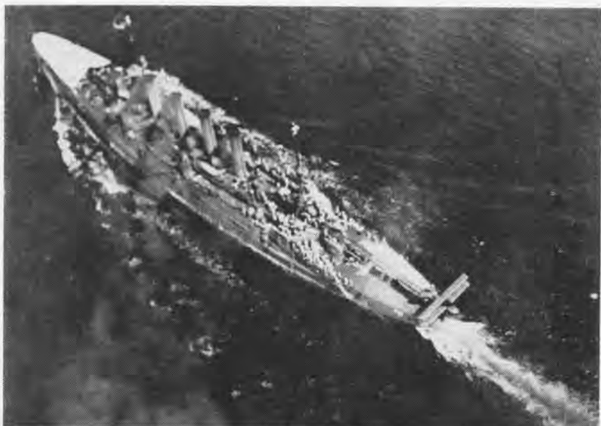
PLANE LAUNCHES from catapult on cruiser Huntington. After U.S. intervention in WW I, catapult was removed from all U.S. ships. Huntington spent war years in convoy escort duty.
