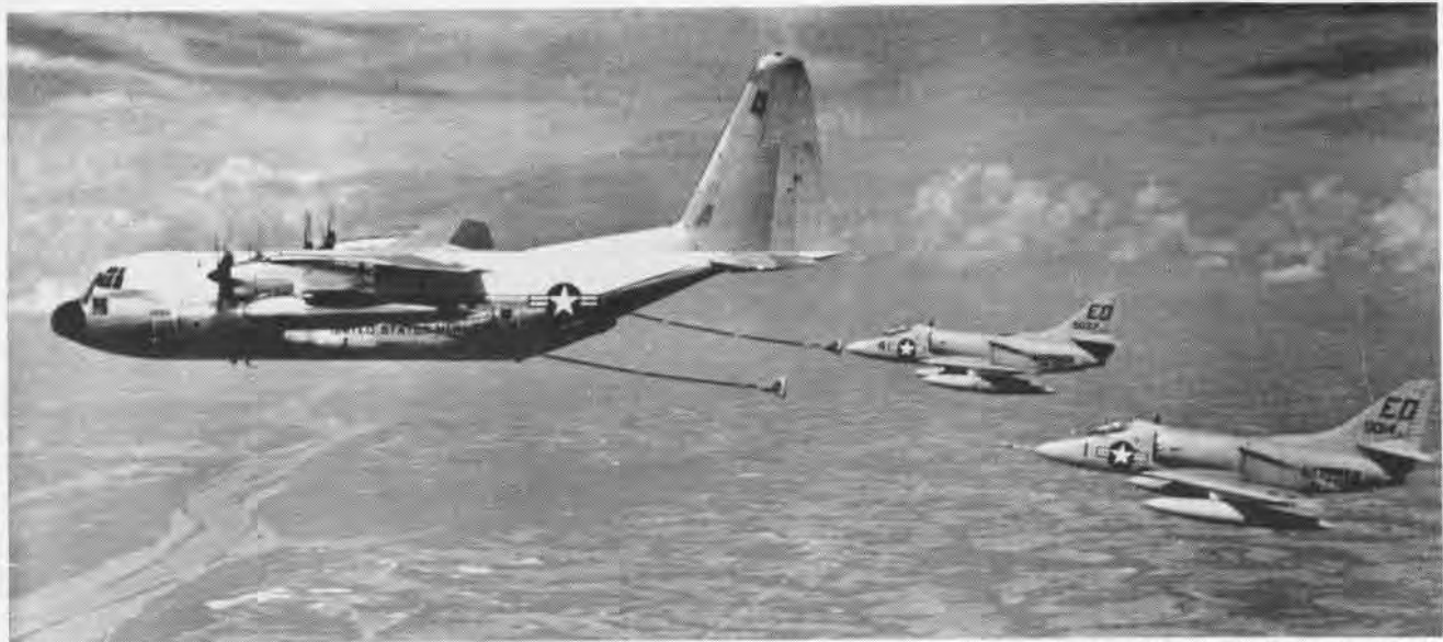
MARINE'S NEW TURBOPROP GV-1 Hercules refuels two A-1J attack jets. An aerial tanker of over 10,000-gallon capacity, the GV also has
