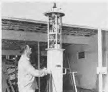
UNDERSEA SOUNDS broadcast by this "doctor" buoy are compared with test buoy signals.
