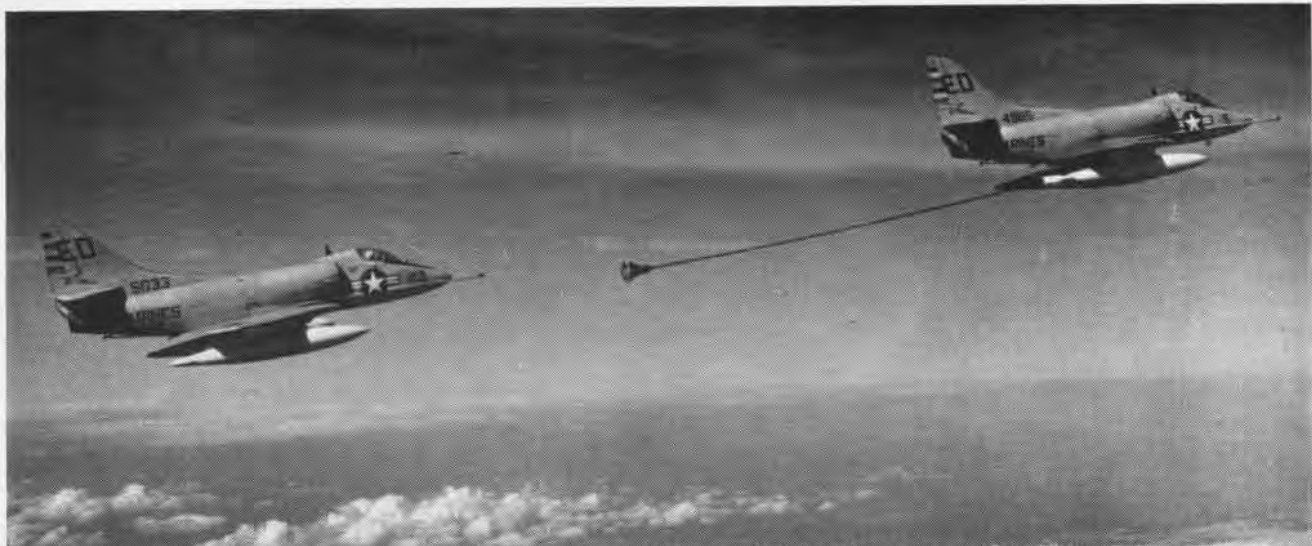
LINING UP WITH DROGUE, 'THIRSTY PLANE' GETS READY FOR MOMENT WHEN FUEL TRANSFER IS MADE AT 200 GALS. PER MINUTE
