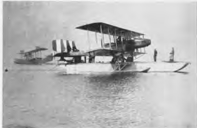
A MUSTIN SEA SLED holds a Caproni bomber in post-WW I tests at Hampton Roads. Sled was designed to add launching power to planes.
