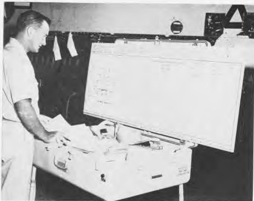
SEQUENCE CHART provides a pre-planned order for accomplishing the work on the cards and helps achieve smooth workflow where parts, people, and equipment needs are fully coordinated.
