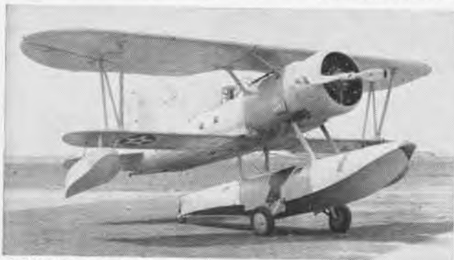
PROTOTYPES of three designs for observation amphibian types to replace the Vought Corsairs were built in 1934, including this X02D-1.
