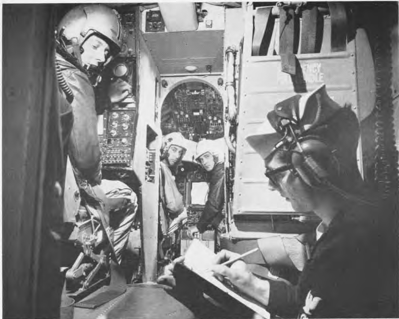
THE FREEZE IS ON. Training session in the 2F-66 weapon system trainer is "frozen" as crewmen await comments of an observer on their performance during simulated mission. This "stop-go" capability alone is said to increase advantage of trainer over actual aircraft 30 per cent.
