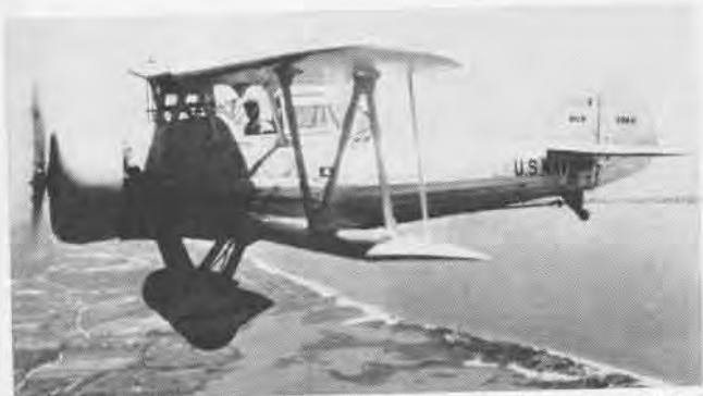
VOUGHT CORSAIR biplanes were built under many designations. XSU-4 was one of the last models. Like other SU's, it was a carrier scout.
