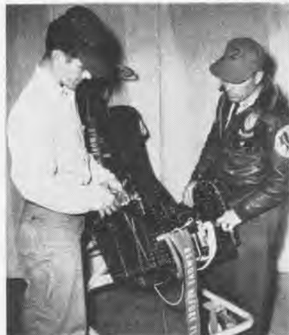
W.R. SMOOT, AMS2 of VF-124, imprints seal of quality on guillotine-firing mechanism.
