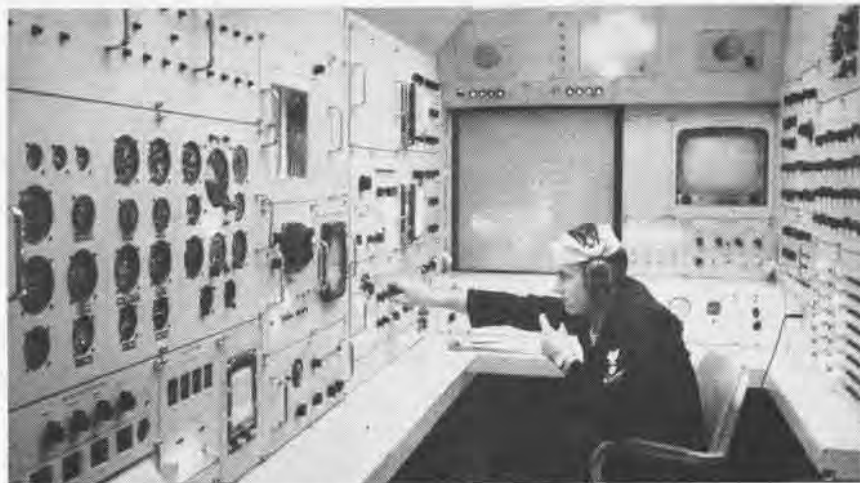
THERE'S TROUBLE ahead for the 2F-66 pilot as instructor injects "engine malfunction" into the problem. "Hen tracks" on screen are picture of simulated aircraft and "target"—a sub.
