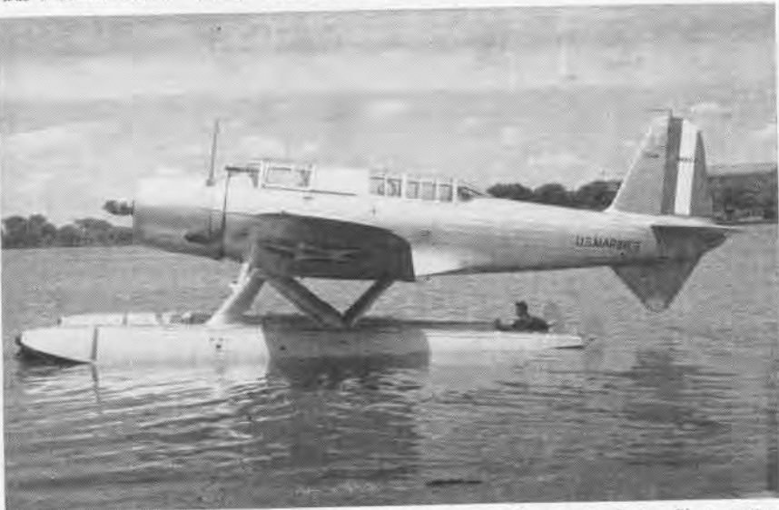
VOUGHT SB2U-3 was 1941 production carrier type, convertible to twin floats. Float versions of other contemporary carrier types were tested, but were not put into production.
