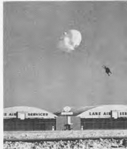
THESE GROUND-LEVEL TESTS OF THE ROCKET SEAT IN THE T2J BUCKEYEWERE PART OF NORTH AMERICAN AVIATION'S TEST PROGRAM
