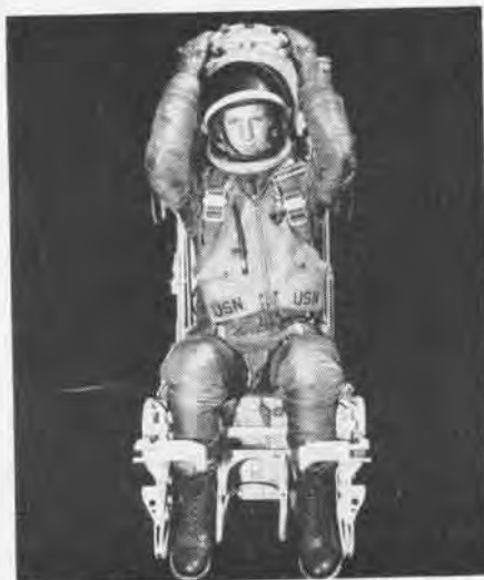
THIS A3J SEAT PACKAGES ESCAPEE FOR SUPERSONIC ROCKET RIDE. IT CAN BE TRIGGERED BY FACE CURTAIN OR ARM REST SQUEEZE GRIP
