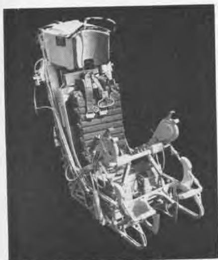
THIS A3J SEAT PACKAGES ESCAPEE FOR SUPERSONIC ROCKET RIDE. IT CAN BE TRIGGERED BY FACE CURTAIN OR ARM REST SQUEEZE GRIP
