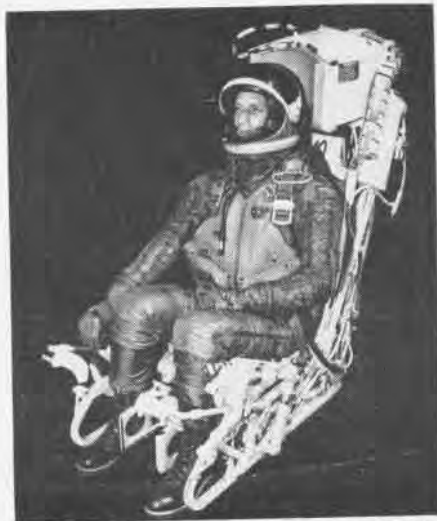
THIS A3J SEAT PACKAGES ESCAPEE FOR SUPERSONIC ROCKET RIDE. IT CAN BE TRIGGERED BY FACE CURTAIN OR ARM REST SQUEEZE GRIP
