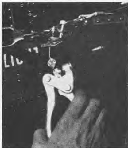
DIES IN JAWS of hand press inscribe seal with "mark" of man certifying work quality.
