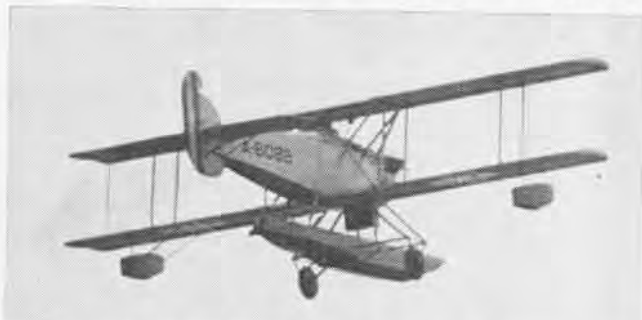
DAYTON-WRIGHT WA-1 prototype was one of first Navy amphibians. This observation type was equipped with a 325-hp Wright Hisso.
