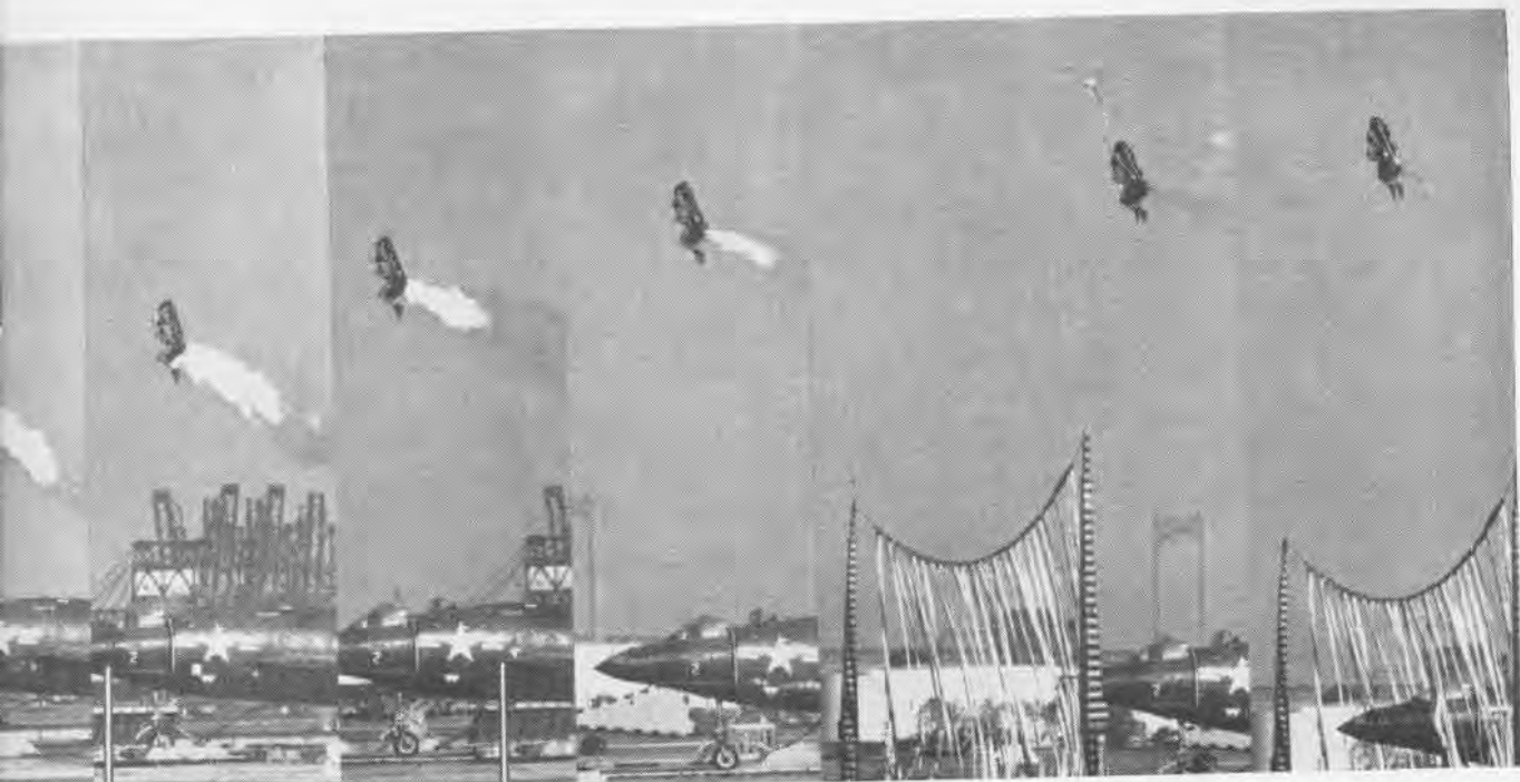
SH RIDE—118 FT. APOGEE—IN RECENT TESTS AT NAVAL AIR MATERIAL CENTER IN PHILADELPHIA
