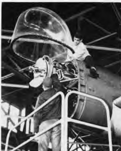
SEARCHLIGHT OPERATION is checked by crewmen to keep P2V ready for ASW missions.
