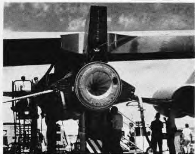
REAR VIEW SHOWS SINGLE-CHAMBER 57,000-LB.-THRUST ENGINE
