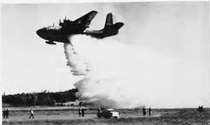
THE GIANT MARTIN MARS flying boat, retired by the Navy in 1956 after more than 13 years of service, has found a new berth deep in the Canadian forests of British Columbia. It is serving as a forest water bomber for six leading wood products firms. It has been modified to skim along the surface of a lake and scoop into special tanks up to 8160 gallons of water in 15 seconds. Flown over a fire area, the water is jettisoned in 3½ seconds.
