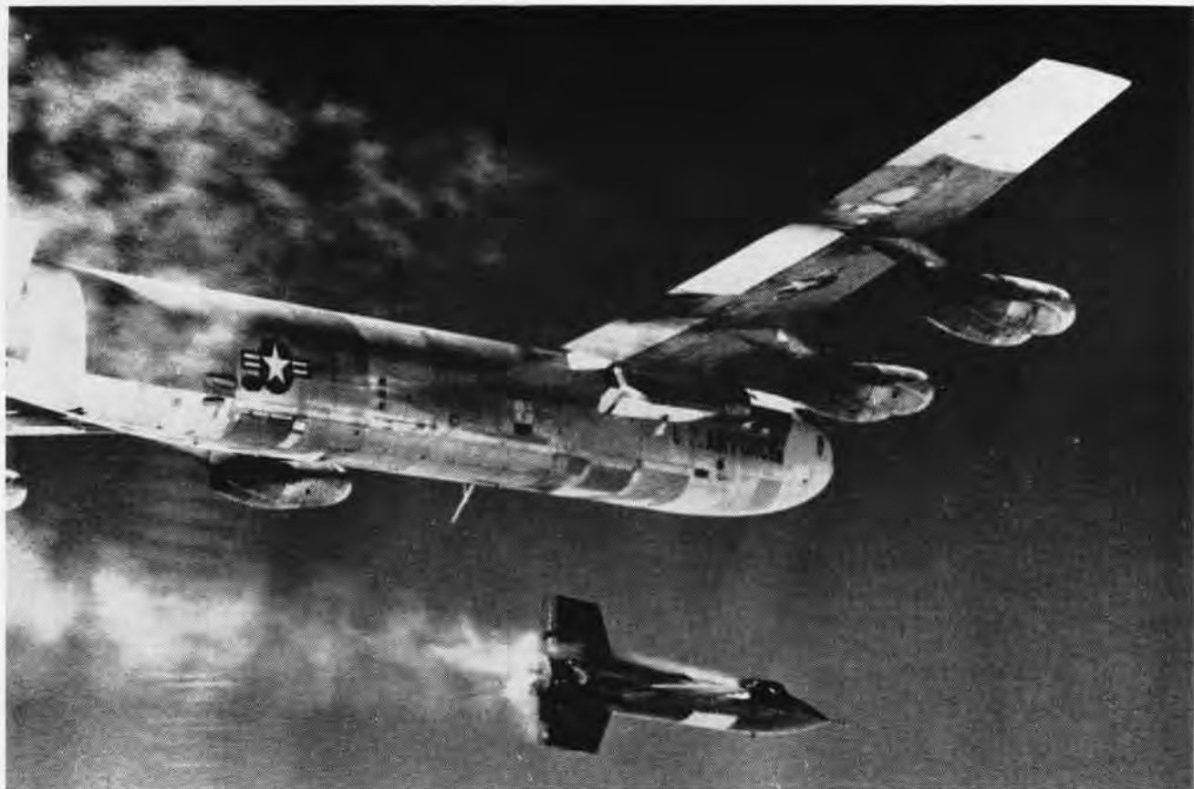
DROPPED FROM THE WING OF A B-52, THE NORTH AMERICAN X-15 USES ITS OWN ROCKET POWER TO SPEEDS IN EXCESS OF 4000 MPH
