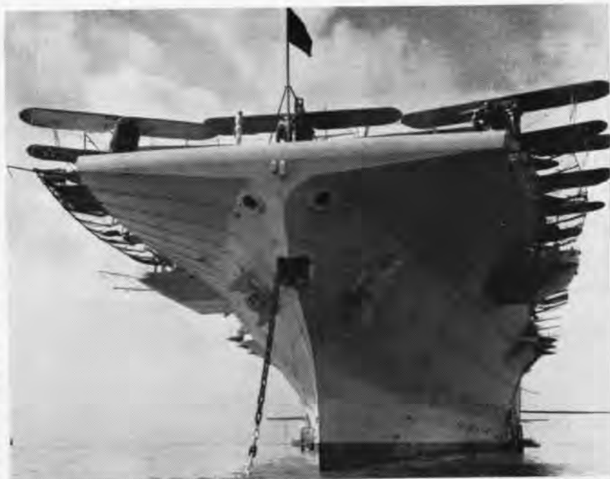
GRUMMAN FIGHTERS are parked on deck of USS Lexington . View emphasizes battle cruiser hull design. Weather bow, appearing in 1933-34, was standard in post-WW II modernization.
