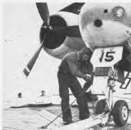
MIDGE ARCHIE CLEMENS, University of Illinois, ties nose gear of S2F to the deck.
