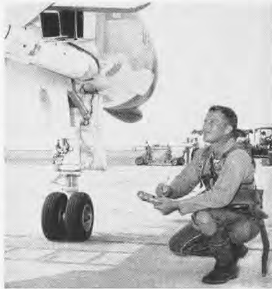
SERIAL NUMBERS, type missiles and station on plane are entered in Missile Identification Section of AAMREP card.
