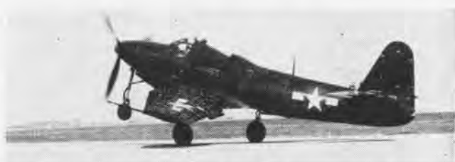
TWO NAVY L-39's were converted by Bell from Army Air Force P-63 Kingcobra fighters to study low speed characteristics of swept wings.
