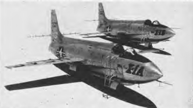
THE X SERIES of research aircraft started with the Bell X-1's. Rocket-powered X-1 was the first airplane to exceed the speed of sound.
