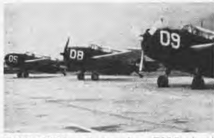
ONCE FILLED with torpedoes, TBM's bomb bay now is "armed" with tanks full of slurry.
