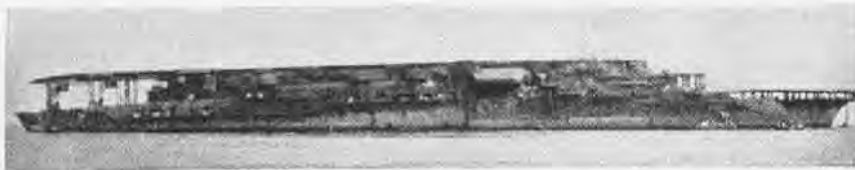
UNDER THE WASHINGTON Naval Treaty, Japan converted a battle cruiser to aircraft carrier characteristics. In 1928, that country's 2nd carrier was completed and named Akagi , after a mountain.
