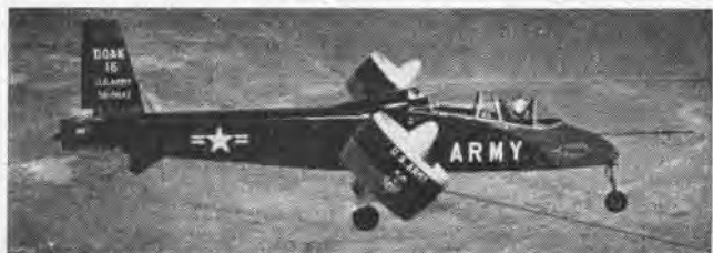
DOAK VZ-4 was successful VTOL research vehicle using tilting ducted fans at wing tips. QNR played major role in VTOL research program.
