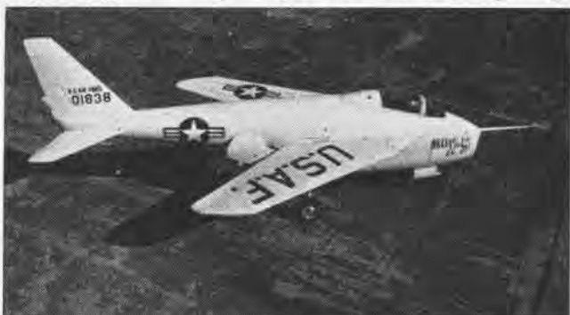
VARIABLE SWEEP wing tests were the principal design purpose of the Bell X-5, a jet-propelled research airplane type of the early Fifties.
