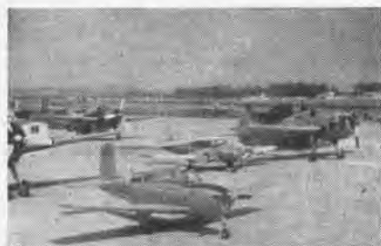
LINE-UP of firefighting aircraft includes the T-34 Mentor, foreground, and fleet of TBM's.
