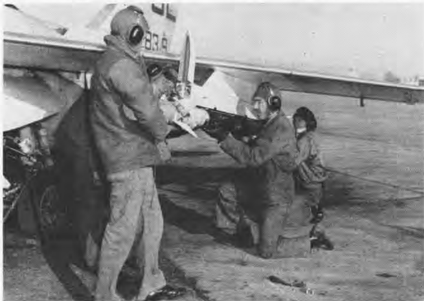
VT-26 ORDNANCEMEN attach the lethal Sidewinder air-to-air missile to an F11F Tiger before an exercise. The Beeville, Texas, outfit has an important role in the Air Defense Command.
