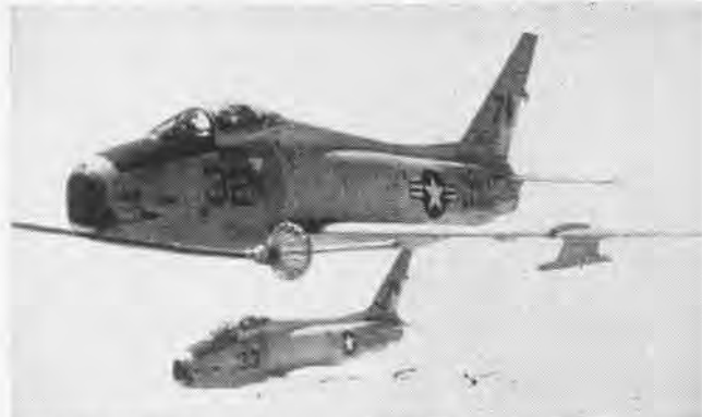
WILLOW GROVE Marines take a drink from a GV-1 tanker during air drills at Cherry Point. It was first GV-1 connection for Reserves.
