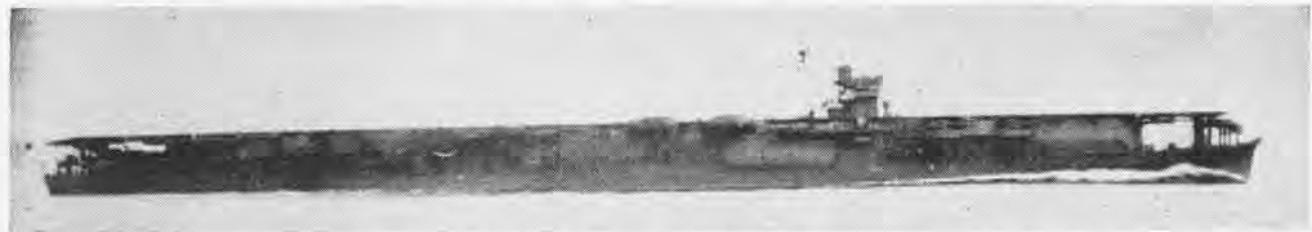
THE SORYU CLASS was first laid down in 1934 and 1936, displacing about 18,000 tons standard, at a speed of 34 knots. The Soryu had her island on the starboard (conventional) side. She, with other IJN aircraft carriers, participated in the Dec. 7, 1941 Pearl Harbor raid.
