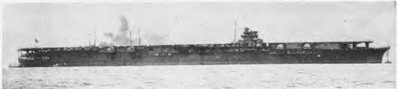
THE SHOKAKU CLASS consisted of two carriers, Shokaku (shown here) and Zuikaku . They were authorized under the Fleet Replenishment Program of 1937, displacing 25,675 tons standard. Zuikaku was first to have a bulbous bow configuration. Both were completed in 1941.
