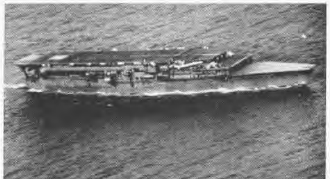
AN AERIAL VIEW of Kaga shows the chopped-off bow configuration and the starboard stack. Kaga , even after refitting, had no island
