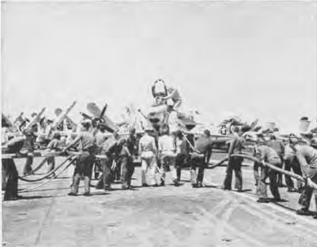
FIREFIGHTER TEAMS approach aircraft with seven hoses from windward and protect a rescuer in asbestos suit as he helps the pilot from cockpit.
