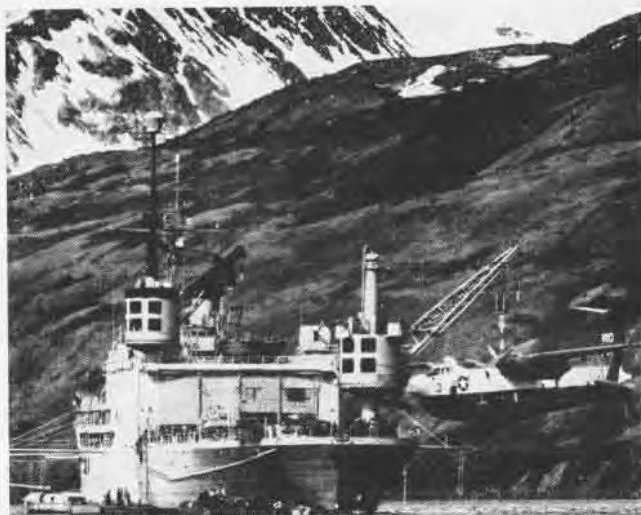
SERVICE AT KODIAK included major engine maintenance work, requiring deck hoist for P5M. VP-47 flew 1056 hours in May while deployed
