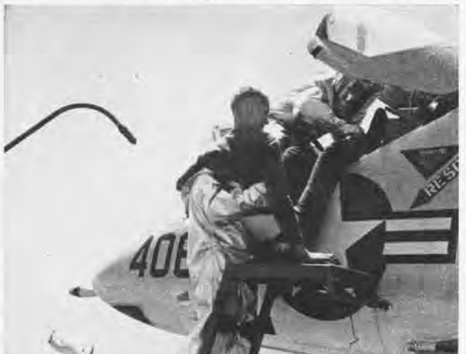
RESCUERS in asbestos suits carefully remove the "injured" pilot from plane as fog applicator protects the men by cooling the cockpit area.
