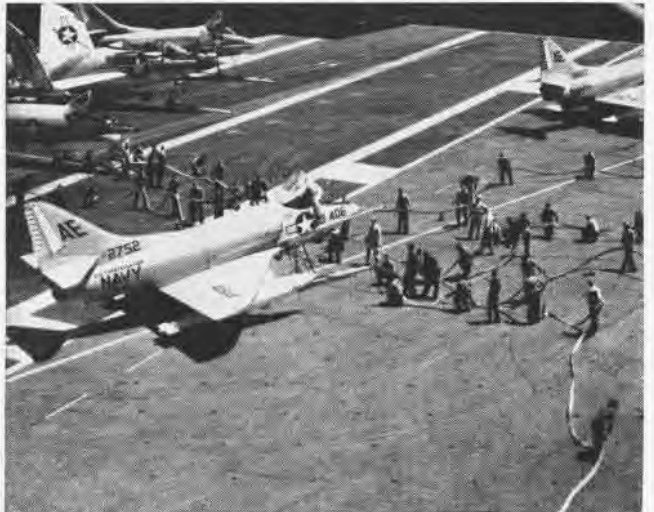
A MAN IN 'HOT SUIT' gets up on the aircraft to rescue the pilot as bosemen encircle plane to safeguard rescuers as well as smother fire.
