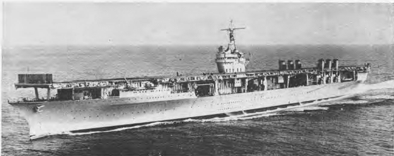
A FAMILIAR VIEW of USS Ranger (CV-4) shows forward palisade placed aboard carriers with cross-deck tie-downs to protect planes and men from wind, spray and water. She entered the Fleet Problems in 1935 and with comparatively light tonnage indicated role of small carriers.
