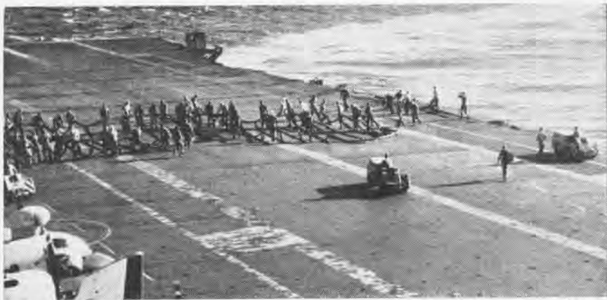
THE BARRICADE , made of nylon webbing, is built strong enough to hold a total of 200,000 pounds. Most crews are able to get the barricades into position in less than two minutes.
