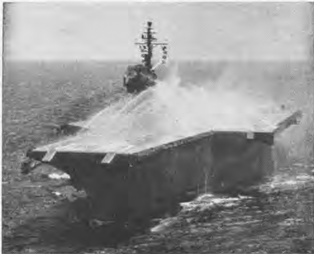
A STRIKING PICTURE of the "washdown" of one of the Navy's fast attack carriers was taken during a drill on the USS Kitty Hawk.
