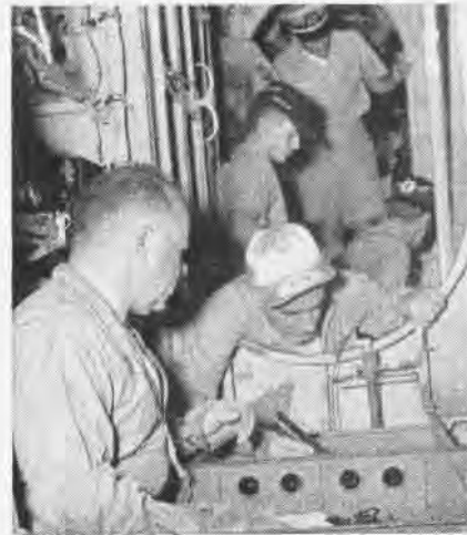
ized corrosion preventive measure is employed. Paraketon, where appropriate, is generously used. At left, E. L. Williams, AMS-1, explains the corrosion areas of the P5M to his corrosion team. Above, Cdr. J. S. Laney, former VP-40 skipper, and Tommy Thompson, Naval Aircraft Engineering Service Unit representative, inspect bilges of a P5M-2 at VP-40's station, Sangley Point, Republic of the Philippines.
