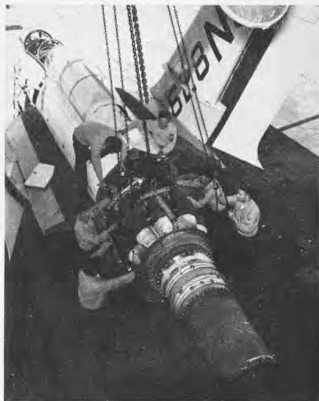
CHECK TEAM works together on engine removal, an all-hands task. The teams compete to keep quality high and maintenance downtime short.
