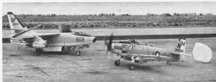
AN AD SKYRAIDER belonging to VA-115 returns to the line at NAAS Fallon, Nev., trailing its drogue chute. The A3D belongs to VAH-13, a component of CVG-11. The "Arabs" of VA-115 had watched the Skywarrior squadron use the drogue chutes and decided to try one out on the Skyraider during long taxi runs. The experiment was a success, but a Service Change for the AD is not anticipated unless a requirement arises for non-arrested landings on small carriers.
