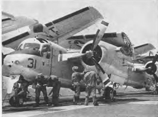
AFTER SIMULATED atomic attack, monitors on Bennington check aircraft for contamination while recorders log radiac instrument readings.
