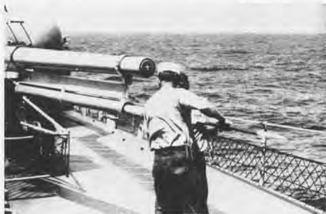
NAVY MEN LOAD HASP INTO LOKI LAUNCHER ABOARD USS McCAIN
