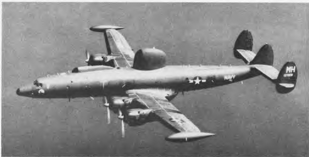
SLEEK STORM SEEKER , this giant Super Constellation is based at U.S. Naval Station, Roosevelt Roads, Puerto Rico. This big 70-ton flying laboratory carries a crew of 28 to 30 men. The radar used is second to none; with one sweep, it covers an area of some 196,000 square miles.
