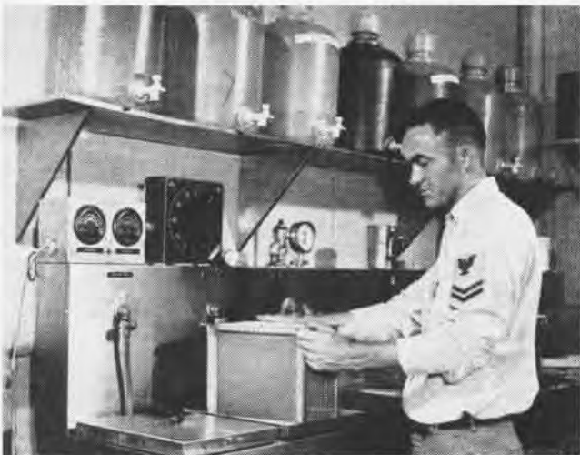
E. J. SHERRILL, PH2 , uses stainless steel, nitrogen-burst type agitation system to process black and white or color prints and films.
