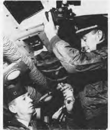
PERISCOPIC sextant is installed by Lt. Joseph A. Ryan, helped by Lt. Henry I. Demers.
