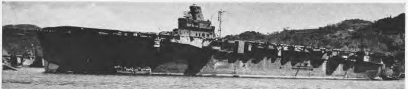
CONVERTED TRANS-PACIFIC liner, the Iunyo , was originally the Kashihara Maru , displaced over 24,000 tons standard, had 12 five-inchers and accommodated 53 aircraft. Sister ship, Hiyo , was ex- Izumo Maru . Both were badly damaged by U.S. subs, Hiyo sunk by CVL-24 planes.
