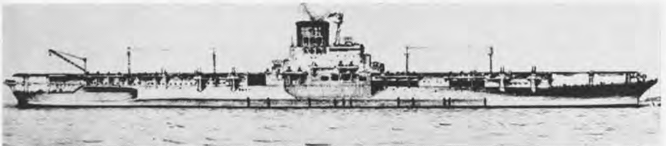
JAPAN'S MOST ambitious conversion was the CVB Shinano from the hull of a Yamato class battleship. Pre-surrender burning of the Imperial
