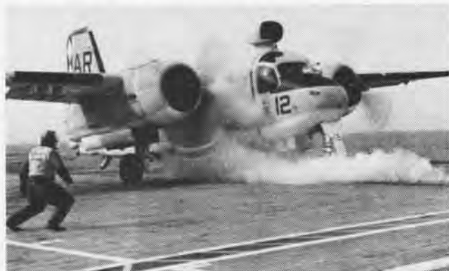
STEAM CATAPULT in USS Lexington permits this Grumman S-2D Tracker (S2F-3) to be launched in two and one-half seconds from signal.
