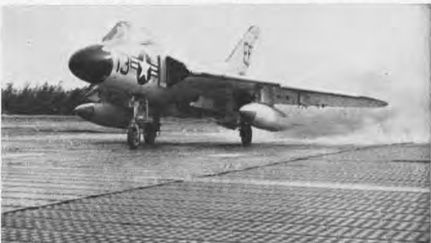
"HAVE AIRFIELD—will travel" is motto of Marines using the SATS system. Runway length is only 2000 ft., utilizing catapult assist for takeoff and arresting wire system for landings.
