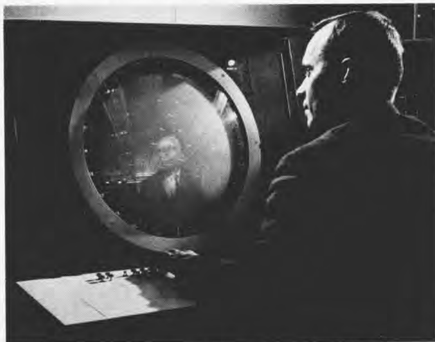
A RECOMMENDED SONOBUOY pattern, calculated by the computer, appears on display console and is studied by a technician. This is a prototype model used to test the data processing system.
