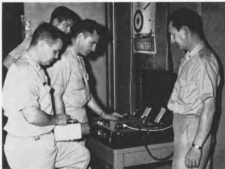
STUDENTS LEARN techniques of Sperry X Ray Control Unit from O. R. Daughenbaugh, AMCS. Machine takes X rays of material in another room, leaving operator unexposed to radiation.
