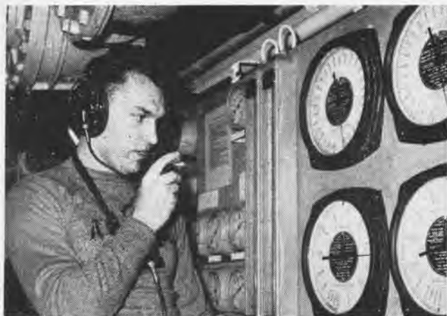
DEAN MILLS, AN, PHONES TANK-LEVEL READINGS TO FLIGHT DECK
