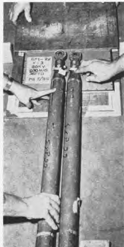
AIRCRAFT PARTS are positioned for X ray. "Invisible" defects in metal are revealed.
