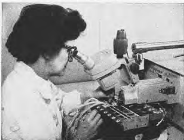
INTERIOR CONNECTIONS of the basic building blocks are made by resistance welding to ensure high environmental tolerance and reliability.
