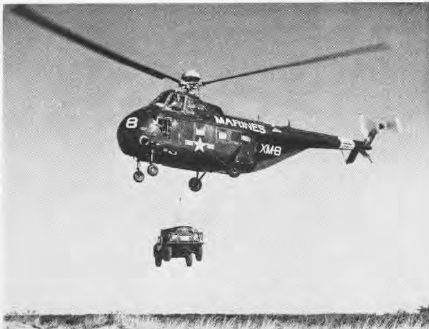
HELICOPTER DELIVERY of troops and equipment is one of Marines' tactics during beach assaults. Attachment atop rotor is called ROR (Rocket on Rotor), an auxiliary power system for lifting.
