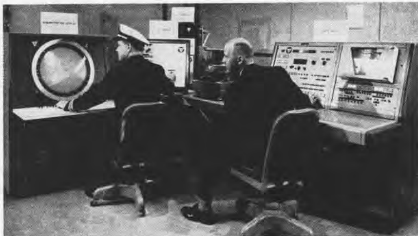
MOCK-UP OF THE EXPERIMENTAL computer and display shows compactness. Raw data is fed from the test bench (R) to the computer which generates ASW information displayed on the console.
