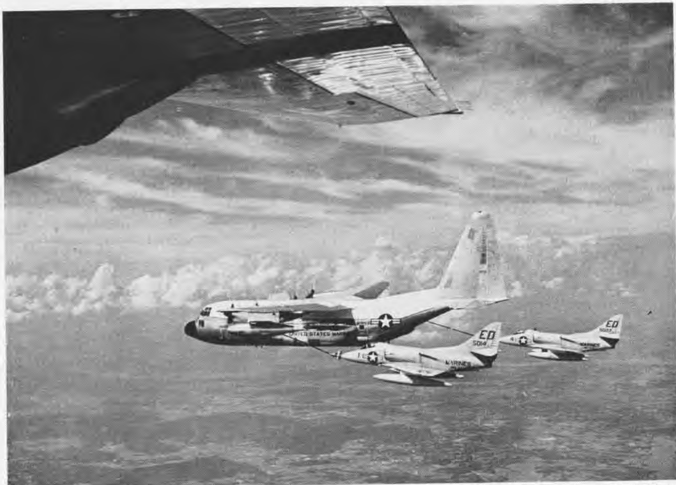
AIR-TO-AIR REFUELING operation shows largest prop aircraft (Hercules) and smallest jet attack aircraft (Skyhawk) in U.S. Marines' aircraft inventory. Story by Gen. Binney, outlining the mission of Marine aviation, is excerpted from a talk given recently to aviation writers.
