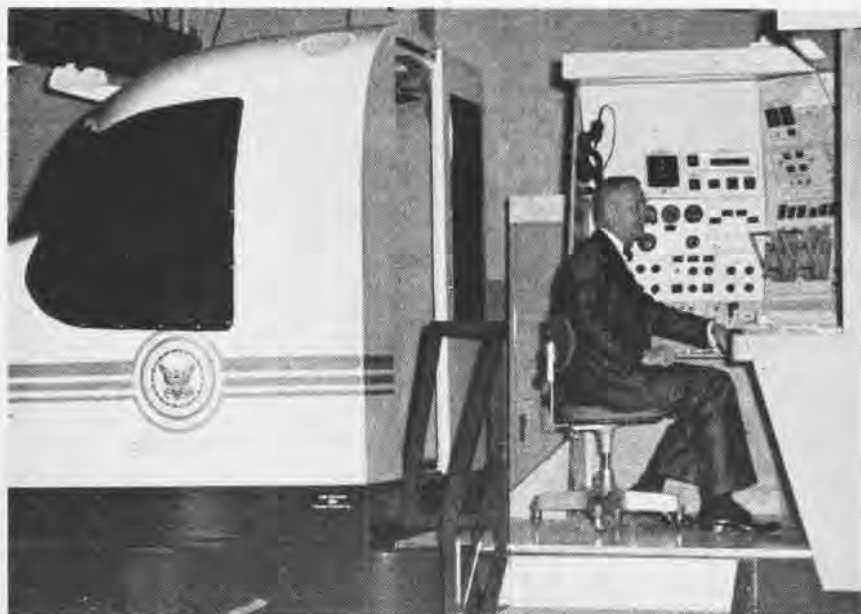
A NEW MULTI-ENGINE simulated instrument flight trainer is monitored by civilian instructor Jack Nelson at NAS Corpus Christi. Known as the 2B13, it is the youngest in the family of Link trainers, one of 13 ordered by the station. It simulates a twin reciprocating engine, land-based aircraft with a gross weight of 21,400 pounds with a cruising air speed of 140 knots indicated. The unit has a trainee station, an instructor station and D-C analog computing equipment.
