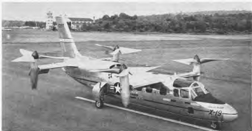
FIRST TRI-SERVICE VTOL to be rolled out is the Curtiss Wright X-19. A tandem tilt-propeller design, the X-19 is powered by two Lycoming T-55 engines. The four propellers tilt forward through approximately 90 degrees from the vertical takeoff and landing position (shown here) to the forward flight position. Built under the cognizance of the U.S. Air Force, the first X-19 is at present in the early stages of a very extensive ground and flight test program.
