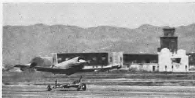
JINDIVIK , an Australian target aircraft, was evaluated at Point Mugu in 1962. Tricycle trolley is used to accelerate it down runway.
