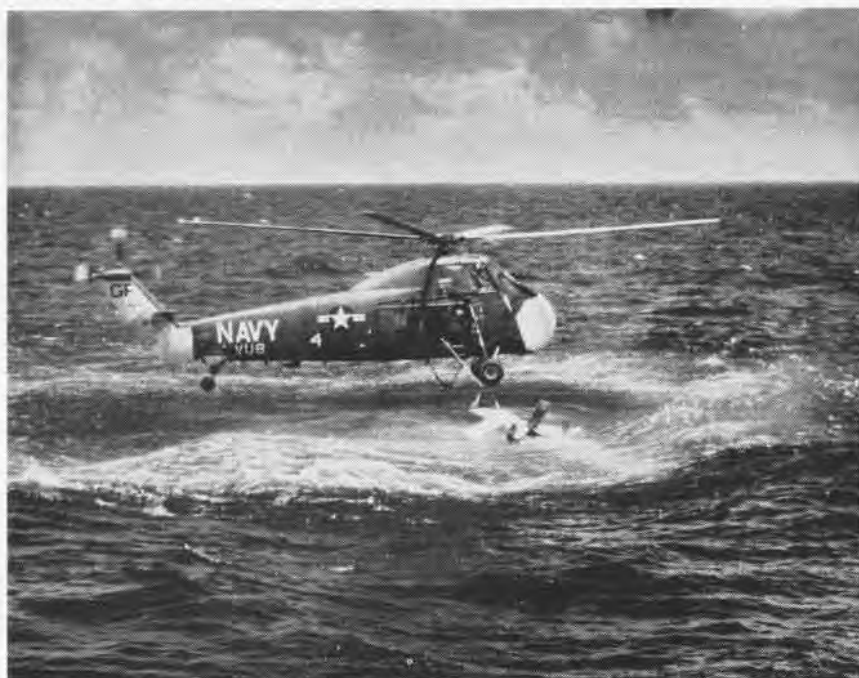
DRONE IS DROPPED IN RECOVERY AREA BY PARACHUTE AND HELICOPTER RECOVERS IT
