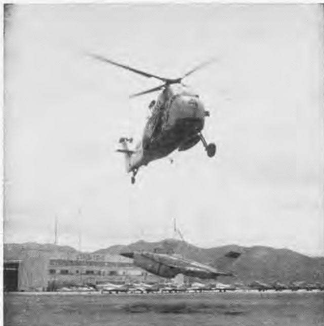
A UTILITY SQUADRON EIGHT helicopter brings back a Ryan BQM-34A (Q2C) Firebee drone to the naval station after recovering it from sea.
