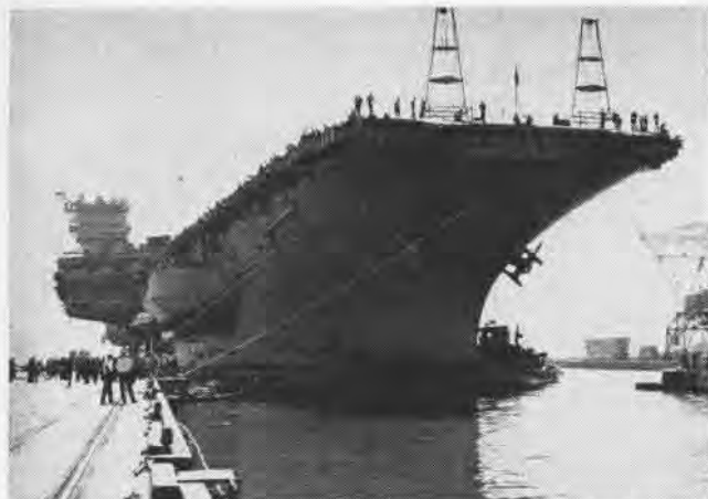
USS RANGER (CVA-61) is warped into drydock by workmen at the San Francisco Naval Shipyard, Hunter's Point, for a major overhaul.
