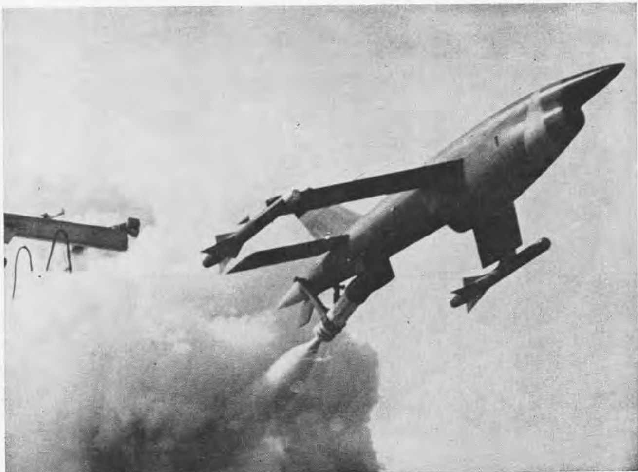
THE END RESULT of the intensive instruction given at NAF Naha, Okinawa, is the successful launching of the new Ryan Firebee. This photograph shows the drone target just as it leaves a ground launching pad, aided by the 11,000-pound thrust of a jet-assisted take-off bottle.
