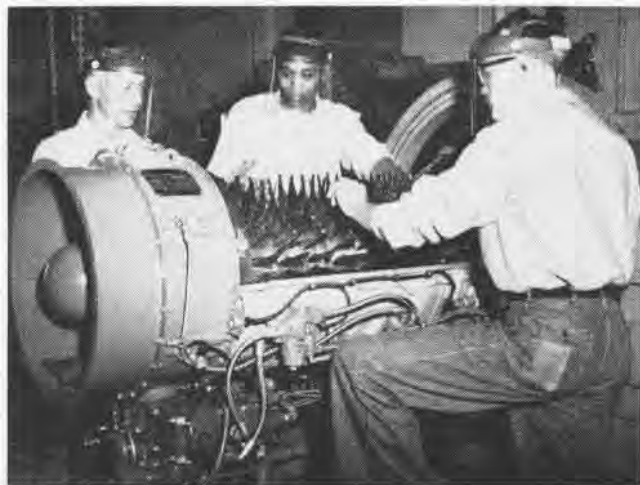
BUCKEYE Westinghouse J-34 engine undergoes thorough scrutiny by Meridian maintenance personnel. Planes are sent to Pensacola for PAR.
