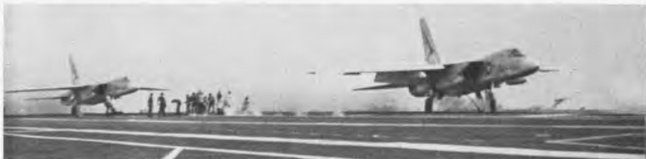
AN A-5A VIGILANTE is hurled aloft from one of CV-62's waist catapults as another Vigilante readies to taxi into the slot for hook-up. The catapult provides 42 million foot-pounds of energy, pushing the plane down a 253-foot track. End speed is approximately 140 knots.
