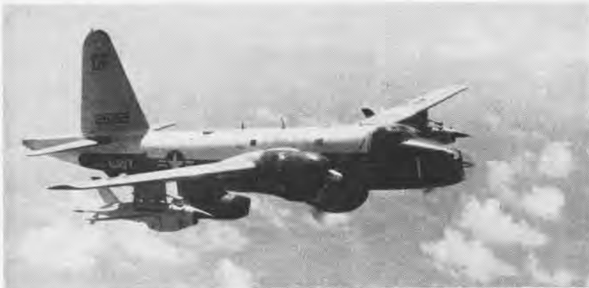
NEPTUNE IS LAUNCHING PLATFORM FOR TWO Q2C FIREBEEES, ONE UNDER EACH WING
