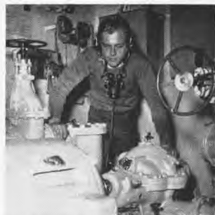
WATER BRAKE system stops piston assembly in five feet, monitored by A. F. Ecklund, AA.
