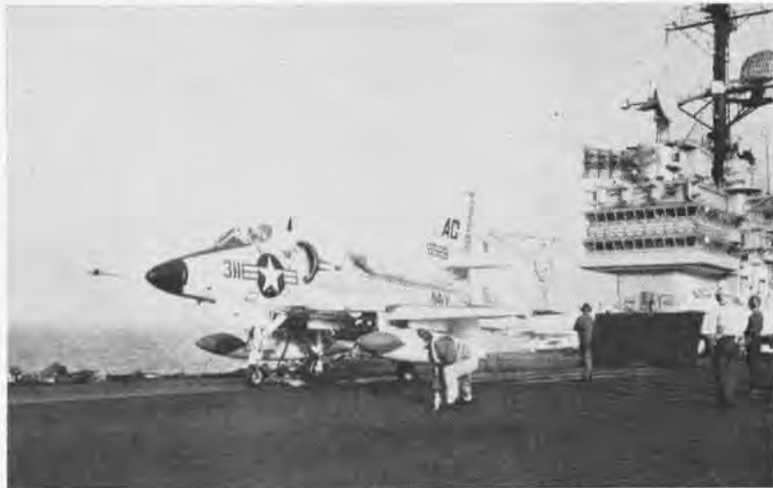
THE CATAPULT OFFICER aboard the Independence gives the signal and another A-4C Skyhawk heads down the track. The hold-back cable can be seen falling away as the tension bar breaks.
