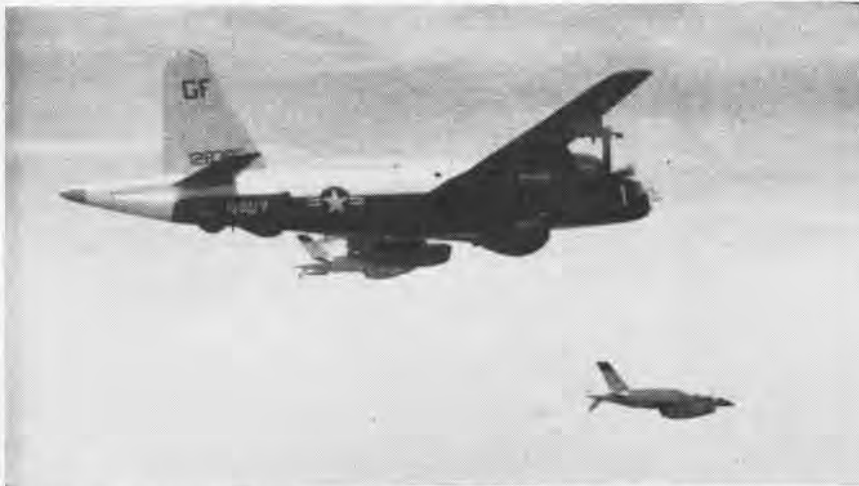
FIREBEE, ITS ENGINES AS YET UNFIRED, DROPS FROM THE WING OF A VU-8 NEPTUNE
