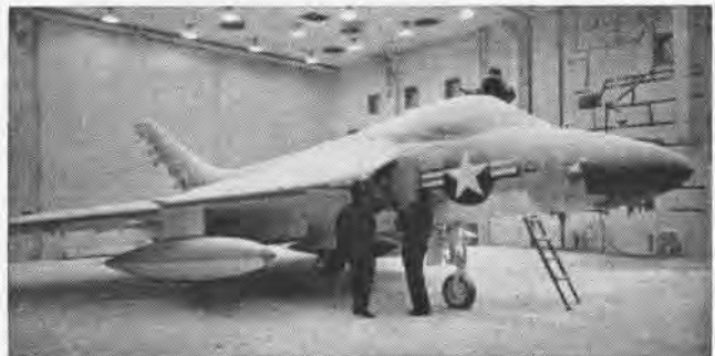
AN F-6A SKYRAY undergoes minus 40 degrees temperature in NMC's environmental test lab which experiments with missile components also
