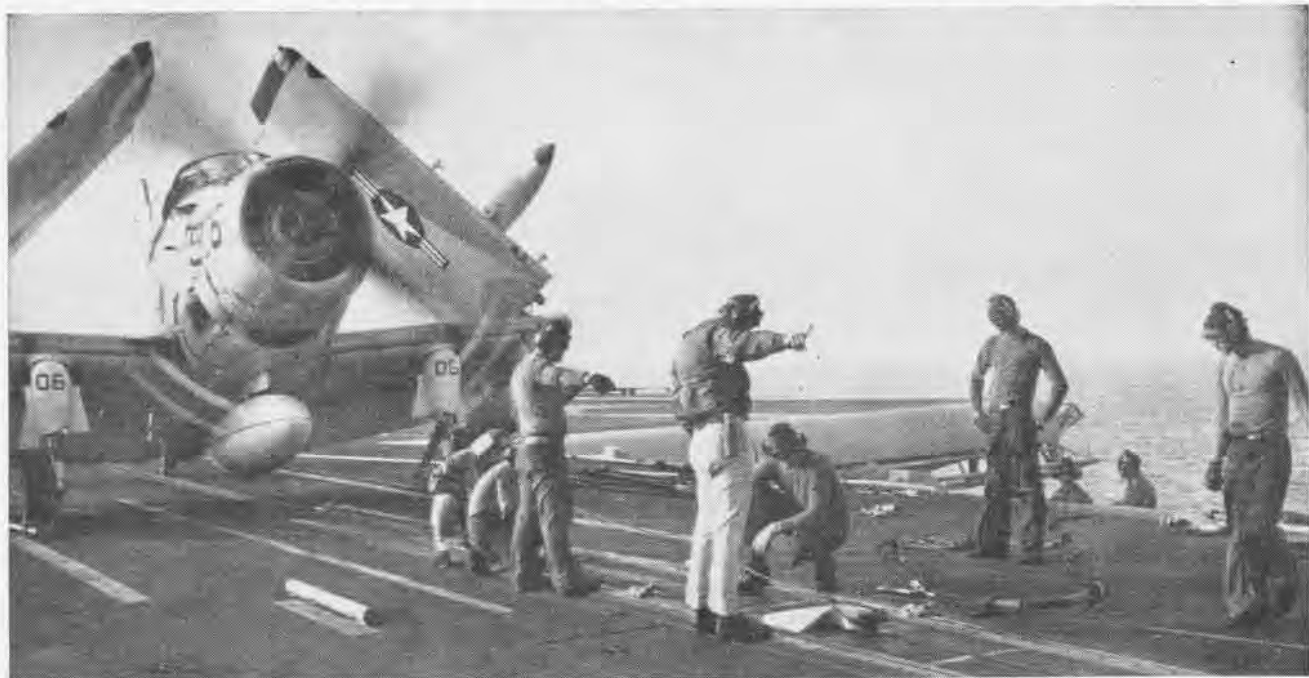
TAKING DYNAMOMETER READINGS to insure proper tensioning forces Independence prepare to launch aircraft. Green jersey men shown here are being applied during a catapult shot, V-2 Division men in the are filling some of the 17 positions manned during each catapult shot.
