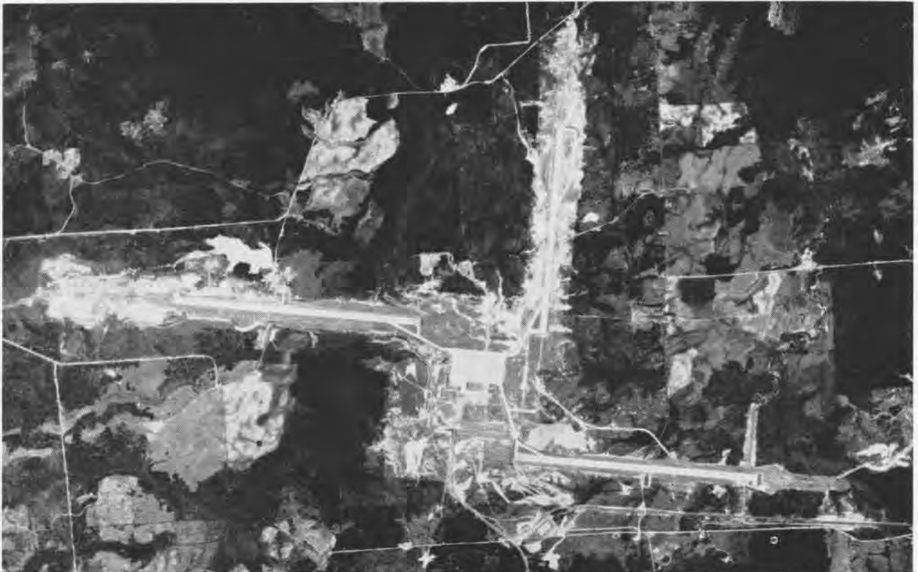
AERIAL VIEW of bangar and runways shows centralized ramp area which helps expedite taxi traffic. Aircraft can launch from one of the
