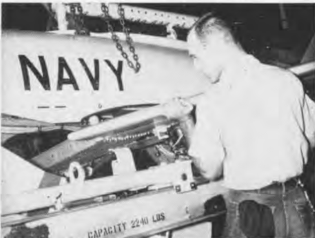
RICHARD McDONNELL learns to assemble the BQM-34A by best method—doing it. He works with others to put the wing assembly in place.
