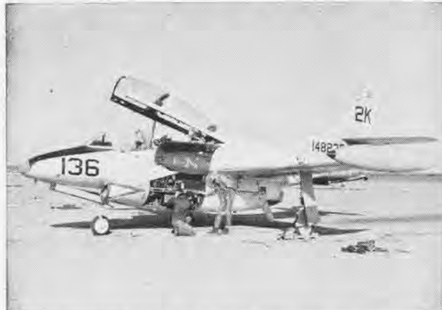
WAIST-LEVEL door provides easy access to aircraft systems components, permitting plane captain and pilot expeditious pre-flight inspection.
