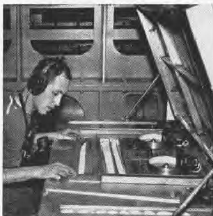
END SPEED is read by J. A. Burke, ABE3, from electrically punched recording tape.
