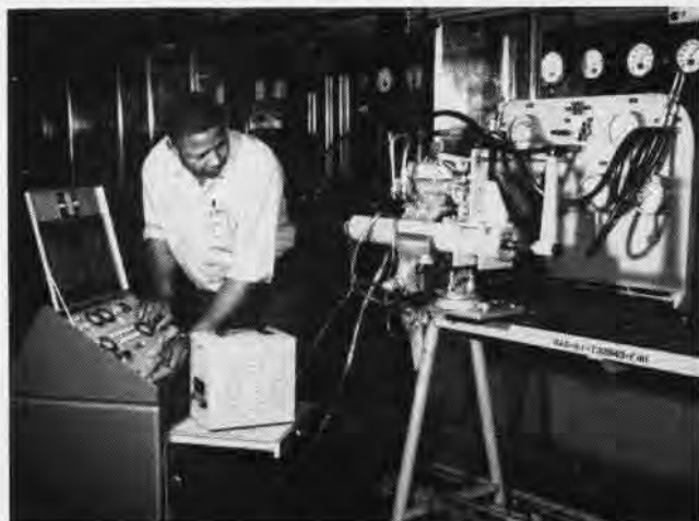
SPECIAL EQUIPMENT is needed for F-4B program. John Richardson gives stabilator cylinder assembly an electrical-hydraulic actuator test.
