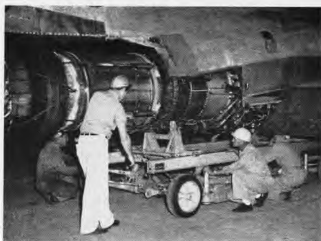
EVERY PART of the aircraft is O&R's business. Here the assembly crew rolls one of the twin J-79's into the F-4B engine compartment.
