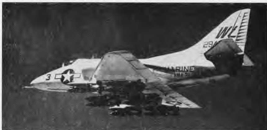
MULTIPLE CARRIAGE BOMBRACK ON A-4, FLOWN BY VMA-311, WAS EVALUATED BY VX-5
