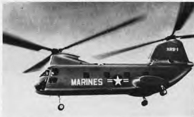
ASSAULT TRANSPORT helicopter, CH-46A (HRB-1), military version of Boeing Vertol 107, has rotor blade folding system operated by pilot.
