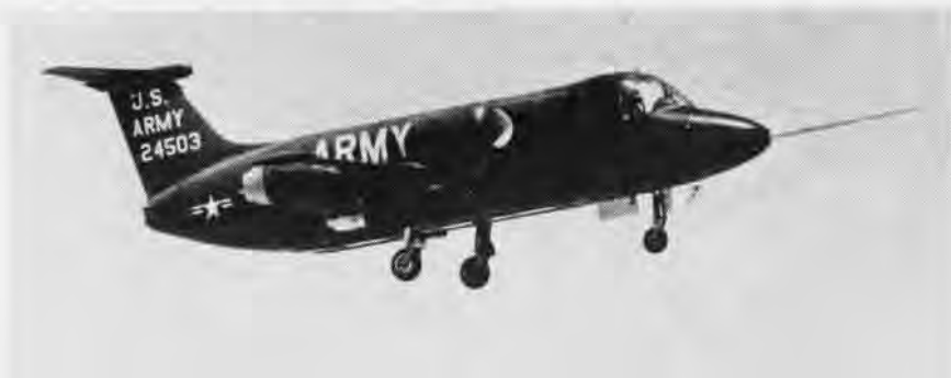
THE XV-4A HUMMINGBIRD, Army's first turboprop VTOL airplane, made its initial conventional flight at Marietta, Ga. This unique, stubby-winged, twin-jet research craft has many flight characteristics of a real, live hummingbird. It will fly straight up, straight down, hover, then dart like a flash at about 500 mph. Built by Lockheed, it is a mid-wing monoplane, 32 ft., long with a wing span of 25 ft. and powered by two Pratt & Whitney turboprops.
