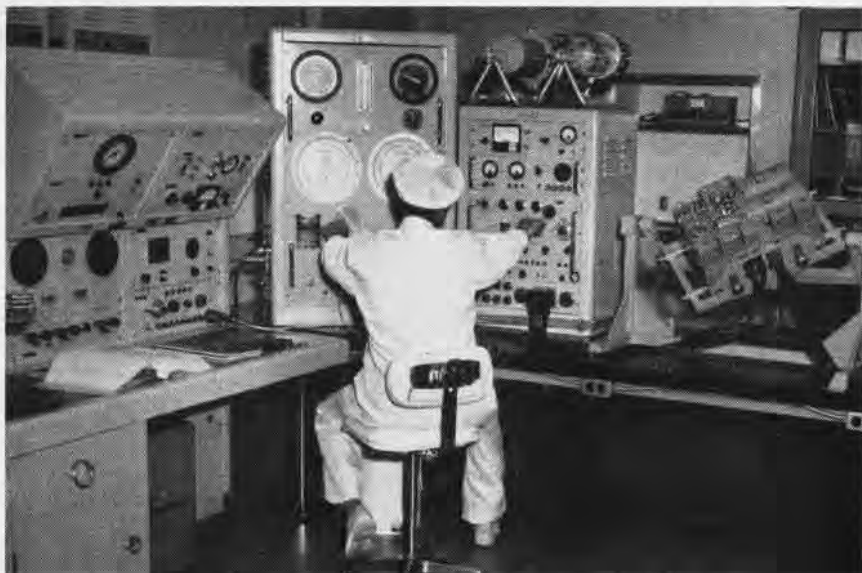
ROSLYN JOHNSON calibrates the Central Air Data Computer. The CADC was processed in the Superclean Instrument Overhaul Facility at NAS North Island as a pilot rework package.
