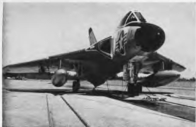
F-6A IN POSITION PRIOR TO ATTACHMENT OF LAUNCHING BRIDLE
