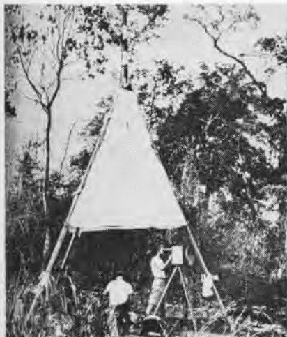
LAND PARTY uses an electronic tellurometer which measures distances up to 21 miles.
