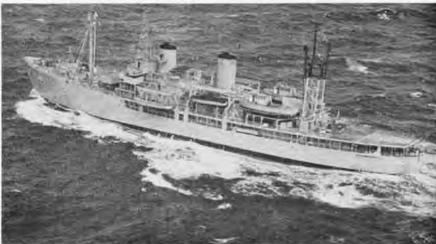
USS MAURY stores soundboats and LCVP's amidships and has helicopter platform on the fantail. Modern drafting room, print shop and photo laboratory provide for efficient recording of data.
