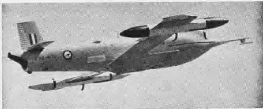
JINDIVIK , Australia's jet-powered target aircraft, has been undergoing its second series of evaluation flights at the U.S. Naval Missile Center, Point Mugu, Calif. The first series occurred in 1962. The Jindivik can take off or land in 2500 feet or less, operate up to and above 60,000 feet, and fly at near-sonic speed. Another target, the French CT-41, has also been under test at the Center. Its twin wing-tip ramjets power it to speeds up to Mach 2.7.
