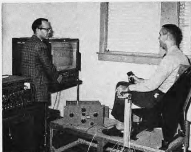
STUDENT TEST PILOTS "fly" longitudinal tracking tasks with variable "airplane" response on simulator. Scope can also display response.
