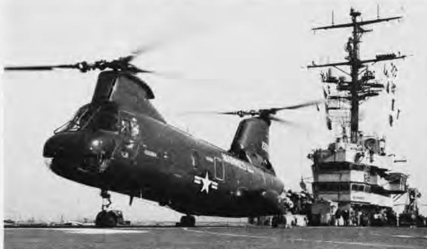
A U.S. MARINE CORPS CH-46A Sea Knight helicopter, designed and produced by Vertol Division of the Boeing Company, is shown above as it prepares to take off from and land on (at right) the flight deck of the new amphibious assault carrier, USS Okinawa (LPH-3). The series of the touch-and-go landings was performed as an early compatibility
