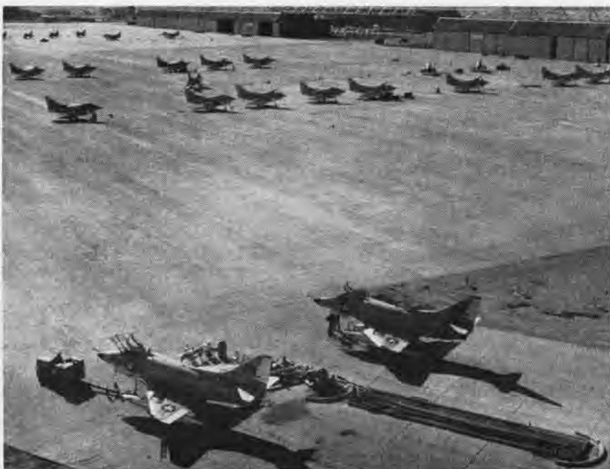
CONVENIENTLY LOCATED FUEL PITS HELP TO REDUCE TURN-AROUND TIME FOR NEXT FLIGHT
