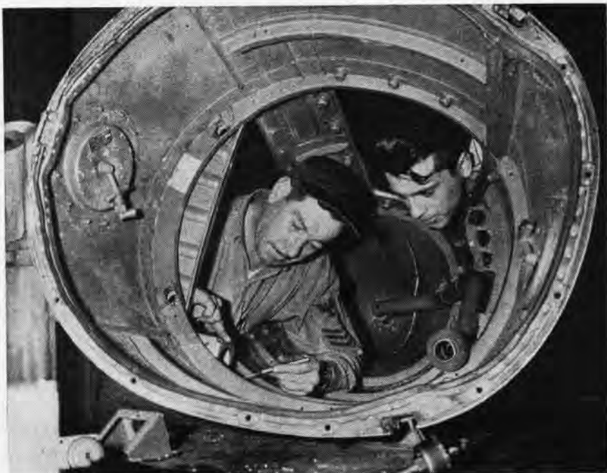
PRELIMINARY ADJUSTMENTS for effecting radar installation of service change in stripped nose section of an A-4 Skyhawk are made by G. T. Burleson, AM1, and A. Cacace, AM3.
