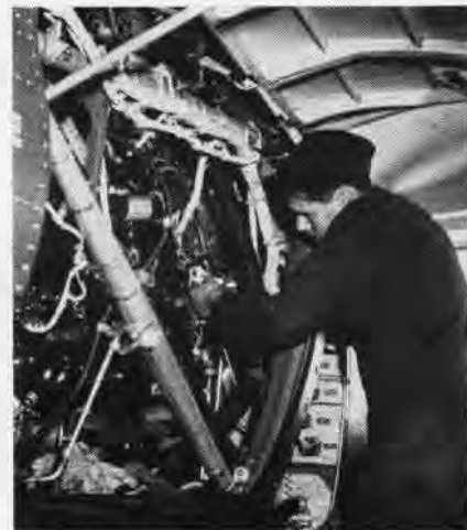
A. ALBERICO , AN, performs a scheduled maintenance check of mighty turboprop T-56.
