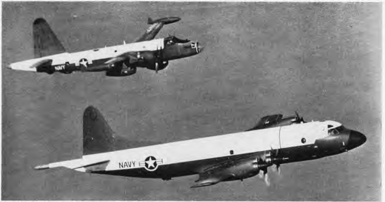
MIGHTY ORION leads its predecessor in the sub-hunting role, the venerable Neptune. Even though twice as fast in the air and more than twice as potent as a sub-killer, the prop-jet Orion can be inspected in half the time required for the less sophisticated two-engine Neptune.
