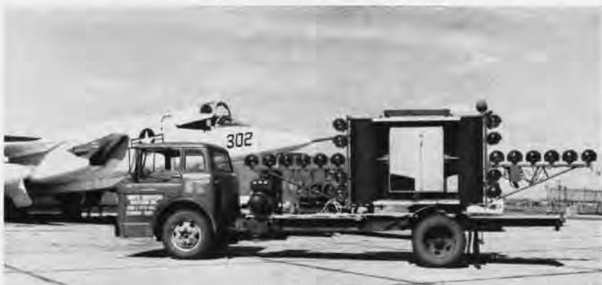
A MIRROR LANDING SYSTEM from an aircraft carrier is being used by North American's Columbus Division at Clinton AF Base in southern Ohio in a phase of the Navy preliminary evaluation program of the A-5C Vigilante. The mirror is mounted on a truck so it can be placed in different positions as required. The A-5C is the tactical reconnaissance version of the Vigilante. Earlier attack A-5A's are operational aboard the nuclear carrier, USS Enterprise.
