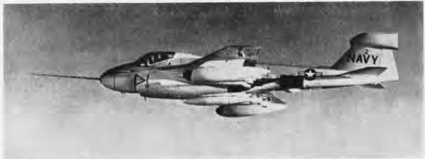
INTRUDER IN NEW ROLE —With the A-6A well along in its development, the first special version of Grumman's new all-weather attack plane has made its initial appearance. Bumps and pods house avionics equipment. The EA-6A aerodynamic prototype is shown here on its first flight.
