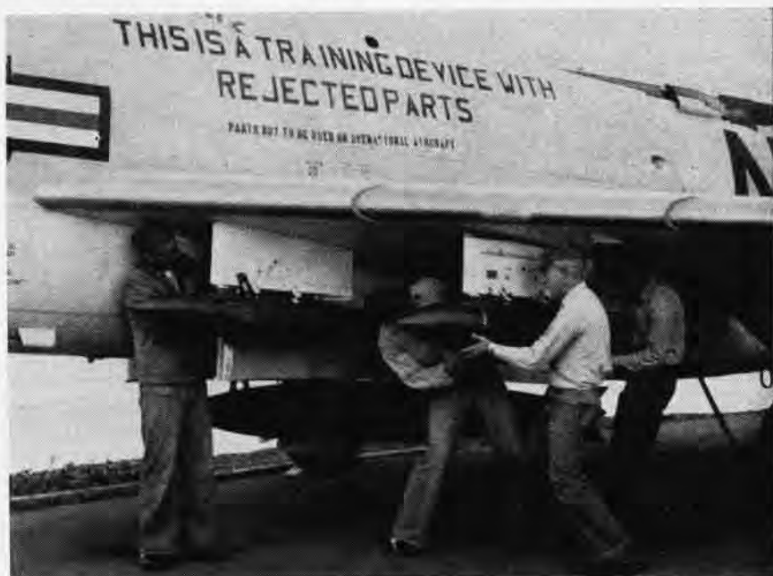
THREE TRAINEES of VF-161 undergo 'on the line' practical instruction by banging conventional ordnance on wing racks of a squadron Demon as C. M. Richards, AO1, supervises.
