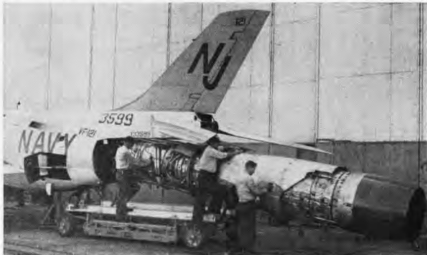
POWER PLANT crew members, under the guidance of an instructor, make final preparations on a new J-71 engine before installing it in one of the F-3 Demons flown by VF-121.
