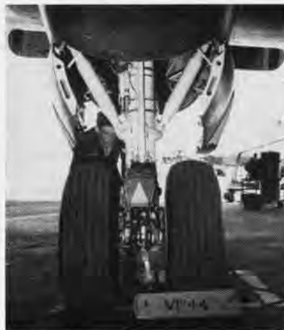
AMS3, R. C. SHOEMAKER , is absorbed in work of checking hydraulic lines on landing gear.
