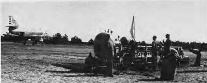
MOBILE ARRESTING GEAR BRINGS VMA-225 SKYHAWK TO A QUICK STOP ON SATS STRIP
