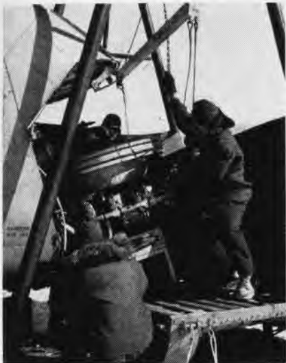
'A' FRAME HOLDS THE NEW HELO ENGINE
