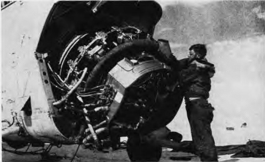
HOWARD E. HUMPHREY, ADCR, CONNECTS THE EXHAUST SYSTEM OF THE NEW ENGINE
