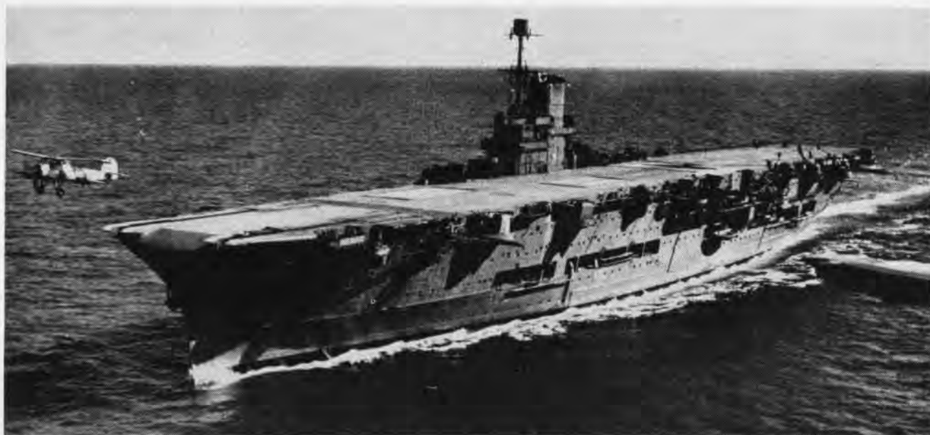
HMS ARK ROYAL , a 22,000-tonner, had large hangars on two decks, three elevators. She boasted the largest wardroom in the Royal Navy. In war, her fighters downed or damaged more than 100 enemy aircraft, her bombers wrecked Sardinian airfields, hit Italian Navy.
