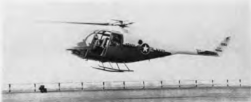
FIRST XH-51A flight photo shows new Army-Navy rigid rotor helicopter. An advanced concept research vehicle built by Lockheed-California Co., XH-51A is designed for speeds in excess of 150 mph. It features "hands-off" flying capability at all speeds with no form of autopilot or artificial stabilization. It is equipped with retractable landing gear, has free-falling skids operable without hydraulic power, and is stable and controllable with power on or off.
