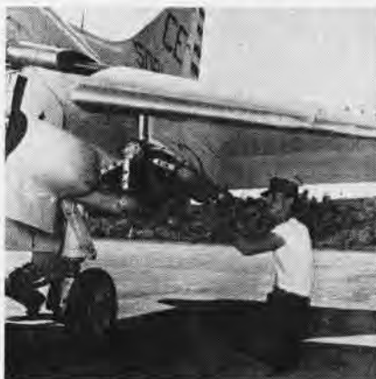
MARK 76 BOMBS are loaded by ordnance man prior to training hop during Caribbean cruise.
