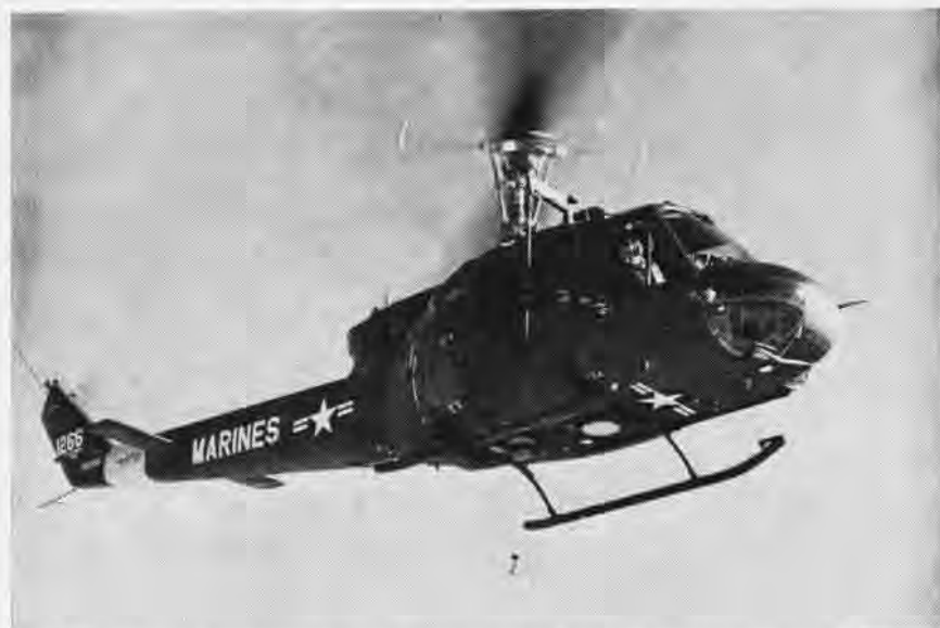
THE MARINE CORPS' new assault support helicopter (ASH) is being manufactured by Textron's Bell Helicopter Company. The turbine-powered model, to be known as the UH-1E, is basically the same as the Army's famed UH-1B Iroquois. Helicopters of the Army series hold six world flight records. The Marine version will vary from the Army's helicopter in three ways: It will have a personnel hoist, rotor brake and special navigational/communication equipment.
