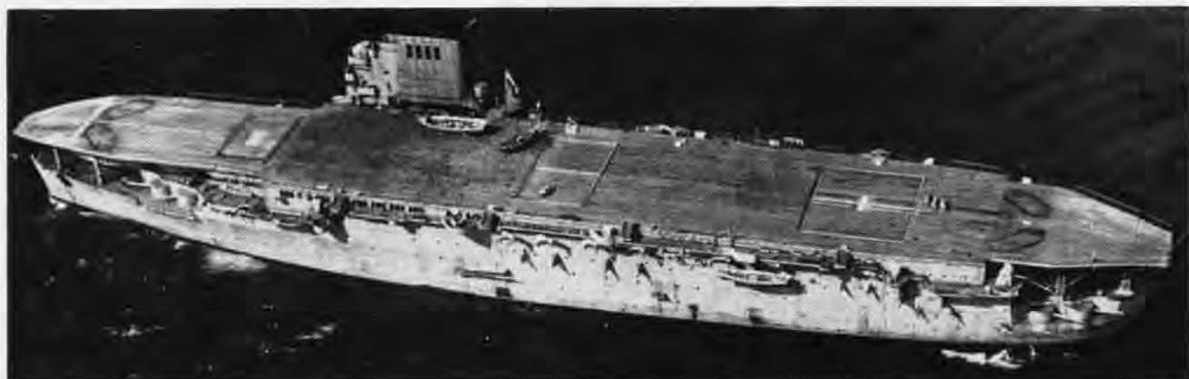
BEARN WAS the only carrier France had completed before the start of WW II. Converted to aircraft carrier characteristics between 1923 and 1927, she had a speed of 21.5 knots, or a radius of 6000 miles at 10 knots. She spent most of the war years at Martinique.
