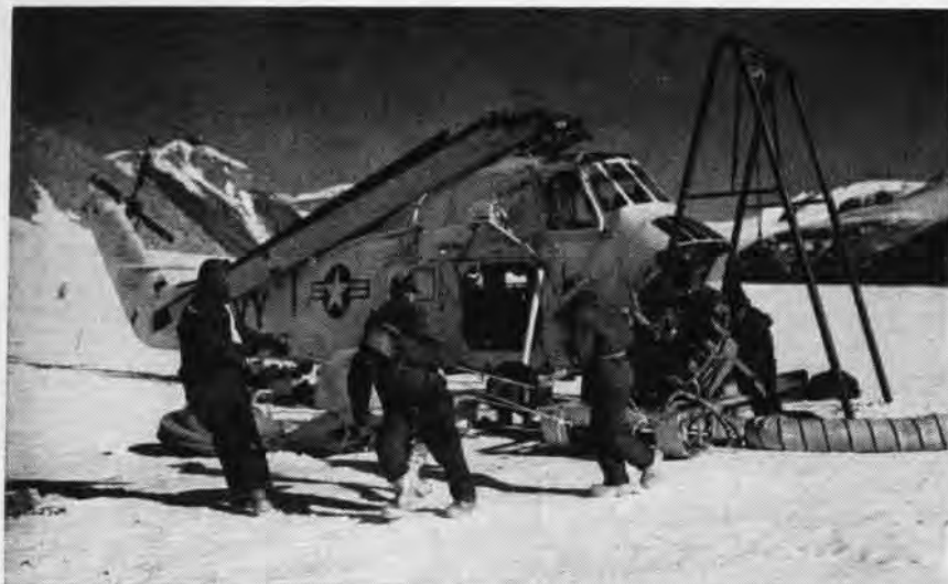
WITH THE AID OF A JERRY-BUILT AND JURY-RIGGED 'A' FRAME, THE ENGINE IS PULLED OUT
