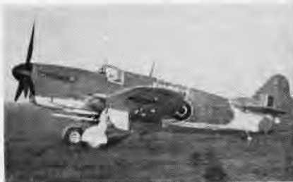
FAIREY FIREFLY was World War II two-place carrier fighter used by the British Navy.
