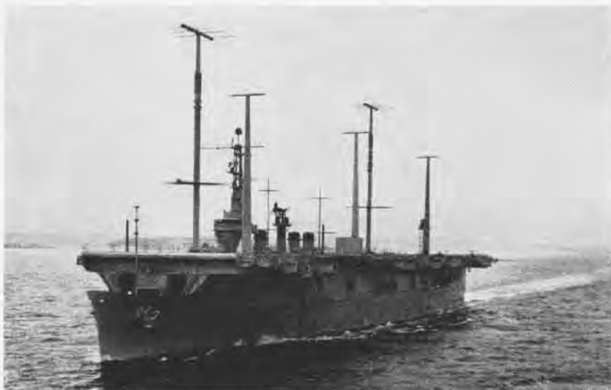
THE COMMAND SHIP, USS Wright (CC-2), formerly an aircraft carrier (CVL-49), represents a new concept in command at sea. As "the voice of command," it can be heard by ships, aircraft and stations throughout the world. Wright's command spaces, designed for theater type presentations, are equipped with projection equipment and motion picture screens. Room is amply provided for command operations, plotting, charts and graphics, briefings and conferences. On the antenna deck are arranged the largest, most powerful transmitting systems ever installed on a naval vessel. The largest antenna towers 114 feet above deck. Wright's carrier days are not wholly a thing of the past; there is room for helicopter landings aft of the "trees."
