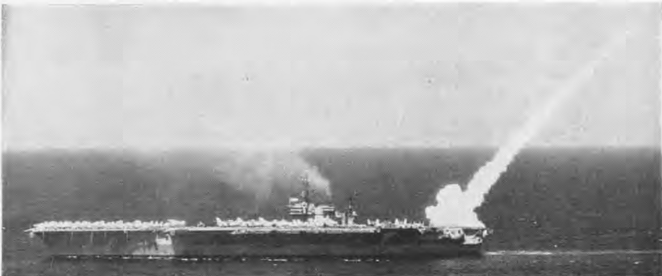
USS CONSTELLATION (CVA-64), sister ship to Kitty Hawk , fires a Terrier missile. Basic design of the Kitty Hawks is of the Forrestal class. The angled area of flight deck is some 40 feet longer than the Forrestals , and catapults and elevators installed have greater capacity.
