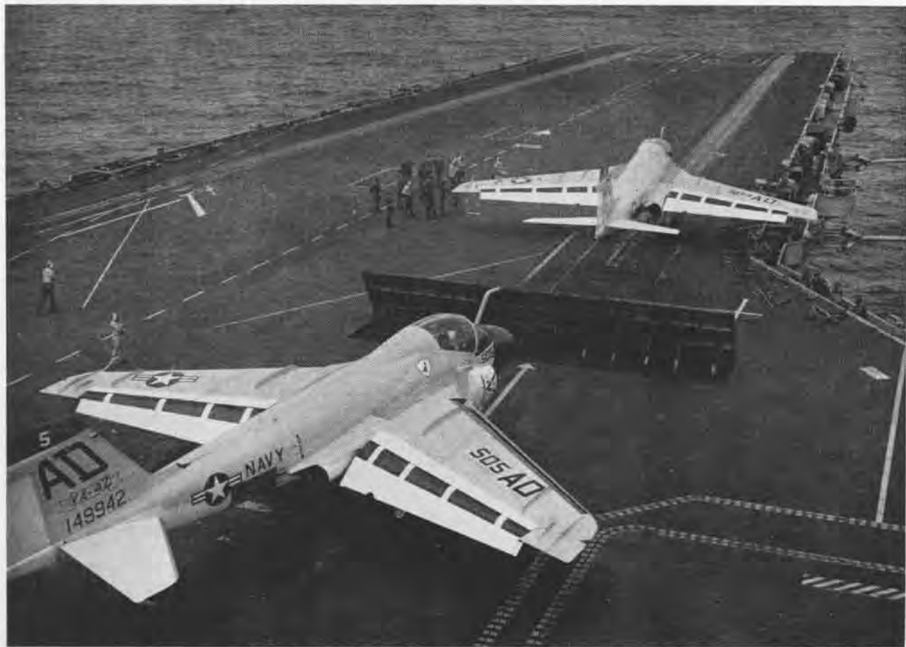
ONE INTRUDER IS ON A FORRESTAL CATAPULT WHILE ANOTHER STANDS BY. NEW CRAFT WILL REPLACE A-1 SKYRAIDER AS ATTACK BOMBER
