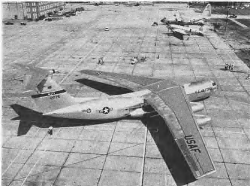
UNVEILED at the Lockheed-Georgia Company, Marietta, Ga., USAF's C-141 StarLifter dwarfs predecessors, C-47 and C-130, in background. Global transport has 160-foot wing span, four jet engines, can airlift 90,000 pounds, carry 154 troops and fly at 550 mph. President Kennedy called the plane's debut "a good moment for the United States." He also referred to the C-141 as the world's fastest cargo-carrying airplane. Flight tests on the aircraft begin in December.
