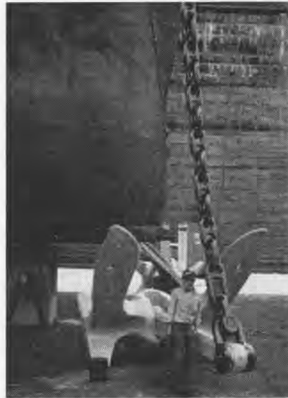
THE AUTHOR INSPECTS Champ's 15-ton starboard anchor resting on bottom of dry dock.
