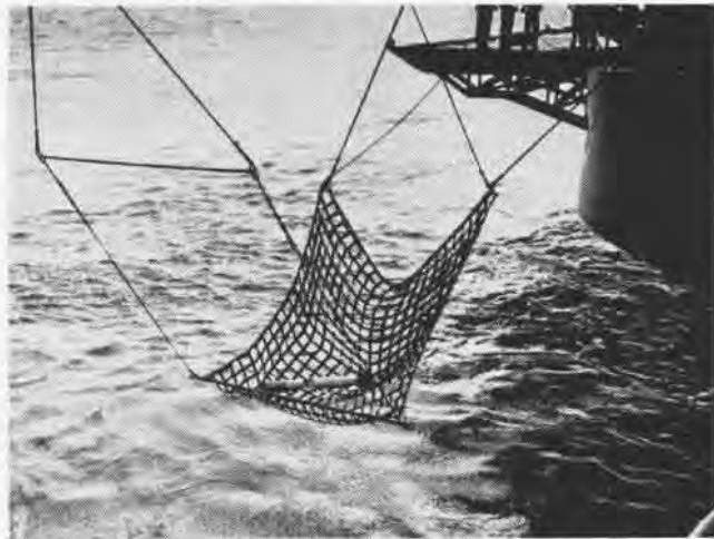
A NEW METHOD of retrieving aircraft exercise torpedoes is devised by Intrepid , using boat and airplane crane and a 14-sq.-ft. cargo net.
