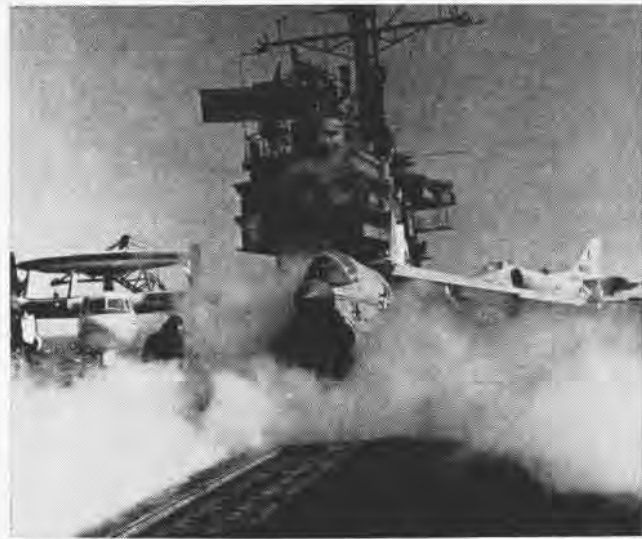
A CRUSADER is launched by a powerful catapult system installed in Forrestal . Angled deck resulted from experiments in USS Antietam .
