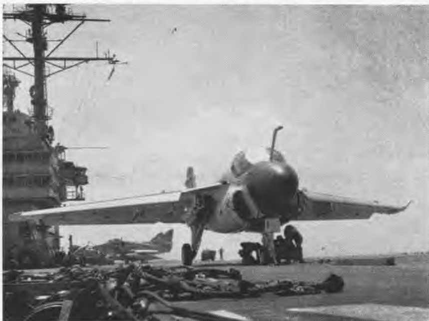
AN INTRUDER, USING ITS 'NOSE-WHEEL TOW,' IS HOOKED UP FOR LAUNCH ON CATAPULT
