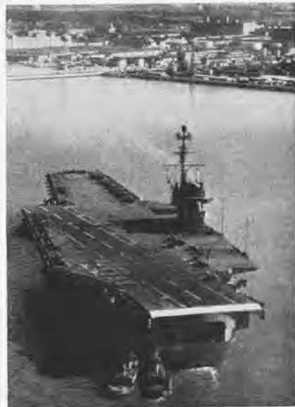
USS RANGER'S after flight deck was altered slightly to provide a longer overall length.
