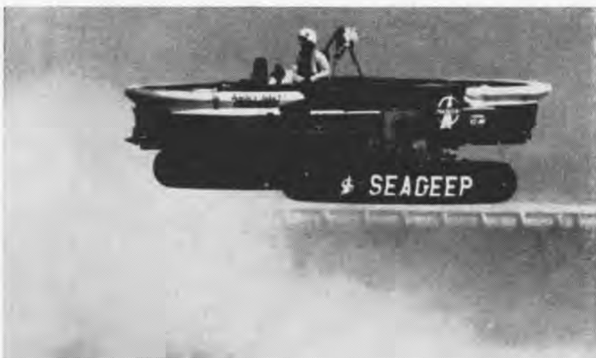
PIASECKI'S SEAGEEP, powered by Avresearch's 331-6 turbine, has been tested on Chesapeake Bay. The final phases of the flight test were performed at NATC Patuxent River, Md., with Piasecki's Chief Pilot, Stuart "Tammy" Atkins, at the controls. When taxiing on the water, landing or taking off or hovering, the Seageep does not generate spray which would soak the aircraft or impair pilot's vision. Wide-tread floats and low center of gravity stabilize the Seageep.
