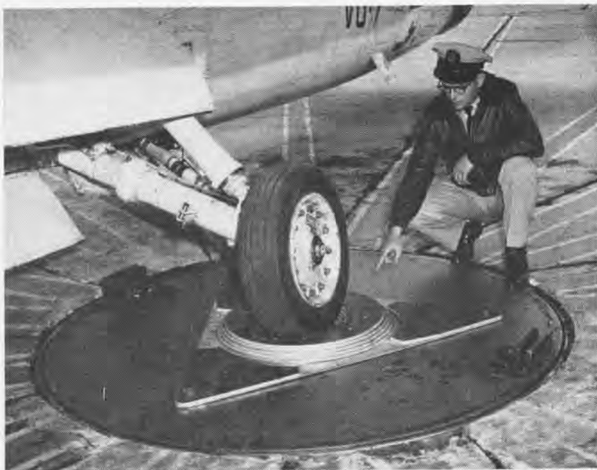
CHIEF COCHRAN INDICATES HOW DEVICE HE INVENTED GRIPS TIRE OF A VU-7 CRUSADER
