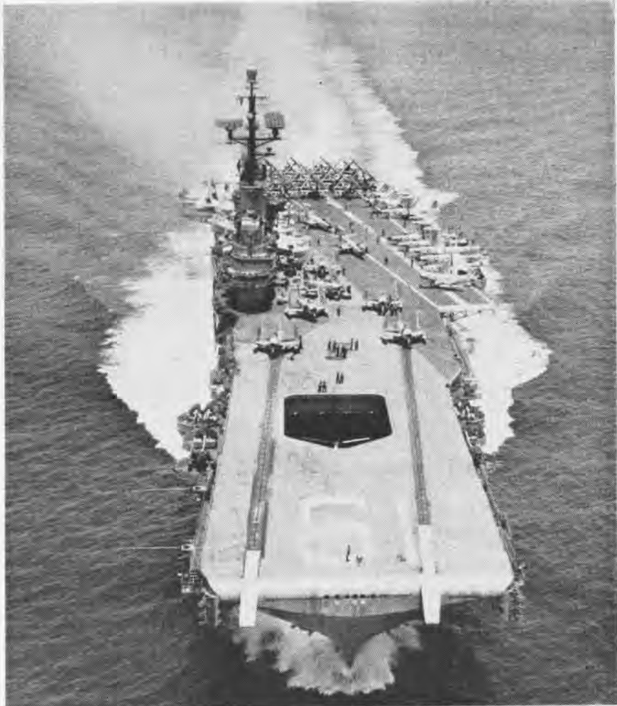
HANCOCK WAS the first carrier to receive the C-11 steam catapult. Note the TACAN "bucket" atop mast for homing, enlarged elevator, and the distinctive bridle catchers at end of catapults.
