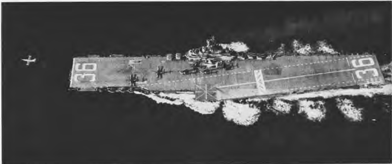
ANTIETAM TESTS British-designed angled deck in the Virginia Capes area in April 1953. Fifteen types of aircraft were used during evaluation period. Pilots were enthusiastic, for it eliminated barriers, barricades, and danger of parked planes at runway's end.
