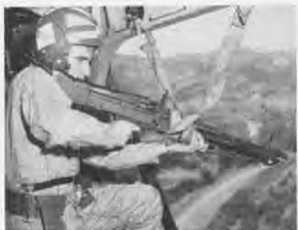
M-60 IS so rigged with straps that crewman is able to fire horizontally or vertically.
