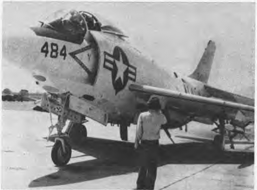
LT. ROGER BELLNAP, USN , prepares to start engines on this F-3B at the U.S. Naval Missile Test Center, Point Mugu, Calif., prior to Operation "Nite Owl." A Sparoair two-stage, solid-propellant probe, mounted beneath the wing at right, carries instruments to measure the ultraviolet radiation of the stars. The atmosphere's ozone layer at about 100,000 feet absorbs the ultraviolet rays emitted by the stars, so that studies of this kind cannot be conducted from the earth's surface. Lt. Bellnap launched the Sparoair in a nearly vertical attitude at about 30,000 feet over the Pacific Missile Range sea test area. The probe reached some 350,000 feet.
