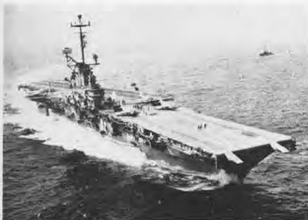
ORISKANY was the first of the carriers to be reworked in the post-war modernization program. Angled deck was installed in Project 125A.
