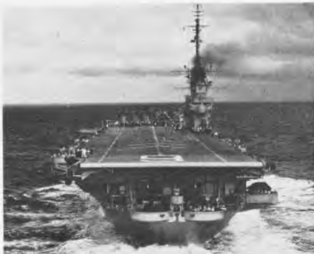
ESSEX joined the Oriskany class after Project 27A. She is shown after Ship Improvement No. 1. CV-9 got her angled deck in Project 125.
