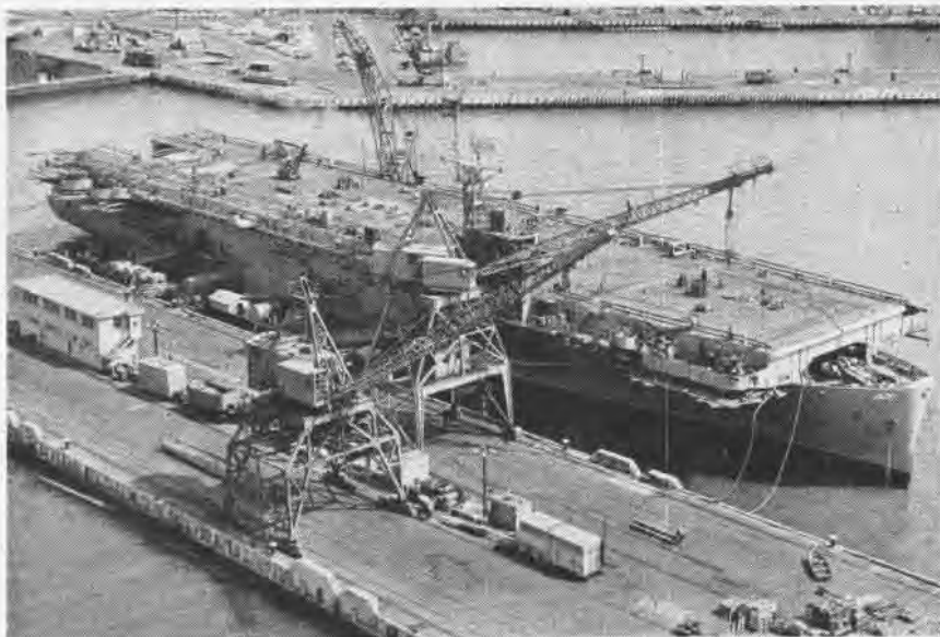
THETIS BAY (CVE-90) was redesignated CVHA-1 and started the phasing out of CVE's from the Navy's list of combatant ships. Here the ship is being converted for the operation of helicopters.
