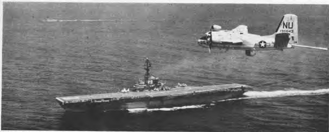
ITS MAD GEAR BOOM EXTENDED, S2F TRACKER FLIES ACROSS BOW OF ITS HOME SHIP, USS YORKTOWN, DURING ANTI-SUBMARINE OPERATIONS
