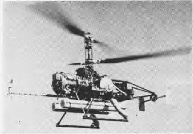
THE DASH (drone anti-submarine helicopter) is a vehicle that is to be used as a platform for delivering torpedoes in anti-submarine warfare.
