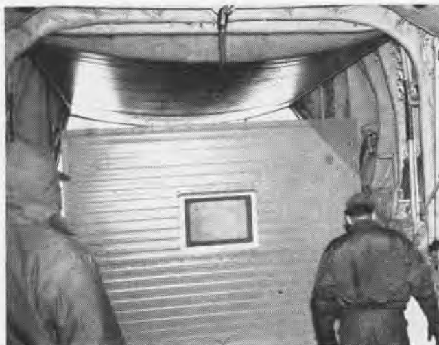
INTERIOR VIEW of one of the squadron's LC-130F Hercules shows minimum clearance between the designed module and the cargo aircraft.
