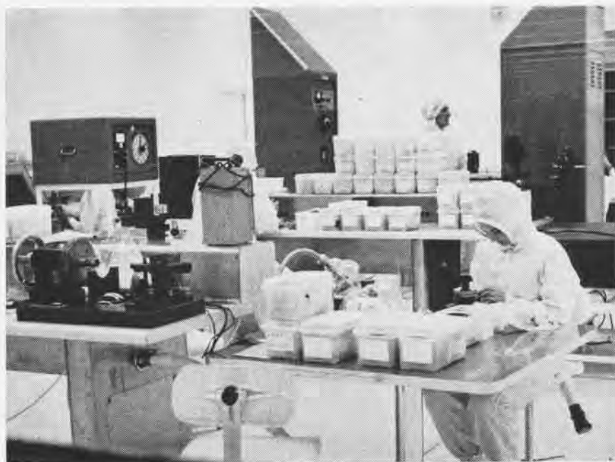
THIS ULTRA-CLEAN white room has standards of cleanliness so great that they meet the exacting tolerances of high precision instrument processing. Employees work in lint-free clothing.
