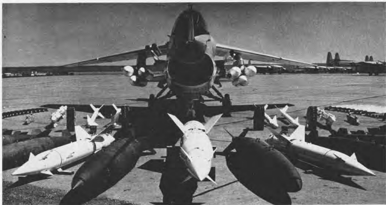
SURROUNDING CHANCE VOUGHT'S F-8 Crusader all-weather fighter is the armament which can be carried by this high-performance aircraft on a single mission. Various missions call for different types of attack; Navy strives to offer commanders a flexibility in choice of weapons.
