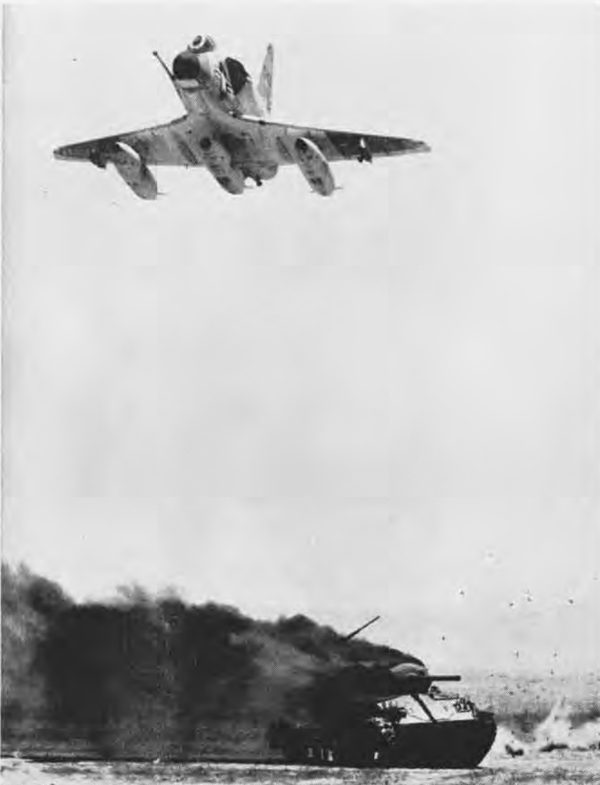
AS THE SKYHAWK passes over the tank target, three pods which make up the Hipeg gun system can be clearly seen beneath the airplane. Note shell cases flying in vicinity of tank target.
