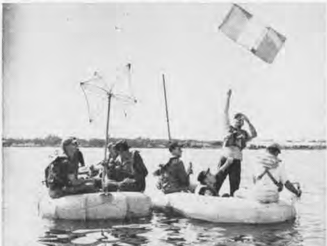
LIFE RAFTS AFLOAT and manned, the radar reflector (1) produces a typical blip on search plane's screen, as kite lifts radio antenna.
