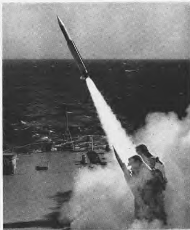
A TARTAR surface-to-air missile is launched from the fantail of the USS Norton Sound. It is designed especially for use aboard destroyers.
