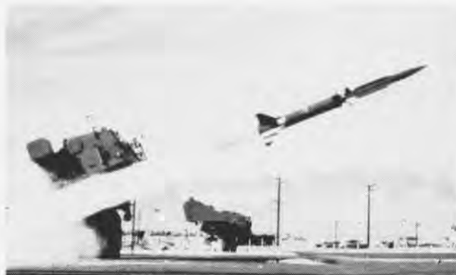
NAVY'S ADVANCED Terrier, an all-weather, surface-to-air missile, blasts off in a test firing at Naval Ordnance Test Station, China Lake, Calif.
