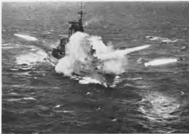
IN THE FIRST such launching by any Navy, guided missile cruiser USS Albany simultaneously test-fired three missiles: two Talos, one Tartar.
