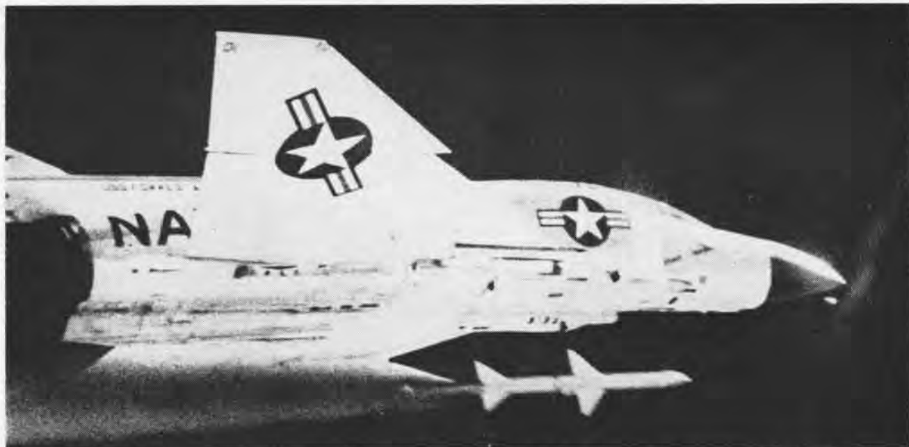
THE ADVANCED SPARROW III is the prime armament for the F-4 Phantom II. It can also be carried by the F-3B Demon. This supersonic, all-weather, radar-guided, air-to-air missile is 12 ft. long, weighs 350 lbs., attains speeds over 1500 mph seconds after launching.
