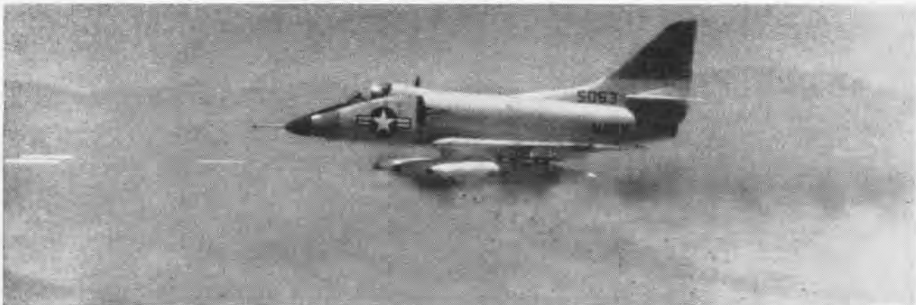
A NAVY A-4 attack aircraft fires Hipeg at a tank target a quarter of a mile away. The three pods slung underneath the aircraft can each fire at the rate of 4000 rounds of 20mm cannon shells per minute. Here tracers (in front of aircraft) have been mixed with armor-piercing shells.
