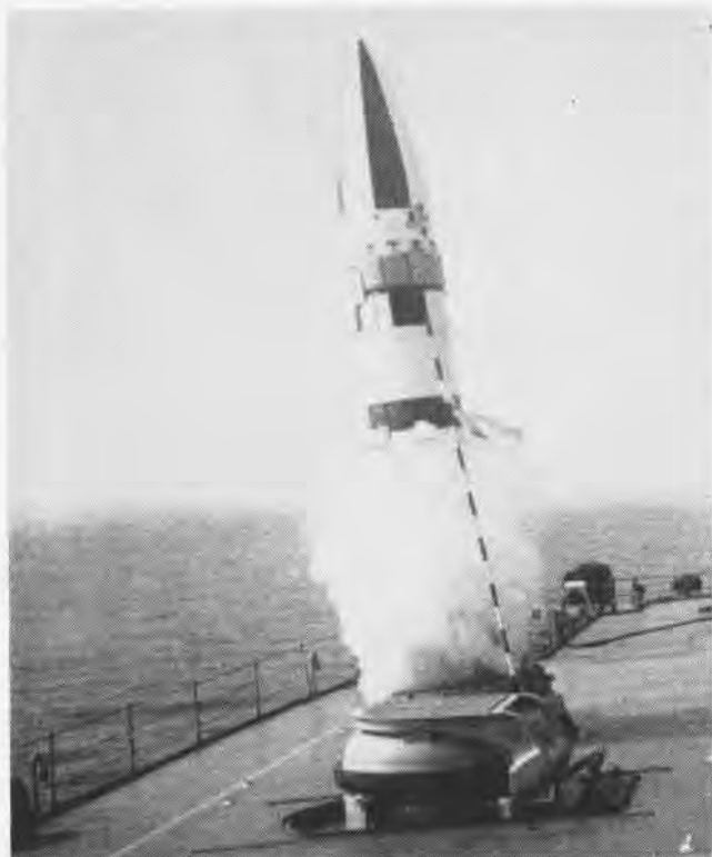
EXPERIMENTAL A-3 POLARIS missile is shown as it leaves missile launching tube of Observation Island (EAG-154) off Cape Canaveral.
