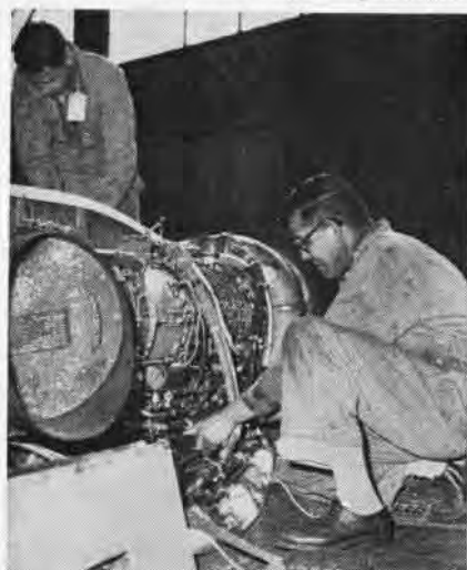
DAVIS and Julio Garcia install the twin T-58 engines on the H-3 during assembly stage.
