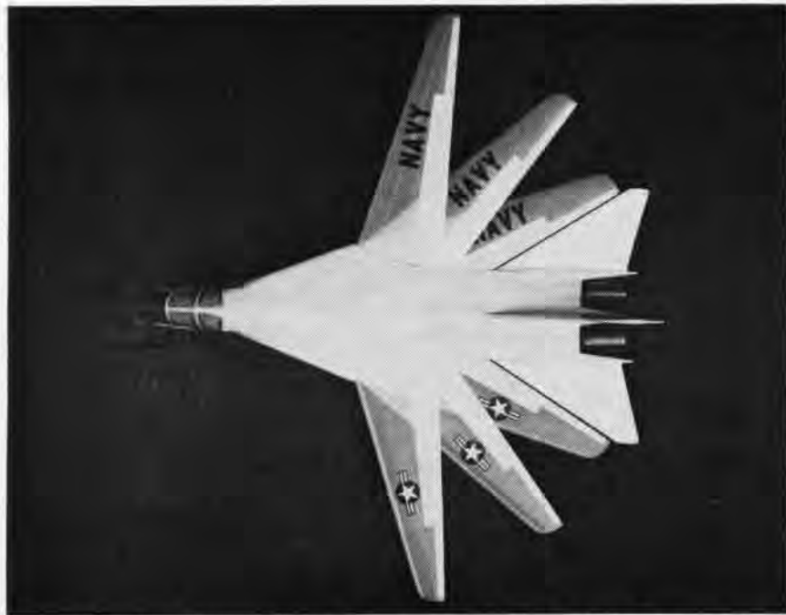
ARTIST'S DRAWING SHOWS DIFFERENT POSITIONS OF F-111'S VARIABLE SWEEP WINGS
