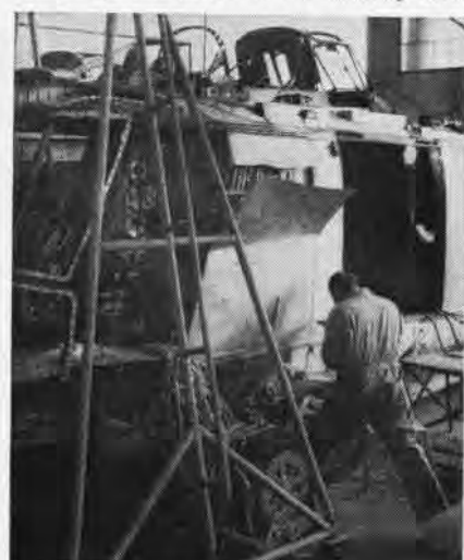
MECHANIC ARREGUI is attaching new skin to a crash-damaged UH-2A which is in overhaul.
