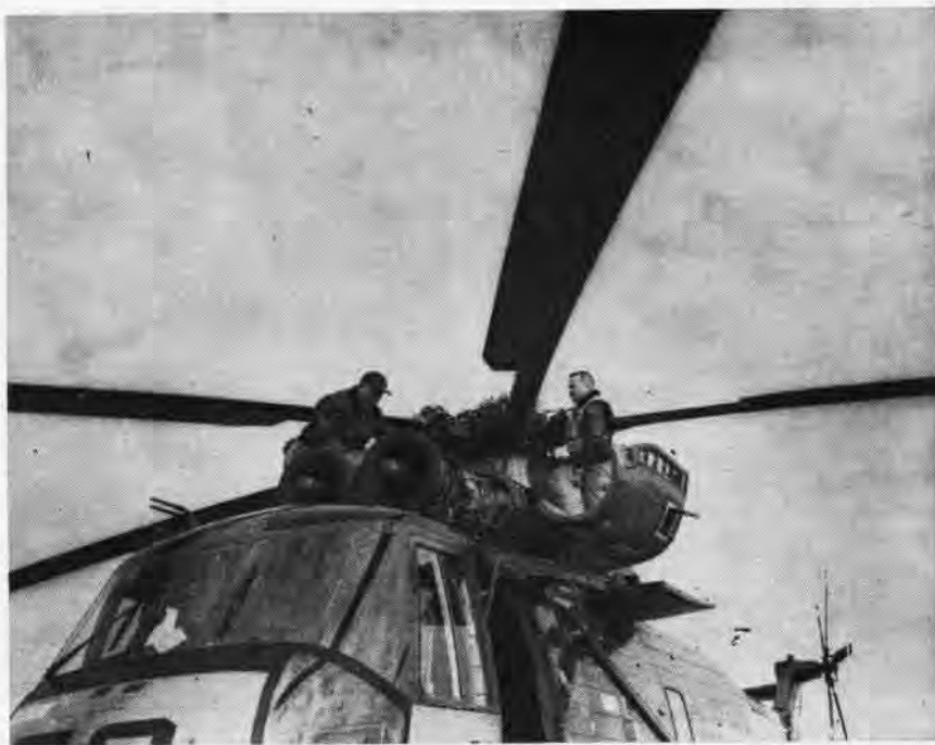
GEORGE TRAVERS , O&R mechanic who is H-3 plane captain, and Lt. E. C. Alexander , make the final check of transmission, rotor head, and engines before approving H-3 for test flight.
