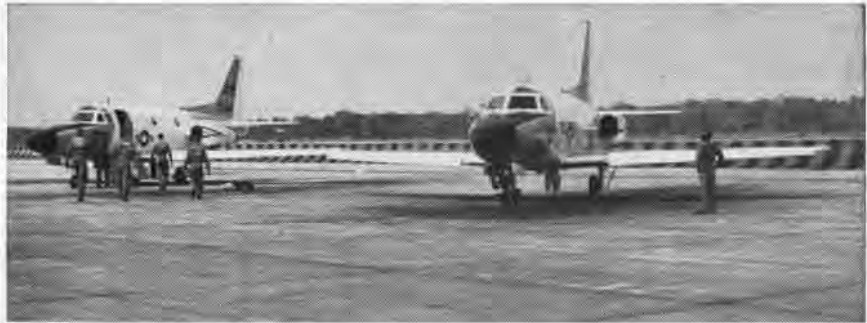
THE LOW WING , twin jet T-39D aircraft, configured for a crew of six, first went into operation at NAS Glynco on August 9, 1963, to train radar intercept students from NATTC. These T-39D's have just been pre-flighted and one will soon be on a training mission.
