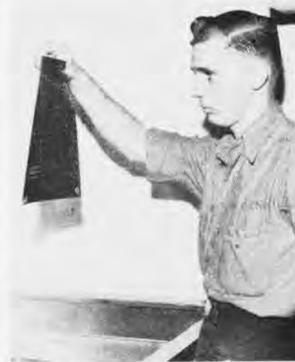
STUDYING a negative for photo offset, S. I. Jablonski, SN, looks for clarity and flaws.
