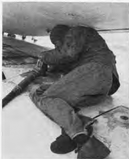
ESMON TUCKER, III, AA, crawls on the wing of an S-2A Tracker to fill the fuel tanks.
