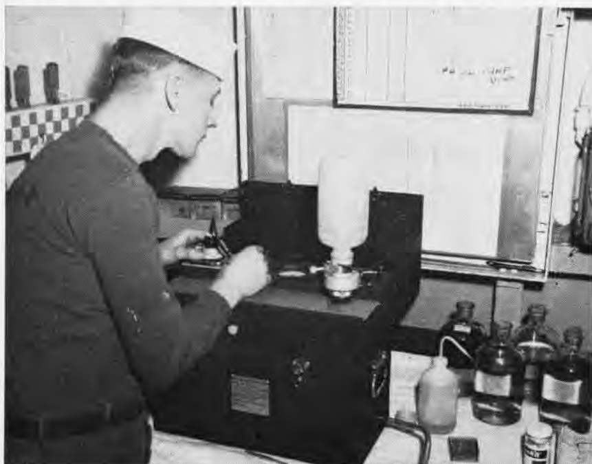
DAILY READING of a fuel sample aboard the Lake Champlain is made by Walter Dixon, ABF2. To ascertain its purity, he uses an Aeronautical Engine Laboratory contaminated fuel detector.
