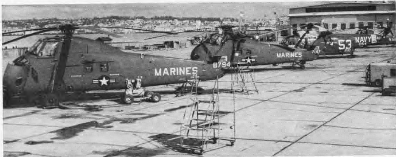
ON THE O&R CHECK LINE, big Sikorsky H-34 Sea Horses and H-3 Sea Kings are being made ready for flight test. Helicopters land on this same ramp when due for rework. Methods of quality control are carefully followed throughout the total program of repair and rework.
