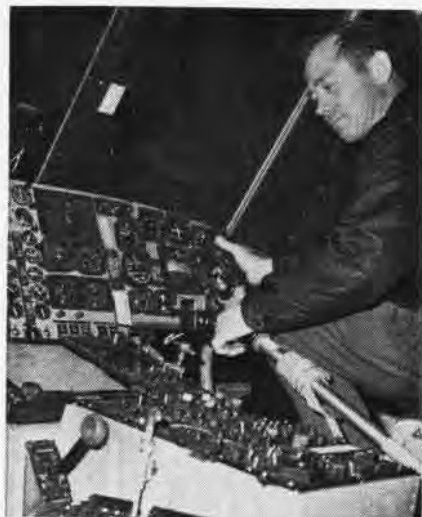
C. F. GEFTERS , O&R inspector, is checking the instrument installation in the Sikorsky H-3.
