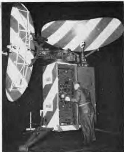
IN BLIMP HANGAR, a student in GCA maintenance course trouble-shoots a radar unit.
