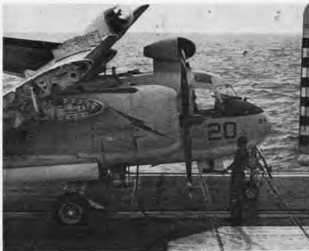
THE INHERENT danger of fire when avgas is pumped is met by Asbley L. Rowe, AN, who stands by the aircraft with a CO2 bottle ready.
