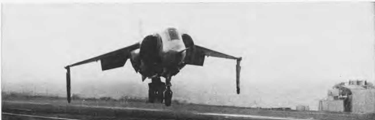
THE HAWKER-SIDDELEY P-1127 approaches for a VTOL touchdown on the British carrier, HMS Ark Royal . Test pilots commented that in ap-
