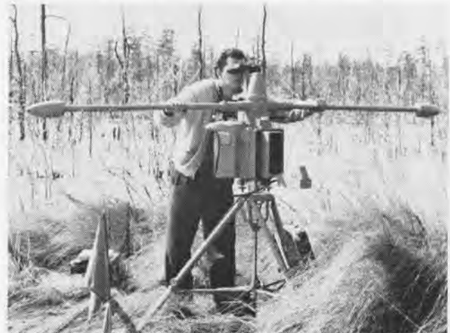
CAMERAMAN PHOTOGRAPHS aircraft glide pattern with Fairchild Flight Analyzer. Camera records 58 consecutive images on one glass plate.
