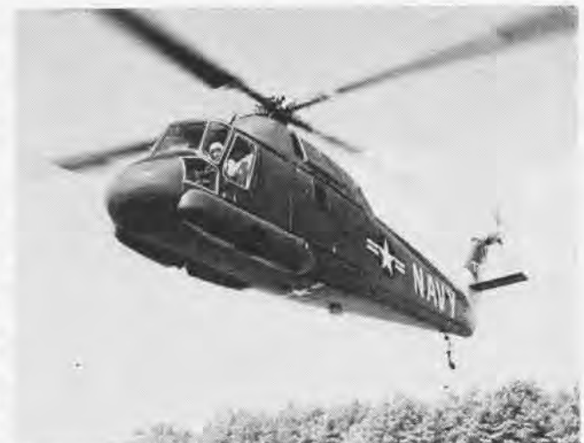
THE UH-2A Seasprite , Kaman's turbine-powered utility helicopter with all-weather capabilities, was put into service aboard ship in June.
