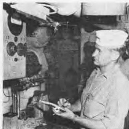
TAKING a reading from a salinity cell is one of the jobs done by R. D. Anrheim, FN.
