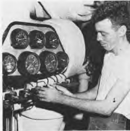
VACUUM gauge at Number Two evap, opened by S. F. Meyers, FN, records boiling point.
