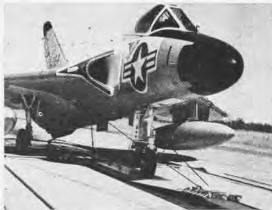
A SKYRAY AIRCRAFT on pre-tensioned catapult is an example of aircraft now being used for research purposes.
