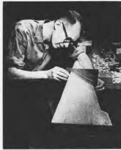
DTMB ENGINEER Richard Hartley checks prop blade section with template during carving.
