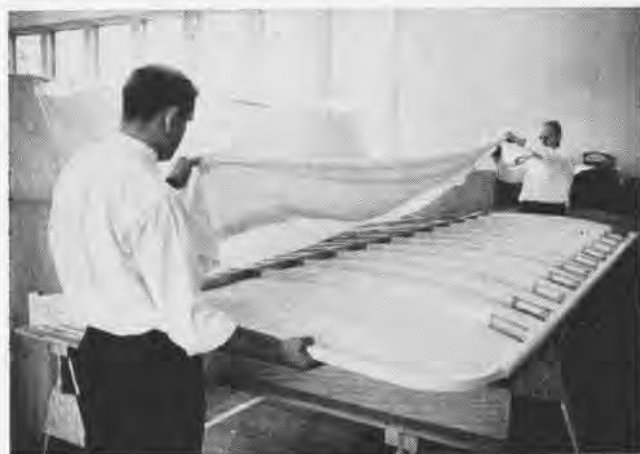
WING RIBS are in their pockets in lower surface muslin fabric; the upper surface will be stretched across and then tacked to front spar.
