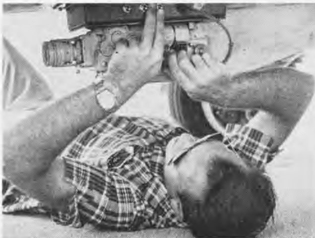
SCIENTIFIC PHOTOGRAPHER mounts 16mm Fastair on aircraft to record action of tailhook during engagement. The pilot actuates the camera.
