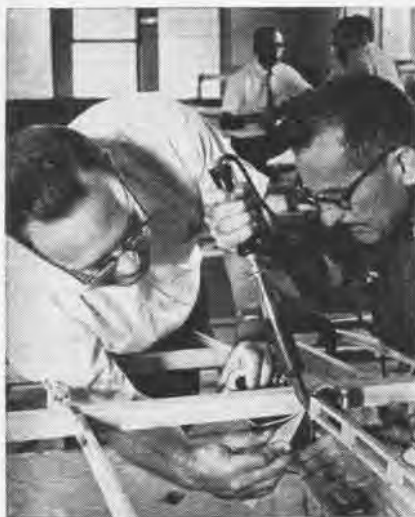
NATC ENGINEERS Harry Down and Nathan Frank carefully solder one of wing rib fittings.
