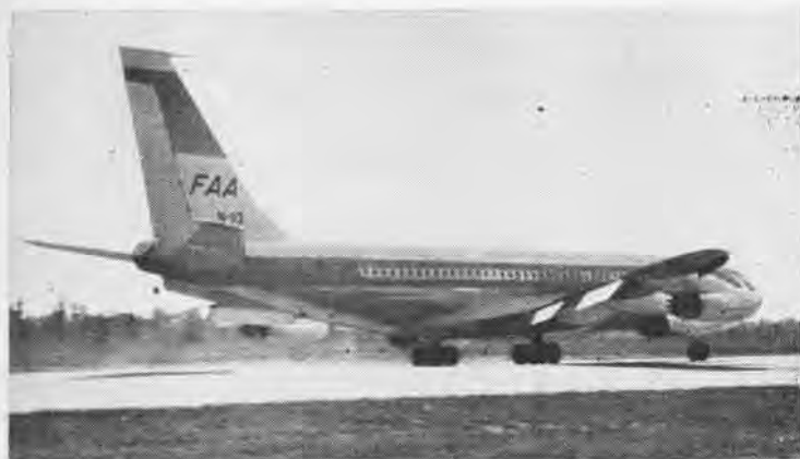
A BOEING 720 from the Federal Aviation Agency engages the E-14-1 arresting gear during test operation conducted at the Naval Air Test Facility.
