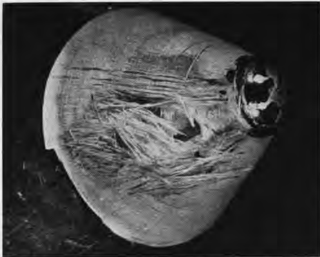
ONCE THIS TYPE of radome damage would have been regarded as irreparable, but now O&R North Island has come up with a sound method.
