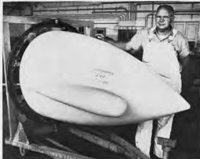
THE REPAIRED RADOME which Quality Assurance personnel have approved as ready-for-issue, and C. E. Reynolds, architect of the method.
