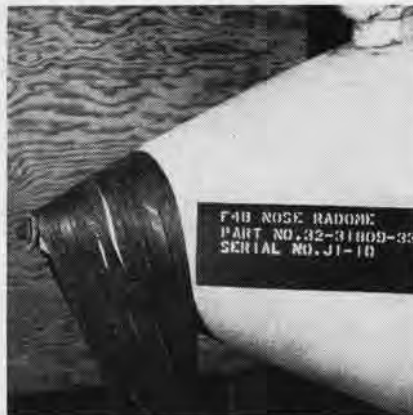
THIS SHOWS the way in which pressure is applied by the use of one-inch rubber bands.
