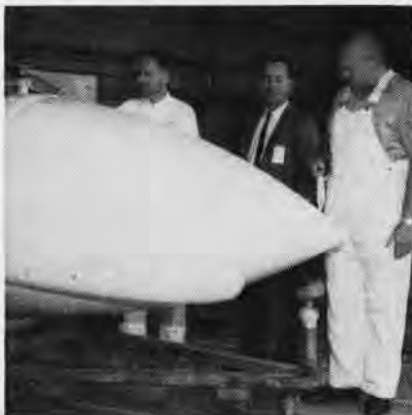
REYNOLDS APPLIES final touch of neoprene as G. S. Roberts and Bill Adkins look on.
