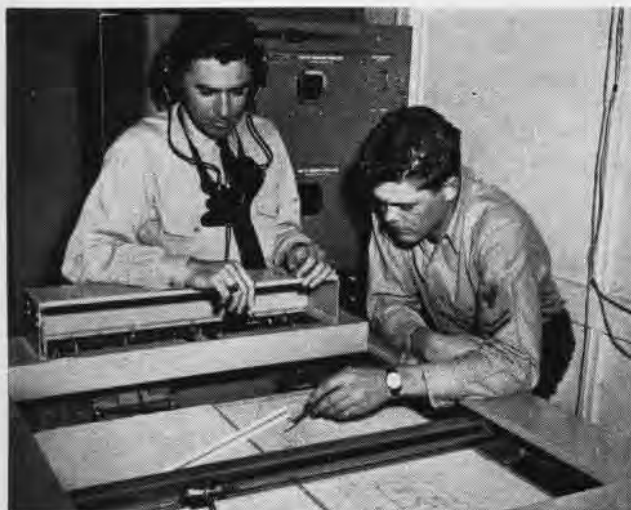
LTJG. W. R. KNIGHT, equipped with headphones, checks D. H. Aldrich, FTM2, on the three-dimensional plotter tracking the missile's flight.
