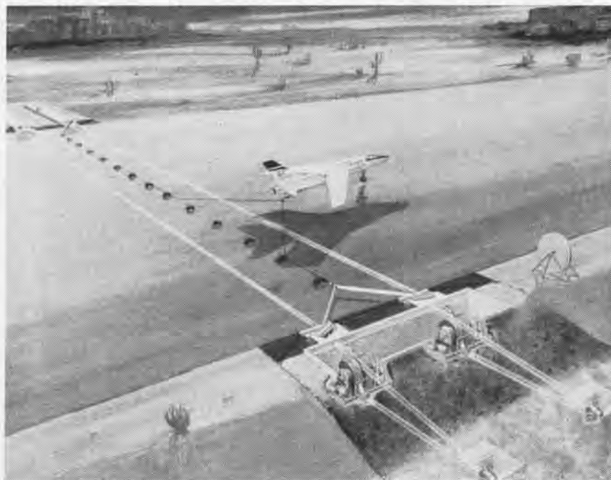
THIS ARTIST'S CONCEPT shows the E-15 arresting gear in action. Rotary friction engines are installed below ground level. The re-battery time for the equipment is about five minutes.
