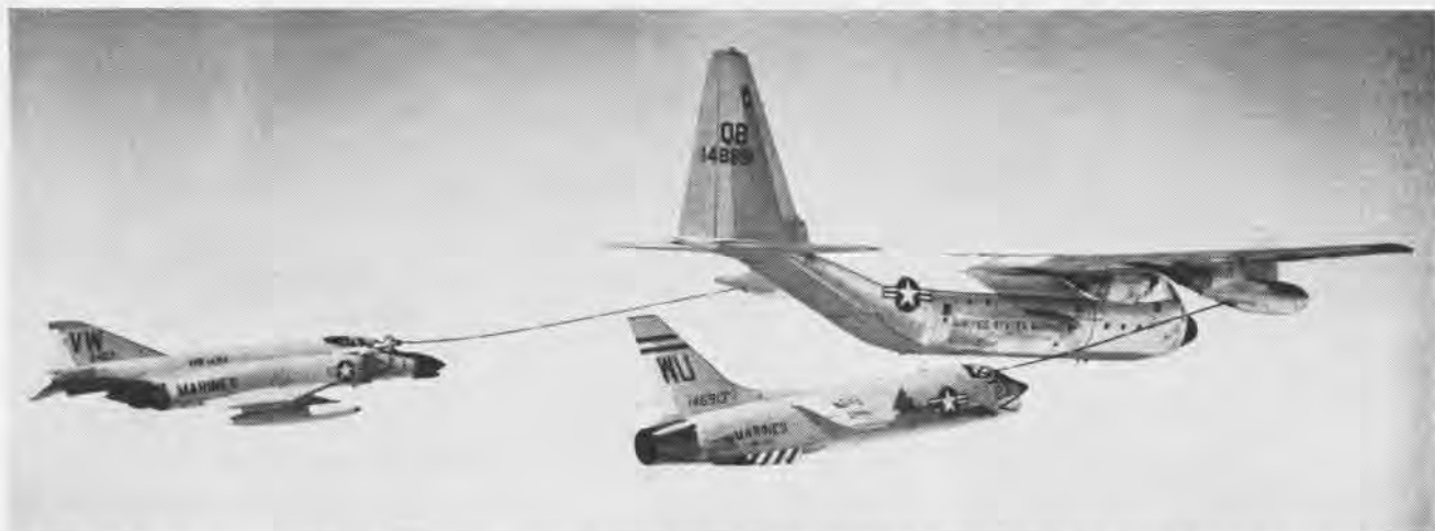
AERIAL REFUELING IS A VMGR-352 SPECIALTY. THIS KC-130F REFUELS TWO FIGHTERS BELONGING TO THE THIRD MARINE AIRCRAFT WING
