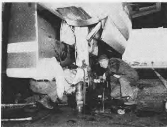
TO KEEP its eight Traders ready requires constant maintenance. Here squadron mechanics repair the brake on one of VR-21's C-1A's.
