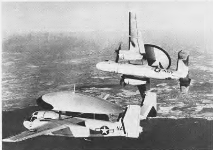
NAVY'S VAW-11, Capt. Martin "Butch" O'Neill commanding, took delivery of the first Pacific Fleet E-2A Hawkeye at North Island in January. The aircraft, flown from Grumman's Long Island plant, will be used to train flight crews and maintenance personnel. The E-2A (rear), a replacement for E-1B Tracer (foreground), is a carrier-based Early Warning Attack and Intercept Control System which provides an umbrella of protection against attacking aircraft.
