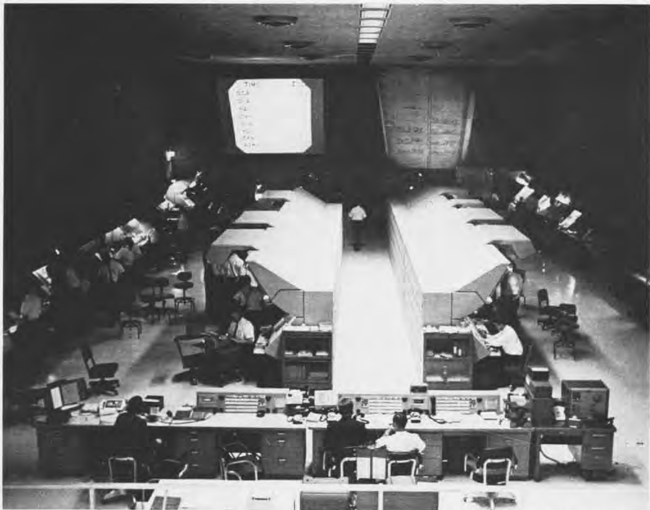
MAIN CONTROL room is manned 24 hours a day. Hooded rows house latest in radar scopes and electronic equipment. Weather information is projected on wall for easy view of controllers. The "Cbute" section is on left while APC area is next to right wall.
