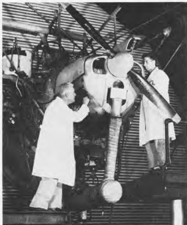
HOURS OF WORK are involved in instrumenting and inspecting engines and propellers. These technicians are moved to task by hydraulic lifts.
