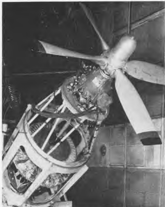
AN R-1820-84 engine is mounted at helicopter flight operating angle. An R-3350 nose gear serves to adapt a propeller for power absorption.
