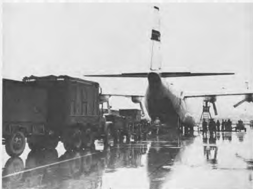
HERCULES AIRCRAFT can carry 16 tons of cargo, 64 combat troops, or 74 litter patients. Rear-loading at truck-bed height, ability to land and take off from short runways aid MATS airlift mission.
