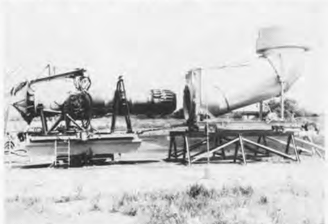
AEL UTILIZES an obsolete 40mm gun mount as a turntable for this outdoor test. Here noise suppressor is being tested with the J-75 engine.
