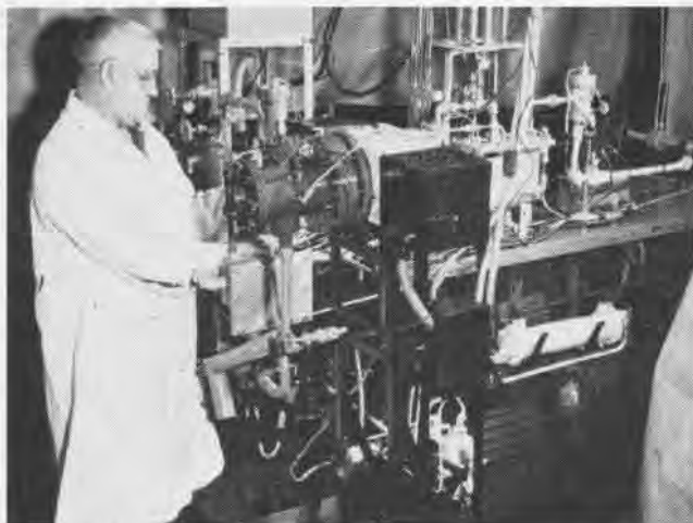
THIS INTRICATE jet engine oil system simulator provides, at reduced expense, the same results to be obtained in full-scale engine tests.
