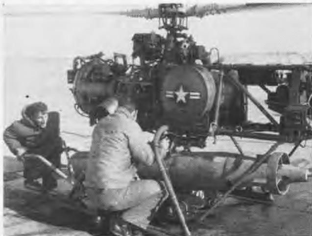
K. D. LARSEN, ADJ2 (left) , and H. R. Asquith, ADJ3 , load dummy torpedo on drone. It can carry a number of ASW weapons.
