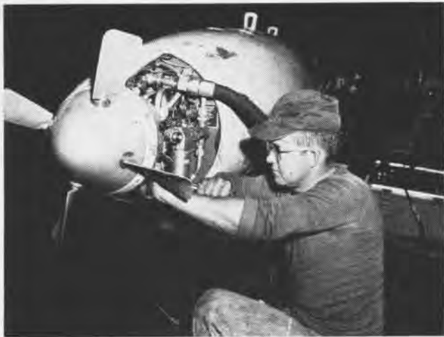
E ach pilot is dependent on outstanding maintenance if the year is to be accident free. Lamberson, AMSI, is working on a buddy store.
