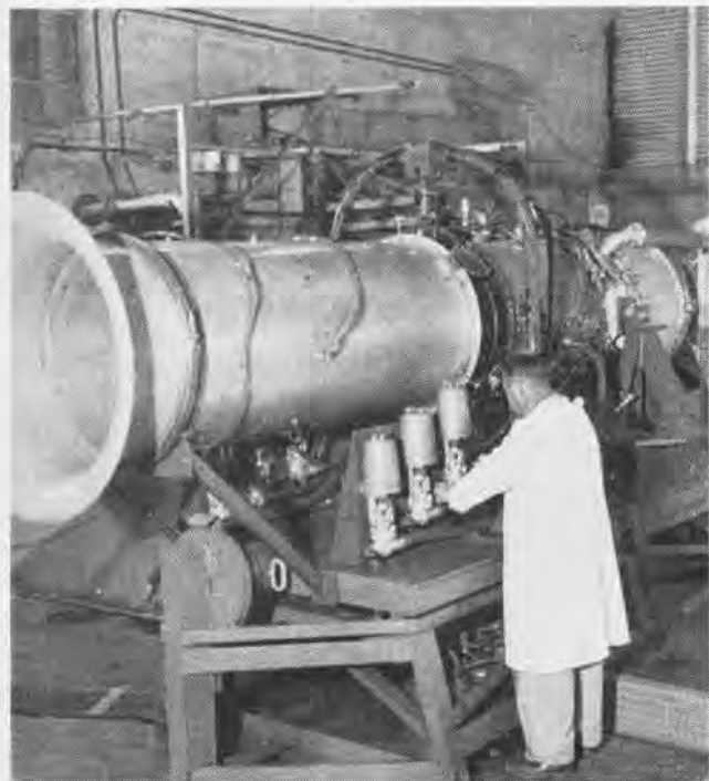
TECHNICIANS ARE involved in checking a test cell which will evaluate JP-5 fuel plus an additive for the J-65-W-4B engine bearings.
