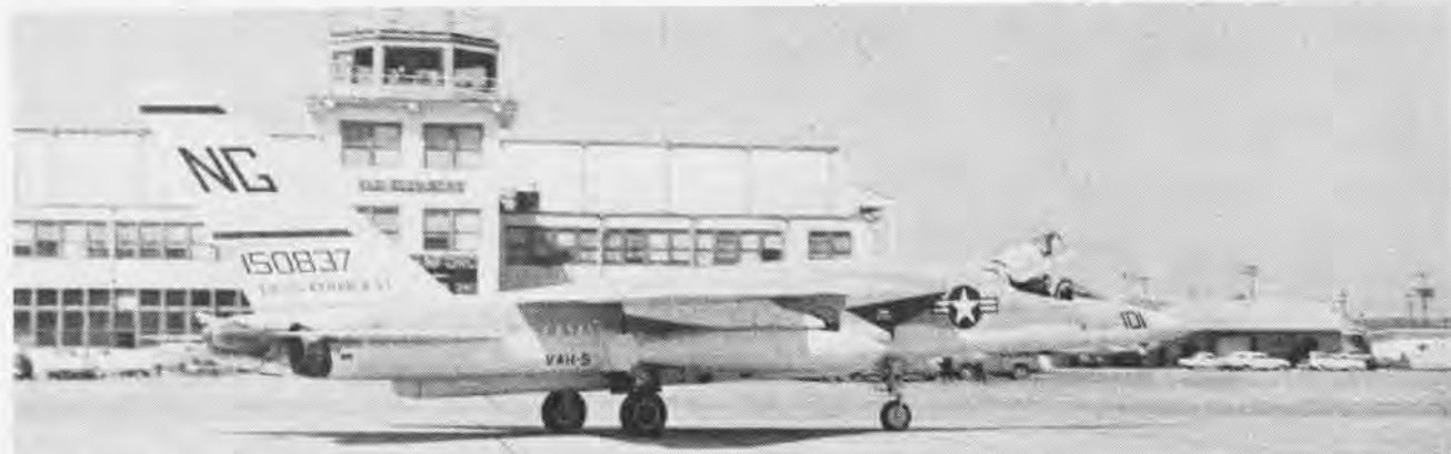
DUAL MISSION RA-5C Vigilantes were newcomers in the Tenth HAT-Wing One Bombing Derby. Flown by VAH-5, the first Fleet unit to operate them, RA-5C's added long-range reconnaissance to Vigilante's previous bomber capability. VAH-5 will deploy in the Pacific shortly.
