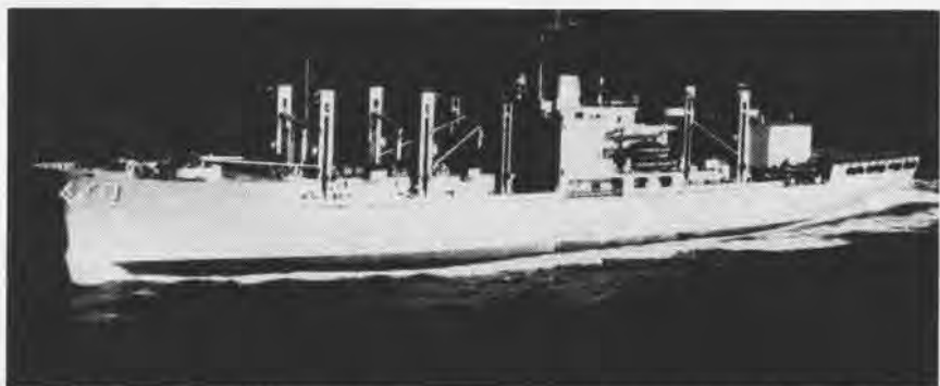
COMBAT STORES SHIP MARS (AFS-1), the first of a new class, was built by National Steel and Shipbuilding Co., San Diego. The ship performs cargo replenishments which previously required three ships—Store Ships (AF), General Stores Issue Ships (AKS) and Aviation Supply Ships (AVS). The Navy's first auxiliary class vessel with complete helicopter facilities, it carries two copters. Crew consists of 403 officers and men, Capt. R. C. Medley, commanding.
