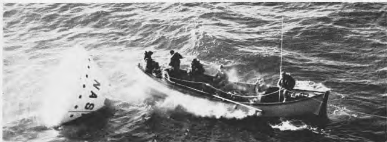
ONE METHOD of retrieval was practiced as follows: After the carrier had maneuvered within yards of the floating capsule, a motor whaleboat was dispatched. Recovery personnel attached a 2½-inch nylon line, and the capsule was then pulled alongside the after portion of the ship.
