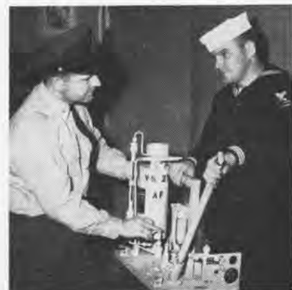
CHIEF W. H. HOLCOMB, AMHC, and R. E. Goss, AMH1, of VS-25, discuss the portable hydraulic test bench they built from discarded and salvaged parts of aircraft. The unit expedites the work of squadron maintenance men.
