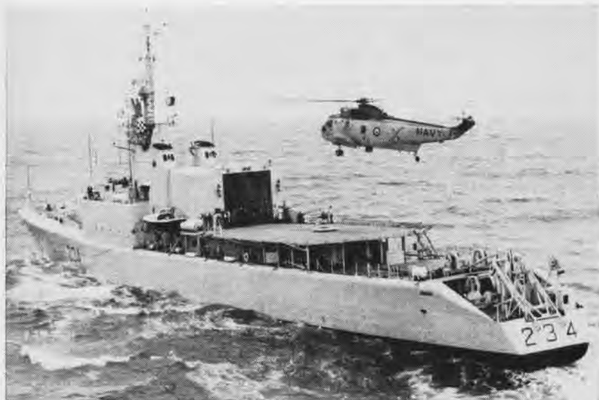
ROYAL CANADIAN NAVY HELICOPTER APPROACHES A DESTROYER ESCORT TO LAND CABLE IS ATTACHED TO SECURING DEVICE
