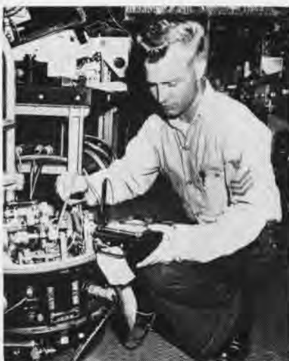
IN THE KEARSARGE, Gallagher, AT1, checks modulator voltage of APS-38 radar transmitter.
