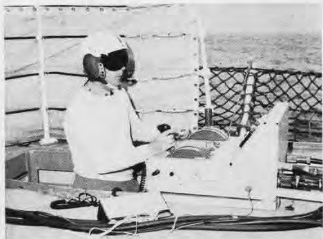
LSO AT ONE SIDE OF FLIGHT DECK CONTROLS TENSION AND SPEED
