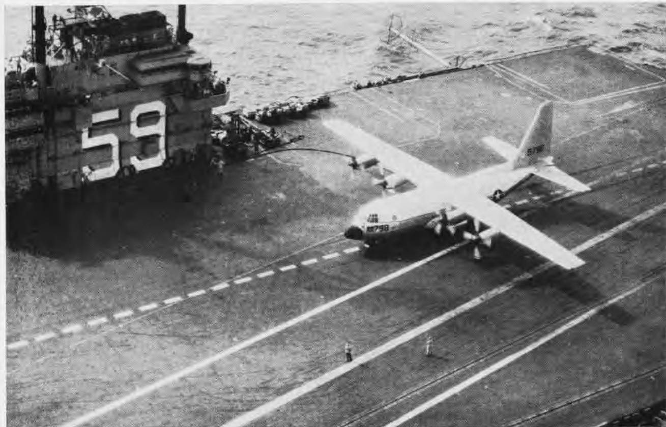
TO AID THE PILOT IN GUIDING THE BIG HERCULES, A WHITE CENTER LINE WAS PAINTED ALONG AXIAL DECK FROM BOW TO RAMP
