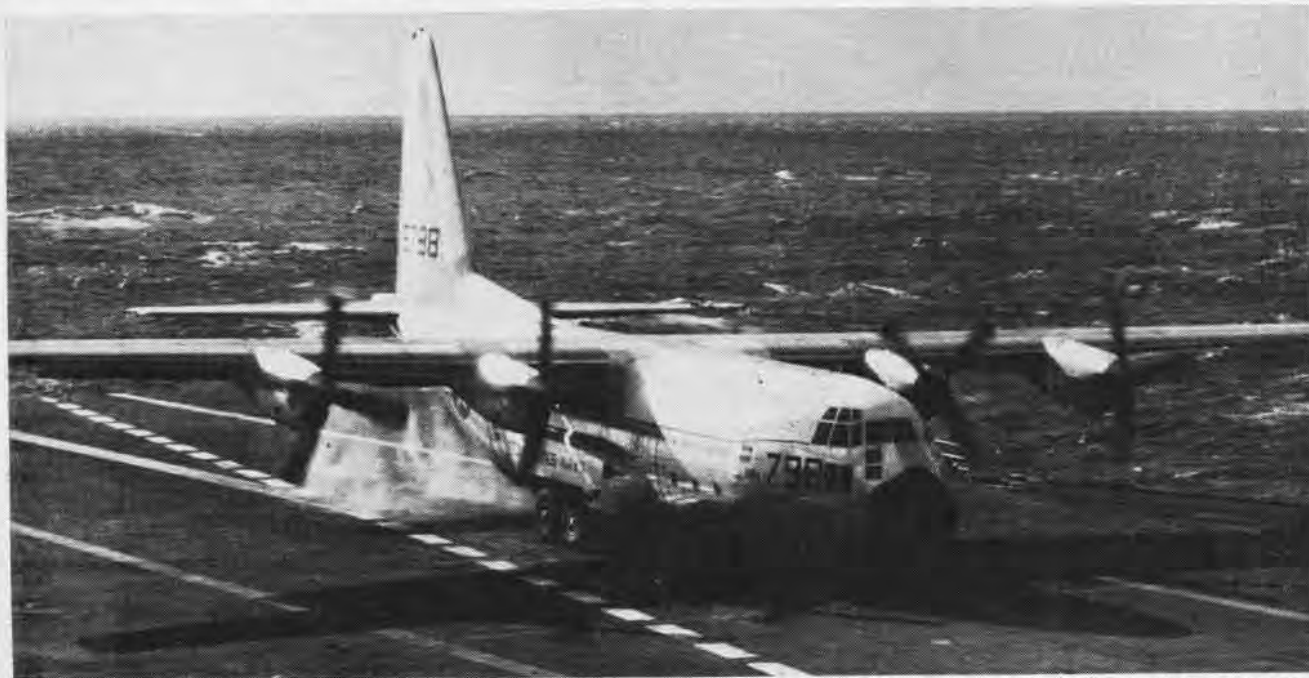
DURING FIRST TRIAL LANDINGS, SHIP SPEED WAS INCREASED 10 KNOTS TO REDUCE YAW MOTION AND STABILIZE WIND DIRECTION
