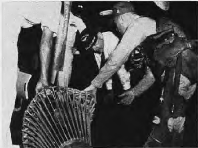
FULLY-GARBED pilot from Bonnie Dick air group shows Nitzte "basket" and explains procedures used in in-flight refueling of aircraft.
