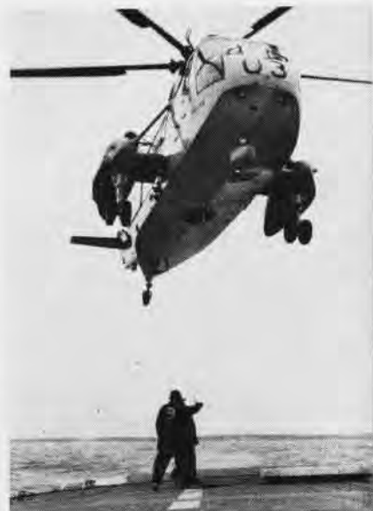
ROYAL CANADIAN NAVY HELICOPTER APPROACHES A DESTROYER ESCORT TO LAND CABLE IS ATTACHED TO SECURING DEVICE
