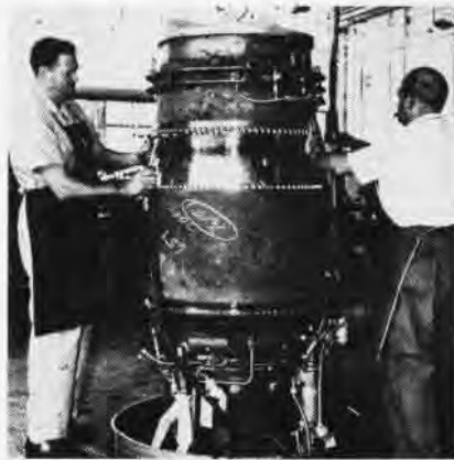
JET TURBINE IS PUT ON HYDRAULIC LIFT
