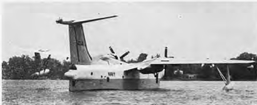
A NAVY SP-5B Martin Marlin patrol bomber returns to its birthplace, Martin Company at Middle River, Maryland, for modification. Under a Bureau of Naval Weapons contract, Martin will install a 3000-pound-thrust Pratt & Whitney J-60 jet engine in the tail of the seaplane and flight-test it to evaluate the improved performance expected during takeoff and in flight. Use of the new engine is expected to cut 20 seconds and 2400 feet off the takeoff time and distance. The engine will be located in what is now the tail observer's position. A radar unit now installed in the tail is scheduled to be relocated in the bow of the big Marlin.
