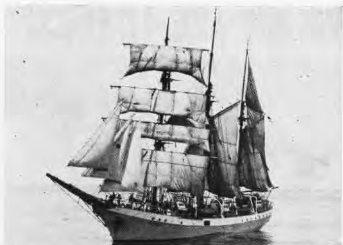
INDONESIA'S 191-foot entry, the Dewarntji, of iron construction, was built at Hamburg in 1953. She has a 600-hp auxiliary diesel engine.
