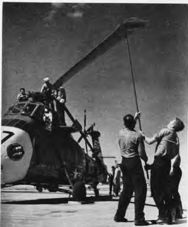
IN AIR/SEA RESCUE , time is of the essence. Plane handlers regularly practice unfolding rotor blades; locking devices are regularly checked.
